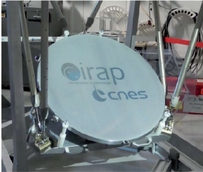
Figure 2.2: A picture of the PILOT primary mirror M1 attached to its interface plate in the PILOT instrument structure. The mirror is made of Aluminum.
