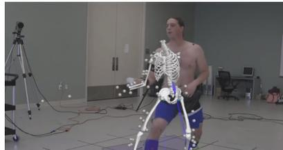
(e) Motion capture of a fencer. The reconstructed skeleton overlays one of the videos used for the recording. Markers are represented by the white dots; the markers on the fencer are not clearly visible. Source: University of Delaware
