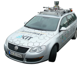
(b) The recording car uses to create KITTI dataset [42]. The Lidar can be seen on top of the car.
