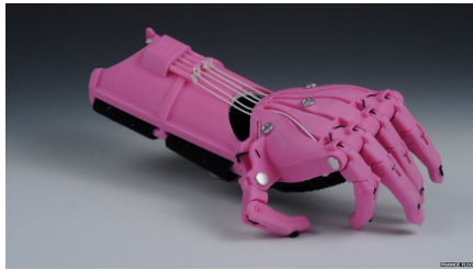
(a) Prosthetic hand. CAD software was used to design the hand and 3D printer to manufacture it. Source: [85]
