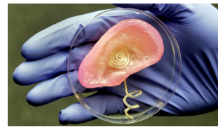
(e) 3D printed bionic ear. The electronic part would be able to enhance functionalities over human [81].
