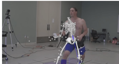
(e) Motion capture of a fencer. The reconstructed skeleton overlays one of the videos used for the recording. Markers are represented by the white dots; the markers on the fencer are not clearly visible. Source: University of Delaware
