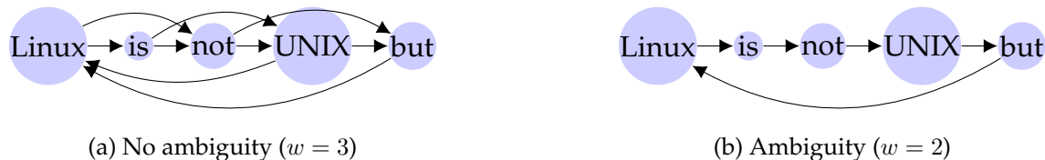
Figure 3.1 – Sequence graphs (or graphs-of-words ) built for the sentence “Linux is not UNIX but Linux” using window sizes 3 (a) and 2 respectively (b). In the second case, the sequence graph is ambiguous, since any circular permutation of the words admits the same representation.
