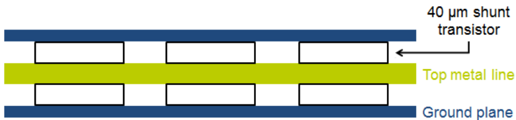
Figure 105: Top view of the shunt positioning in relation to the transmission line
