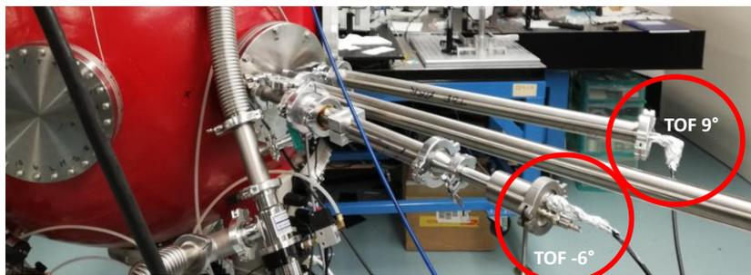
**Figure 3.42** Second ALLS configuration: TOF lines at -6° and 9°. One can observe the small size of the diamond detectors. The line in the middle is for the TP (@ 0°).
