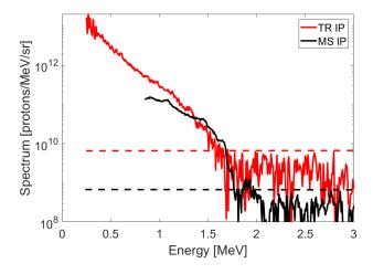
**Figure 4.11** Proton energy spectra recorded at 30° in two similar shots using both types of IPs. The one in red is from a BAS-TR IP while the black one is from BAS-MS IP. Dashed lines indicate the detection limit corresponding to the mean value of the background level plus two times its variance.
