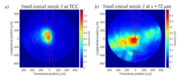
**Figure 4.6** Capture of the  $2\omega$  emission of the plasma during 120 ps after the laser-gas interaction on a conical nozzle. *a*) The nozzle is placed at TCC *b*) The rising slope of the jet density profile is placed at TCC.
