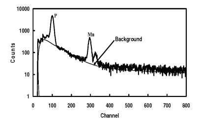
**Figure 5.8** X-ray spectrum of Manganese and Potassium for energy calibration. The figure is taken from [Kabir 2013].
