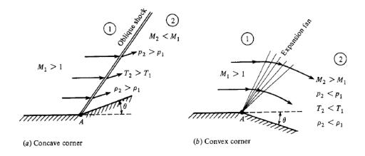
Figure 3.8. Diagrams of supersonic flow over a corner. From [Anderson 1990].
