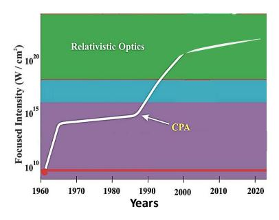
Figure 1.1. Laser intensity evolution from 1960 to 2012. Adapted from [Mourou and Tajima 2012].
