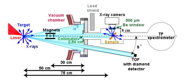
**Figure 5.9** Experimental setup. The interaction of the ALLS 100 TW laser with the solid target (represented in blue, on the left) accelerates several types of ions species (e.g. protons H<sup>+</sup>) and generates X-rays. The ions and X-rays propagate under vacuum to the sample (represented in orange, on the right) to be probed and to the ion detectors (the *Thomson parabola* (TP) and the *time of flight* (TOF)). The X-rays generated by the sample are analyzed by the X-ray camera.
