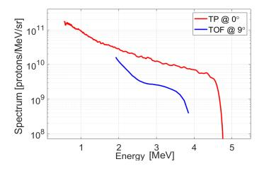
Figure 5.15 TOF (9 $^{\circ}$  in blue) and TP (0 $^{\circ}$  in red) proton spectra as obtained for a Cu typical shot.
