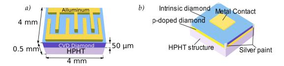
**Figure 3.40** Two different types of electrodes layout: *a*) the interdigital configuration, *b*) sandwich configuration. They are both mounted inside a cylindric metallic enclosure designed to minimize the EMP effects. [Verona 2015]
