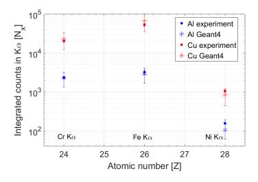
**Figure 5.19** Measured integrated number of counts in the respective Fe, Ni and Zn  $K_{\alpha}$  peaks (presented in dots) obtained from the spectra depicted in B and C. Geant4 simulation results are presented with asterisks.
