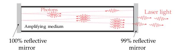
Figure 2.2. Scheme of multi-pass photon process in a laser cavity.
