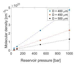
**Figure 3.15** Evolution of the molecular density as a function of the *reservoir* pressure at a distance of 500  $\mu$ m from the *conical nozzle* exit for different exit sizes (400  $\mu$ m, 450  $\mu$ m and 500  $\mu$ m).
