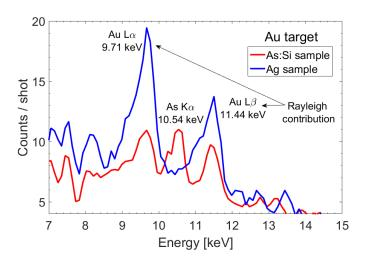
**Figure 5.22** X-ray spectra obtained when irradiating Arsenic doped Si wafer sample (red) using the laser-based sources produced with an Au laser-interaction target. and compared with an Ag sample (blue).
