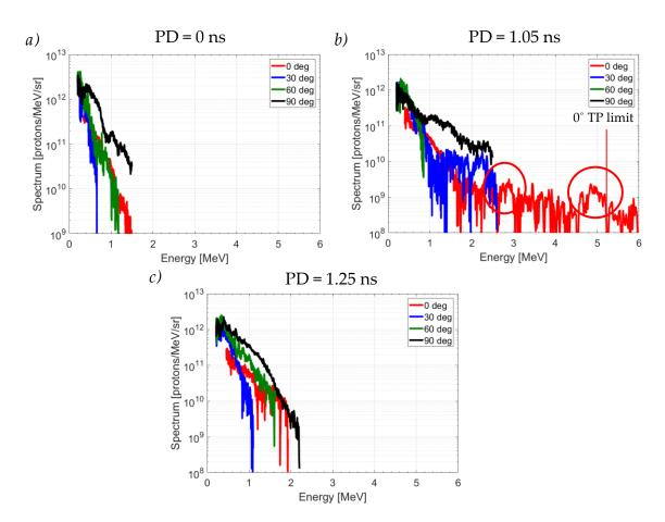
**Figure 4.8** Proton energy spectra at  $0^{\circ}$  (red),  $30^{\circ}$  (blue),  $60^{\circ}$  (green) and  $90^{\circ}$  (black) obtained with the laser focused at the rising slope of the *big conical nozzle* density profile at  $z = 200 \, \mu m$ . The ASE is continuously reduced from one shot to the other.
