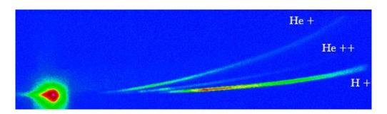
**Figure 3.44** Scanned BAS-TR IP that shows the three different parabolas from the helium-hydrogen gas mixture used as a target. The spot at the left indicates the initial position of the particles before being deflected by the electric and magnetic fields. The X-rays and UV light from the laser reach the IP at this spot.
