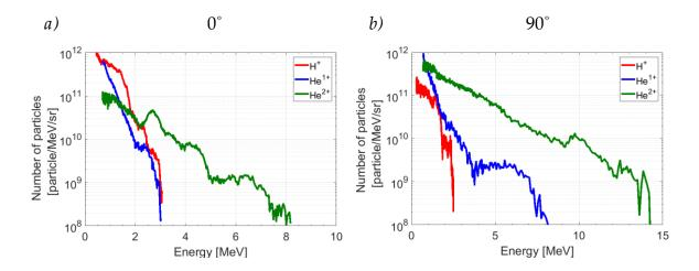
**Figure 4.28** Particle energy spectra of protons (red),  $He^{1+}$  ions (blue) and  $He^{2+}$  ions (green) obtained with a mixture of helium and hydrogen gas-jet target on the same shot at a)  $0^{\circ}$  b)  $90^{\circ}$ .
