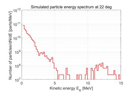
Figure 4.26 Forward proton energy distribution at t = 3.6 ps from PIC simulations from 21° to 23°.
