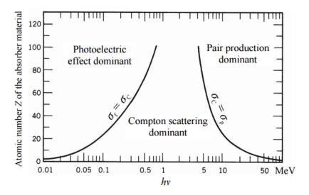
**Figure 5.2** Diagram of the different effects between photons and matter depending on the atomic number of the matter and the energy hv of the incident photon.
