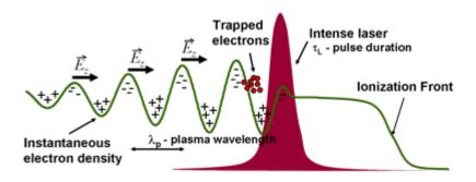
**Figure 2.10** Schematic of a laser pulse interacting with a low-density gas (e.g. hydrogen or helium). This image is taken from [Michigan engineering website].
