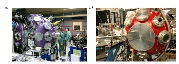
**Figure 3.1** *a)* Picture of the MILKA chamber at LULI Research Infrastructure in France. [Taken from *FuseNet Association*]. *b)* Picture of the *Boule rouge* at EMT-INRS center in Canada. On the left, one can observe the small vacuum chamber coupled to the main one, where a spectrometer is placed. The KF 40 tube visible between the principal door and the secondary chamber is part of another spectrometer.
