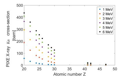
**Figure 5.6** PIXE X-ray  $K_{\alpha}$  cross-sections with different proton energies as function of the sample atomic number, Z. Values are taken from PIXE Data Library which is available from *the Radiation Safety Information Computational Center (RSICC) at Oak Ridge National Laboratory as DLC-246*.
