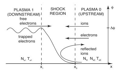
**Figure 2.15** Steady-state electrostatic shock structure as seen from the shock frame. Electrons from the upstream region are free while electrons from the downstream region are free or trapped. Ions are slowed down by the electrostatic potential and reflected back into the upstream for strong shocks. Figure extracted from [Fiuza 2013].
