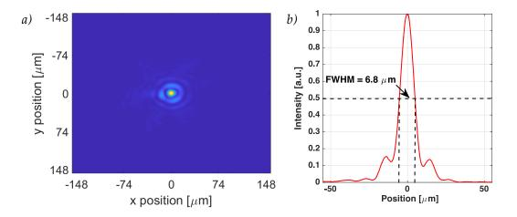
**Figure 3.4** Focal spot imaging system designed to work at full power (2 J at TCC). *a)* Picture taken from a CCD *b)* Reconstructed spot size. The intensity as a function of the position is plotted. Picture taken from [**Paper III**].
