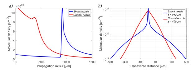
**Figure 3.25** *a)* Comparison of the downstream propagation of the flow from the nozzle exit for *shock nozzles* and *conical nozzles*. *b)* Comparison of both transversal density profiles in logarithmic scale at the optimal *z* where maximal density is reached.
