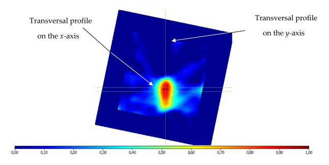
**Figure 3.33** Density reconstruction of **Figure 3.32b.** The image is normalized. The color bar is proportional to the density by a factor of  $10^{21}$  cm<sup>-3</sup>. The lines are at  $x = 360 \mu m$  and y = 400 and  $420 \mu m$ .
