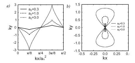
**Figure 2.6** Trajectories of a free-electron in a linearly polarized electromagnetic plane wave propagating in the *x*-direction in *a*) the laboratory frame, and *b*) the averaged rest frame. For a 1  $\mu$ m laser wavelength, the chosen values of  $a_0$  correspond roughly to  $I_L = 10^{17}$ ,  $10^{18}$  and  $10^{19}$  W/cm<sup>2</sup> respectively. Taken from [Gibbon 2005].
