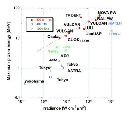
**Figure 2.13** Survey of TNSA cut-off energies measured in experiments before 2014, plotted vs irradiance and labeled according to the pulse duration. This picture was taken from [Borghesi 2014].
