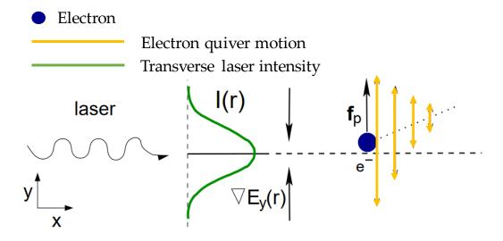
**Figure 2.7** Illustration of the *ponderomotive force* experienced by a non-relativistic electron initially sitting near the center of the beam in a spatially varying laser intensity profile. The electromagnetic wave propagates in the x direction. The laser electric field is assumed to vary in the y-direction and in time. Taken from [Gibbon 2005].
