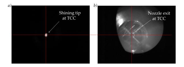
**Figure 4.2** First experiment bottom view. The red cross represents TCC. *a)* The illuminated tip at TCC. *b)* The nozzle at the same place.
