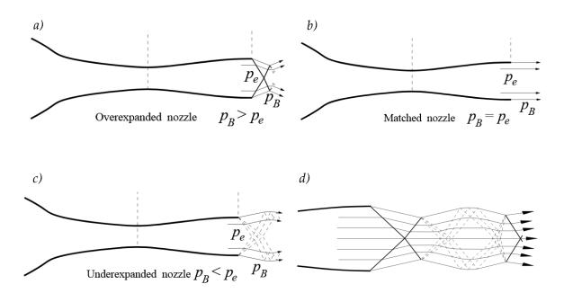
**Figure 3.10** Scheme representation of the flow of *a*) an *over-expanded* nozzle, *b*) a *matched* nozzle, *c*) an *under-expanded* nozzle and *d*) a *jet shock diamond*. In this last picture, only the nozzle exit is presented on the left. Taken from [Anderson 1990].
