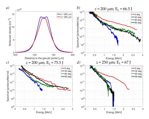
**Figure 4.9** Proton energy spectra at  $0^{\circ}$  (red),  $30^{\circ}$  (blue),  $60^{\circ}$  (green) and  $90^{\circ}$  (black) obtained with the laser focused at the rising slope of the *small conical nozzle 1* jet density profile at c) and d) 200  $\mu$ m b) 250  $\mu$ m. A comparison between the density profiles at  $z = 200 \ \mu$ m and  $z = 250 \ \mu$ m is shown in a).
