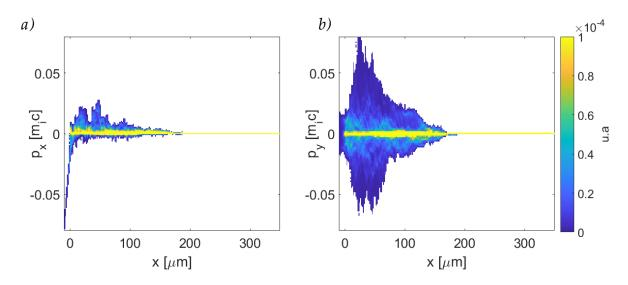
**Figure 4.19** Proton phase space histogram at time t = 1 ps: a) longitudinal and b) transverse momentum as a function of the longitudinal coordinate.
