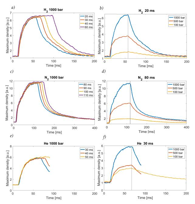
**Figure 3.35** Gas flow evolution of a) b) diatomic hydrogen c) d) diatomic nitrogen e) f) helium as a function of time for a) c) e) different solenoid valve opening durations b) d) f) different pressures. When the solenoid valve is triggered (at t = 0 ms) is about 12 ms before the gas flow.
