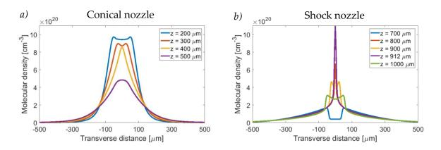
**Figure 3.24** Transversal density profiles at 1000 bar for different distances from the nozzle exit *z a) conical nozzles b) shock nozzles*. A comparison of both can be found in **Figure 3.25b** in logarithmic scale.
