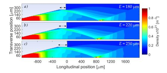
**Figure 3.21** Molecular density maps at 1000 bar for different edge size E. The longitudinal position is normalized to z=0 at the exit of the nozzles. a)  $E=180 \ \mu m$ , b)  $E=220 \ \mu m$  and c)  $E=250 \ \mu m$ . The red color at the entrance of the nozzle can represent densities larger than  $1\times 10^{21} {\rm cm}^{-3}$ .
