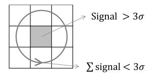
**Figure 5.11** Scheme of the SPE condition in our algorithm. We repeat this process for all the image pixels. The borders are not considered in the algorithm.  $\sigma$  is the standard deviation of the histogram from the acquisition when the laser is off. Only electronic noise is then measured.
