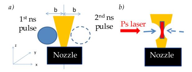
**Figure 6.3** *a)* Principle of the plasma laser-machining using one or two ns laser beams to shape the plasma profile before the arrival of the main ps laser pulse. *b)* The ps laser pulse arrives when the density profile is already modified.
