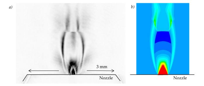
**Figure 3.27** Propagation in air at 1 bar pressure for Mach waves generated by the designed *conical nozzle* fed with 50 bar  $N_2 a$ ) measurement and b) simulation. Shock fronts are observed in both cases at the same distance of the nozzle exit.
