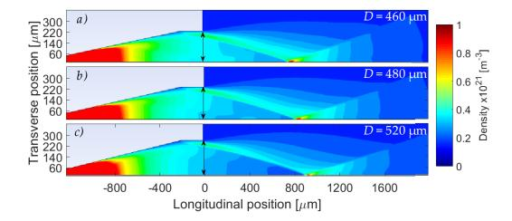
**Figure 3.20** Molecular density maps at 1000 bar for different exit diameters D. The longitudinal position is normalized to z = 0 at the exit of the nozzles. a) D = 460  $\mu$ m, b) D = 480  $\mu$ m and c) D = 520  $\mu$ m. The red color at the entrance of the nozzle can represent densities larger than 1  $\times$  10<sup>21</sup> cm<sup>-3</sup>.
