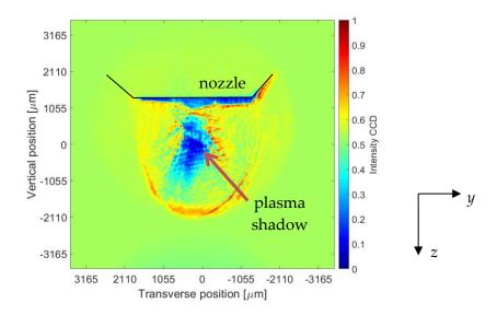
Figure 4.7 Shadowgraphy of the plasma by a Quanta-Ray laser (ns) during 500 ps after the laser-gas interaction.
