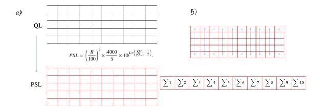
**Figure 3.45** Making the assumption that the parabola trace is just in 10x10 pixels (represented as squares) *a*) QL must be converted in PSL before any manipulation. *b*) Then one can sum the PSL for each column.
