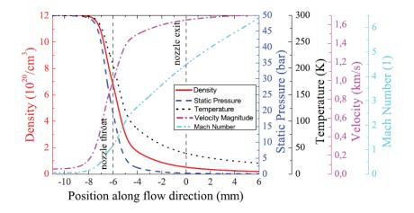
**Figure 3.12** Density, static pressure, temperature, velocity, and Mach number obtained at the center of a helium gas flow through a Laval nozzle obtained from *computational fluid dynamics* simulations from [Schmid 2012].
