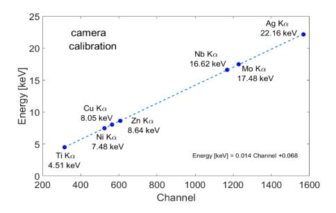
**Figure 5.12** Calibration of the camera with 7 different pure targets. The points are fitted with a linear curve: E (Channel) =  $\alpha_1$  \* Channel +  $\alpha_2$  where  $\alpha_1$ = 0.01413 with a confidence bound of (0.01403, 0.01423) and  $\alpha_2$ = 0.06826 with a confidence bound of (-0.02602, 0.1625).
