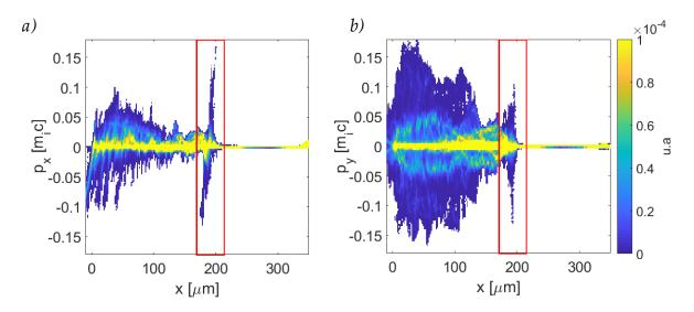
**Figure 4.21** Proton phase space histogram at time t = 1.8 ps: *a)* longitudinal and *b)* transverse momentum as a function of the longitudinal coordinate.
