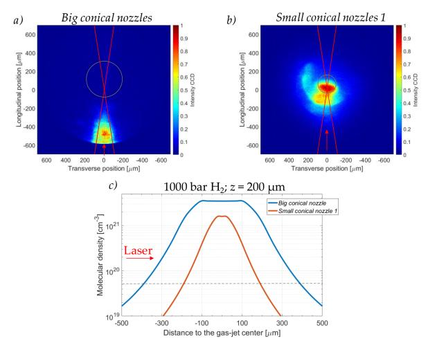
**Figure 4.3** Capture of the  $2\omega$  emission of the plasma during 250 ps after the laser-gas interaction on *a*) a *big conical nozzle b*) a *small conical nozzle 1* . *c*) The gas density profile for these different types of gas targets.
