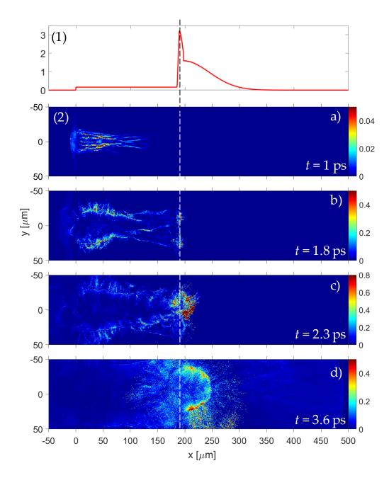
**Figure 4.18** (1) Proton density profile [in  $n_c$  units] at t = 0 ps (2) Evolution of the proton energy density [in relativistic units,  $n_c m_e c^2$ ] in the PIC simulation: a) t = 1 ps b) 1.8 ps c) 2.3 ps d) 3.6 ps
