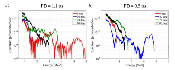
**Figure 4.15** Proton energy spectra at 0° (red), 30° (blue), 70° (green) and 80° (black) obtained with the laser focused at the rising slope of the jet density profile and the ASE level was reduced at the minimum achievable.
