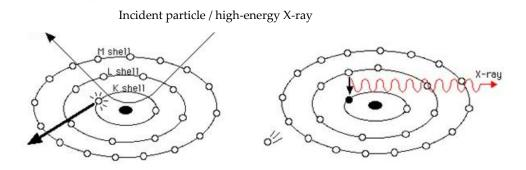
**Figure 5.3** Scheme of the inner-shells atoms when they are perturbated by an incident particle or a high-energy X-ray (for PIXE and XRF respectively). An electron is ejected and a vacancy is formed. Then an electron from an upper level drops down and the atom emits an X-ray.
