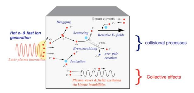
Figure 2.17. Different processes taken into account in the PICLS simulations. Extracted from [PICLS handbook].
