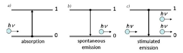
**Figure 2.1** Interaction mechanisms between an atom and a photon (the photon has an energy *hv* equal to the difference between the two atomic level energies) between levels 0 and 1. *a)* shows the absorption, *b)* the *spontaneous* emission and *c)* the *stimulated* emission. Figure taken from [Photonics 2016].
