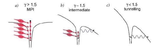
**Figure 2.5** Schematic picture of the Coulomb potential of an atom interacting with laser fields. *a) multiphoton* ionization when the Keldysh's parameter  $\gamma$  is bigger than 1.5 *b)* the intermediate case and *c)* when  $\gamma$  is smaller than 1.5 and *tunneling* of *barrier-suppression ionization* by a strong external electric field can take place.
