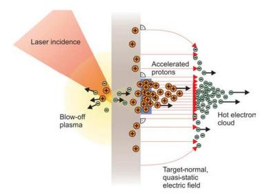
**Figure 2.12** Scheme of TNSA. The laser irradiates the front surface on a thin foil and the laser field ionizes and heats electrons. Hot electrons cross and scatter through the target and ionize the rear side. A hot electron cloud remains at the target rear surface interface that creates a confined electrostatic steep potential with a value in the order of some TV/m. This electric field accelerates ions from the impurities. This figure is taken from [Schwoerer 2006].
