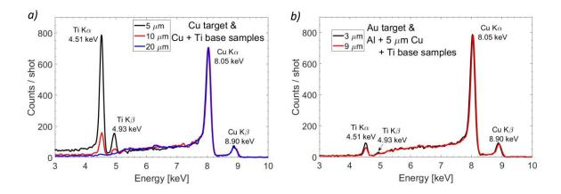
**Figure 5.25** X-ray spectra obtained when irradiating different stacks using the laser-based produced with *a*) Cu and *b*) Au laser-interaction target. In the *a*) case: 5, 10, and 20  $\mu$ m Cu layer on a Ti substrate. In the *b*) case: 3 and 9  $\mu$ m Al layer lying on a 5  $\mu$ m Cu layer on a Ti substrate.
