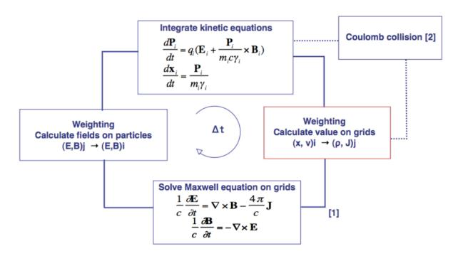
**Figure 2.16** Time loop in a PIC code. Time is increased in steps of  $\Delta t$  so that  $t = t_0 + n \times \Delta t$  where n is the number of loops of the simulation. Taken from [PICLS Handbook].
