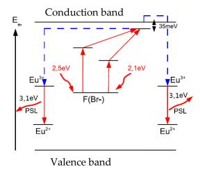
**Figure 3.38** Levels of BaFBr crystal doped with Europium in the SR IP sensitive layer. The figure is taken from [Bonnet 2013].
