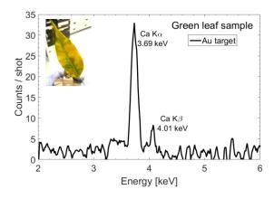
**Figure 5.23** X-ray spectra obtained when irradiating green leaf sample using the laser-based sources produced with an Au laser-interaction target.
