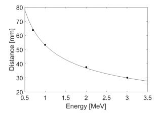
**Figure 3.46** Four different ion beam energies were analyzed in AIFIRA accelerator. 0.7 MeV, 1 MeV, 2 MeV and 3 MeV. A fit was done to relate the position of the beam spot to its energy. This process was performed for all the TPs used in the gas-jet experiment.
