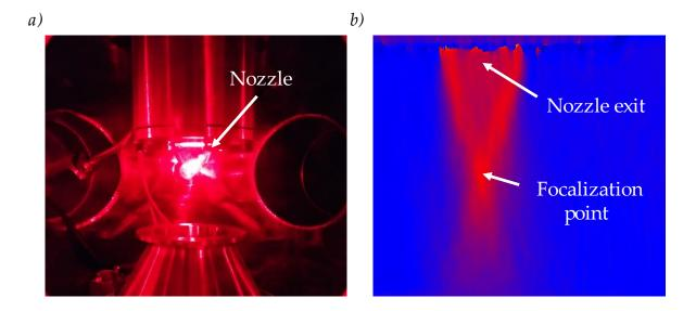
**Figure 6.2** *a)* Picture of the nozzle in the interferometer setup. The nozzle is illuminated by a red laser. *b)* Phase shift image by a glass made *shock nozzle*. The focal point is at z  $\sim$ 900  $\mu$ m.
