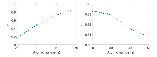
**Figure 5.5**. *a)* Fluorescence yield for the K-shell as a function of the atomic number *b)* probability of  $K_{\alpha}$  transitions a function of the atomic number. Values are taken from PIXE Data Library which is available from *the Radiation Safety Information Computational Center (RSICC) at Oak Ridge National Laboratory as DLC-246*.
