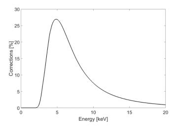
Figure 5.13 Correction curve as a function of the energy taking into account the SPE probability, the two 250  $\mu$ m thickness Be windows and the camera quantum efficiency.
