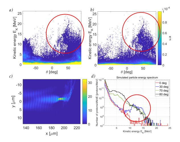
**Figure 4.23** Angular energy distribution of *a*) all forward accelerated protons and *b*) forward shock protons accelerated in the interval  $x = 185 \, \mu \text{m}$  to  $x = 250 \, \mu \text{m}$  at  $t = 2.3 \, \text{ps.}$  *c*) Period-averaged electromagnetic laser energy  $E_z^2 + E_y^2 + (c \, B_z)^2$  at 2.3 ps. *d*) Particle energy spectrum at the same simulation time.
