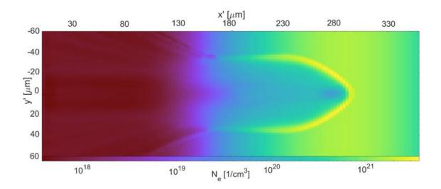
**Figure 4.17** 2D slice of the 3D electron density in the FLASH simulation at t = 240 ps, the time of the main pulse arrival.
