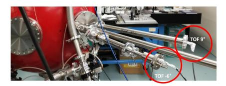
**Figure 3.42** Second ALLS configuration: TOF lines at -6° and 9°. One can observe the small size of the diamond detectors. The line in the middle is for the TP (@ 0°).
