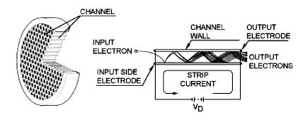
**Figure 3.39** Schematic of a *microchannel plate* (MCP) detector. At the left, a single channel electron multiplier. At the right, with electron multiplication dynamics [dm photonics].
