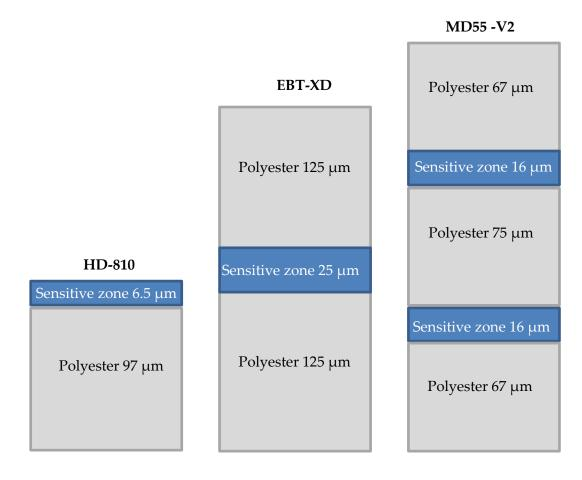
**Figure 3.37** Schematic view of the layers of three different RCF (HD 810, EBT-XD and MD55-V2). In a laser-plasma experiment, protons come from the top to the bottom.
