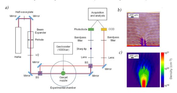
**Figure 3.28** *a)* Scheme of the Mach-Zehnder interferometer (red line). Strioscopy (blue line) is set up by blocking the reference ray in the interferometer and by including a sharp object in the focus of the imaging lens. The signal is detected by a photodiode. *b)* Interferogram obtained with  $N_2$  at 1000 bar reservoir pressure and *c)* density reconstruction considering an axisymmetric nozzle.
