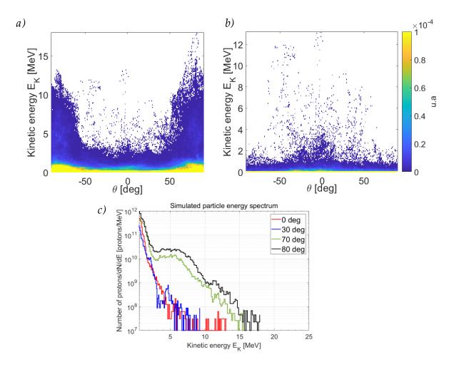
**Figure 4.22** Angular energy distribution of *a*) all forward accelerated protons and *b*) forward protons accelerated between  $x = 185 \mu m$  and  $x = 210 \mu m$  at t = 1.8 ps. c) Particle energy spectrum.
