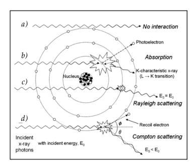
**Figure 5.1** Illustration of three X-ray interactions. *a)* unattenuated beam. *b)* the photoelectric effect, *c)* the Rayleigh scattering and *d)* the Compton effect. The figure is taken from [Seibert and Boone 2005].
