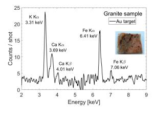
**Figure 5.24** X-ray spectra obtained when irradiating granite sample using the laser-based sources produced with an Au laser-interaction target.
