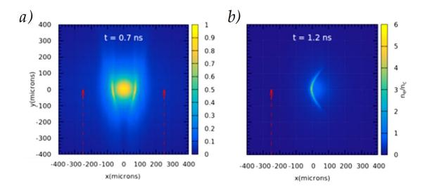
**Figure 6.4** 2D hydrodynamic simulations of the plasma shaping by a) two or b) one nanosecond lasers. The plasma electron density  $n_e/n_c$  is presented. Ns beams are propagating at -250 and + 250  $\mu$ m along the *y*-axis.
