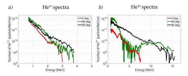
**Figure 4.27** Particle energy spectra at  $0^{\circ}$  (red),  $30^{\circ}$  (blue),  $60^{\circ}$  (green) and  $90^{\circ}$  (black) obtain with a mixed of helium and hydrogen gas-jet target.
