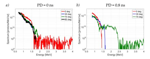
**Figure 4.12** Proton energy spectra at  $0^{\circ}$  (red),  $30^{\circ}$  (blue),  $70^{\circ}$  (green) and  $80^{\circ}$  (black) obtained with the laser focused at the center of the gas jet b) and reducing the ASE at half of the minimum achievable.
