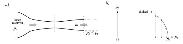
**Figure 3.9** *a*) Diagram of a nozzle, considering a duct with a throat, connected at its inlet to a very large reservoir with total pressure  $p_r$ . The *exit static pressure* is defined as  $p_e$  and the mass flow as  $\dot{m}$ . b)  $\dot{m}$  is presented as a function of  $p_e$ . As  $p_e$  decreases,  $\dot{m}$  increases. Until the duct is *chocked* and the mass flow no longer increases. The figure was taken from [Anderson 1990].
