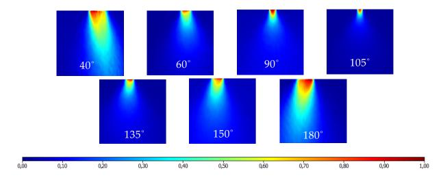
**Figure 3.31** Images of the phase shift taken at different rotation angles with *asymmetrical nozzles*. These pictures are produced with [Neutrino] and the phase shift is normalized to one.
