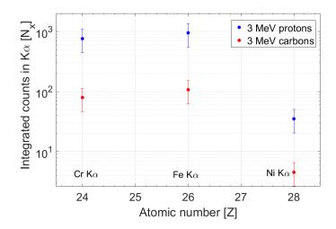
**Figure 5.16** Geant4 simulated number of counts in the Cr, Fe, and Ni  $K_{\alpha}$  peak when irradiating the stainless steel sample with 3 MeV protons (blue) and 3 MeV carbons (red) and scaled with the measured number of 3 MeV protons and carbons in the experiment.
