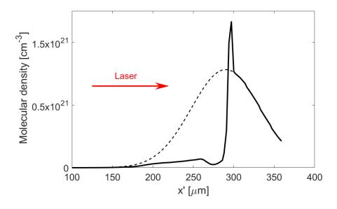
**Figure 4.16** Dashed line: initial density profile of the gas jet based on measurements. Solid line: density profile calculated with the FLASH code taking into account the laser ASE and used as input in the PIC simulations.
