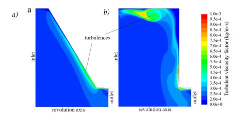
**Figure 3.23** Effect of the sharp discontinuity in the converging region on the turbulent viscosity factor. The figures represent half of the axisymmetric nozzle view where the lower line is the revolution axis. The inlet is in the left and the outlet is in the right of each figure: a) a 59° convergent cone and b) a 90° transition.
