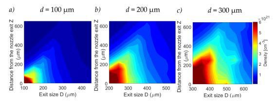
**Figure 3.16** Interpolated contour maps of the molecular density at 1000 bar of hydrogen at different distances from the nozzle exit z as a function of the exit size D for three throat diameters (L is fixed) a) d = 100  $\mu$ m, b) d = 200  $\mu$ m and c) d = 300  $\mu$ m.
