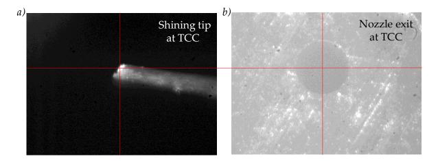
**Figure 4.4** Pictures from the bottom view CCD in the second experiment *a*) of the illuminated tip at TCC *b*) of the nozzle at TCC. The red cross represents TCC.
