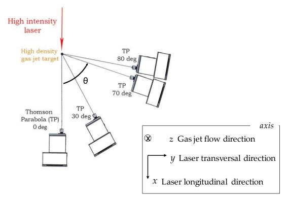
**Figure 4.1** Experimental setup at the LULI facility. PICO2000 high-power laser is impinging on the high-density gas-jet target. Four TPs equipped with IPs are placed at  $0^{\circ}$ ,  $30^{\circ}$ ,  $70^{\circ}$ , and  $80^{\circ}$  with respect to the laser axis, 50 cm away from the gas-jet target.
