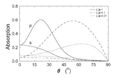
**Figure 2.8** Numerical solution of angular absorption coefficients for various *density scale–lengths* ( $L/\lambda$ ). Taken from [Gibbon 2005].
