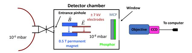
**Figure 3.48** Schematic of the TP-MCP used at the EMT-INRS center. The detector is in a different vacuum chamber allowing a differential vacuum and the possibility of opening the main chamber without breaking the vacuum in the detector chamber. The real photo is in **Figure 3.49** [Paper III].
