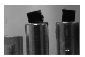
Figure 3.5 a) Target alignment bench (TAB) to pre-align the solid targets outside the vacuum chamber b) Picture is taken with one of the cameras of the multi-holder target. A 20  $\mu$ m diameter tungsten pin is in one holder target to do a first precise alignment. 5  $\mu$ m thickness copper targets are on the right of the picture, displayed from the front.
