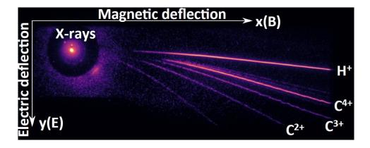
Figure 3.50 MCP image obtained from the TP spectrometer with a Cu target. Taken from [Paper VII].
