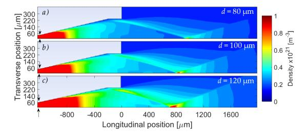
**Figure 3.19** Molecular density maps at 1000 bar of hydrogen for different throat diameters d. The longitudinal position is normalized to z = 0 at the exit of the nozzles. a)  $d = 100 \, \mu m$ , b)  $d = 200 \, \mu m$  and c)  $d = 300 \, \mu m$ . The red color at the entrance of the nozzle can represent molecular densities larger than  $1 \times 10^{21} \, \text{cm}^{-3}$ .
