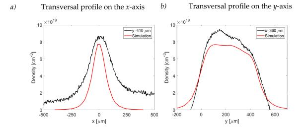
**Figure 3.34** Density profile measured by TomoRaw (black) and compared with FLUENT simulations (red) for *a*) the transversal profile on the *x*-axis *b*) the transversal profile on the *y*-axis.
