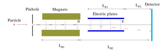
**Figure 3.43** Schematic of a Thomson parabola TP spectrometer.  $L_{B_1}$  and  $L_{E_1}$  is the magnet and electric plates length and  $L_{B_2}$  and  $L_{E_2}$  the distance from the magnet or the electric plates to the detector.
