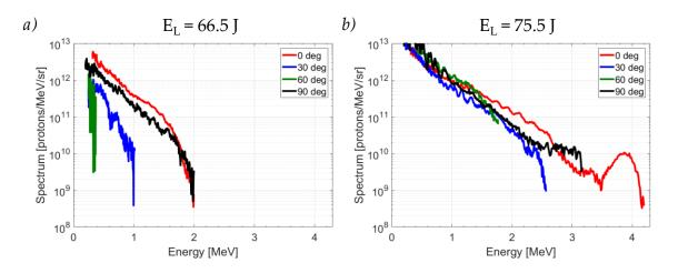
**Figure 4.10** Proton energy spectra at 0° (red), 30° (blue), 60° (green) and 90° (black) obtained with the laser focused at the rising slope of the *asymmetrical nozzle* jet density profile at  $z = 200 \mu m$ . The orientation is probably different in figure a) and b).
