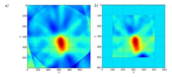
**Figure 3.32** Reconstruction of the phase shift at 200  $\mu$ m of the *asymmetrical nozzles* exit with TomoRaw program. *a)* Using one iteration series between each pair of images *b)* Using two interaction series and a mask to avoid the erroneous interferences of the reconstruction from the overlapping borders. Both images are normalized to 1.
