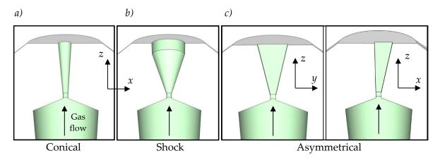
**Figure 3.13** 3D presentation of different types of nozzles. *a)* convergent-divergent nozzle similar to the *Laval nozzle*: *conical nozzle*. *b)* Divergent-convergent nozzle with an edge at the exit of the nozzle: *shock nozzle*. *c)* A more complex nozzle as a rectangular one: *asymmetrical nozzle*.
