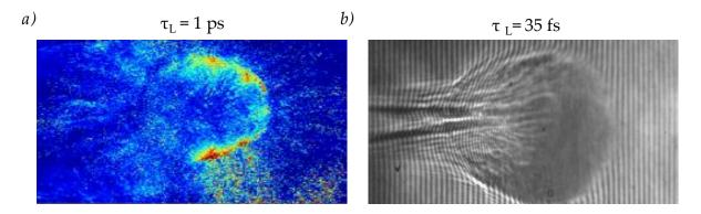
**Figure 4.24** *a)* Laser collapse at 3.6 ps shown in our PIC simulation, with a laser pulse of 1 ps FWHM *b)* Laser collapse from electron density interferogram with a laser pulse of 35 fs FWHM taken from [Sylla 2013].
