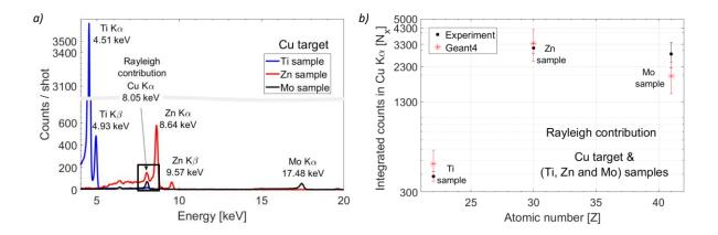
**Figure 5.17** *a)* X-ray spectra as obtained by the interaction of laser-based sources produced by a Cu target and a Ti, Zn and Mo samples. The Rayleigh contribution from the Cu X-rays is visible around 8 keV (see black box). *b*) Integrated number of counts in the Cu  $K_{\alpha}$  Rayleigh peak in Geant4 simulations when 8.05 keV photons are sent on the sample, scaled to  $4.3 \times 10^{10} \pm 1.1 \times 10^{10}$  incident photons/sr.
