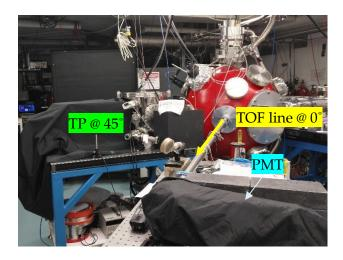
Figure 3.41 The first ALLS configuration. TOF line coupled with an PMT at  $0^{\circ}$ . On the left, at  $45^{\circ}$ , the TP spectrometer.
