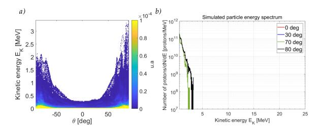
**Figure 4.20** *a*) Angular energy distribution of forward ( $p_x \ge 0$ ) accelerated protons at t = 1 ps. *b*) Particle energy spectrum  $p_x \ge 0$  at t = 1 ps.
