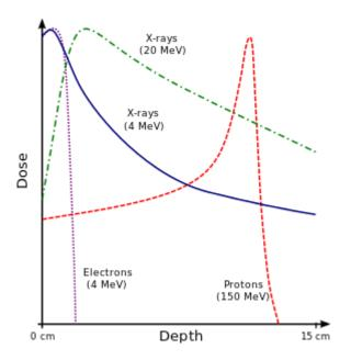
**Figure 1.2** Example of energy deposition for protons (150 MeV) in water compared with X-rays (20 and 4 MeV) and electrons (4 MeV). From wikicommons by Cepheiden.
