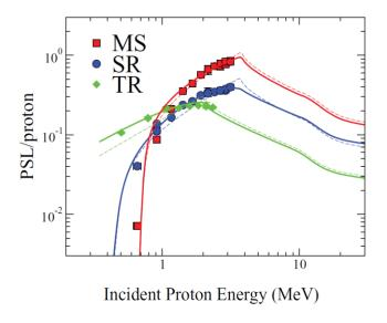
**Figure 3.47** Response function R(E) of BAS-MS, BAS-SR, and BAS-TR IPs. The symbols represent the data from [Bonnet 2013]. For more information [Bonnet 2013].
