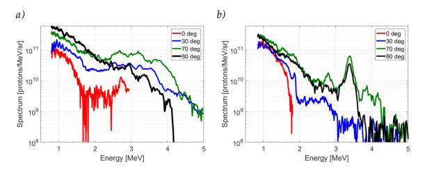
**Figure 4.14** Proton energy spectra at 0° (red), 30° (blue), 70° (green) and 80° (black) obtained with the laser focused at the rising slope of the jet density profile.
