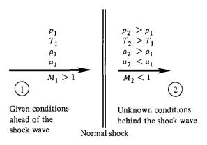
Figure 3.7. Diagram of a normal shock. From [Anderson 1990].
