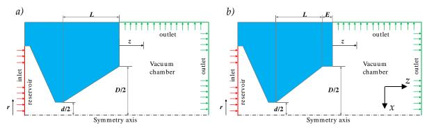
**Figure 3.14** Scheme of the 2D axisymmetric nozzle geometries for *a) conical nozzles* and *b) shock nozzles* used in CFD simulations (see text for details).
