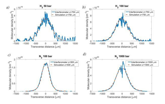
**Figure 3.30** Comparison of simulation results with interferometry reconstructions for *a*) 50 bar diatomic hydrogen at  $z = 750 \ \mu m \ b$ ) 100 bar diatomic hydrogen at  $z = 750 \ \mu m \ c$ ) 100 bar diatomic nitrogen at  $z = 500 \ \mu m \ d$ ) 1000 bar diatomic nitrogen at  $z = 1000 \ \mu m$ .
