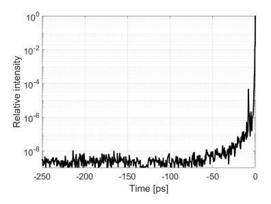
**Figure 3.3** ALLS 100 TW laser system temporal spectrum. On the right, the main laser pulse. The smaller peak on the left (at t = 15 ps) is not real, it is just an artifact of the auto-correlation measurement. The figure shows a contrast of  $< 10^{-8}$  at 100 ps before the main pulse.
