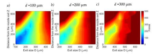
**Figure 3.17** The FWHM interpolated contour maps at 1000 bar of hydrogen at different distances from the nozzle exit z as a function of the exit size D for three throat diameters (L is fixed) a)  $d = 100 \, \mu m$ , b)  $d = 200 \, \mu m$  and c)  $d = 300 \, \mu m$ .
