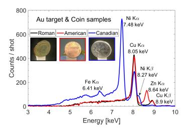
**Figure 5.26** X-ray spectra obtained when irradiating a Roman (black), American (red) and Canadian (blue) coin samples using the laser-based sources produced with Au target.
