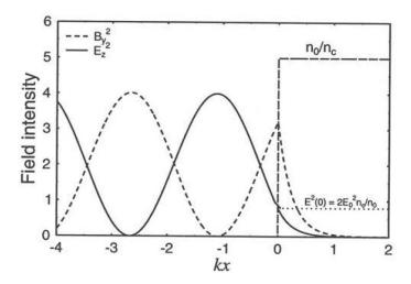
**Figure 2.9** Normally incident electromagnetic fields in an over-dense plasma *skin-layer* with  $n_0/n_c$  = 5 and  $E_0$  = 1. Taken from [Gibbon 2005].
