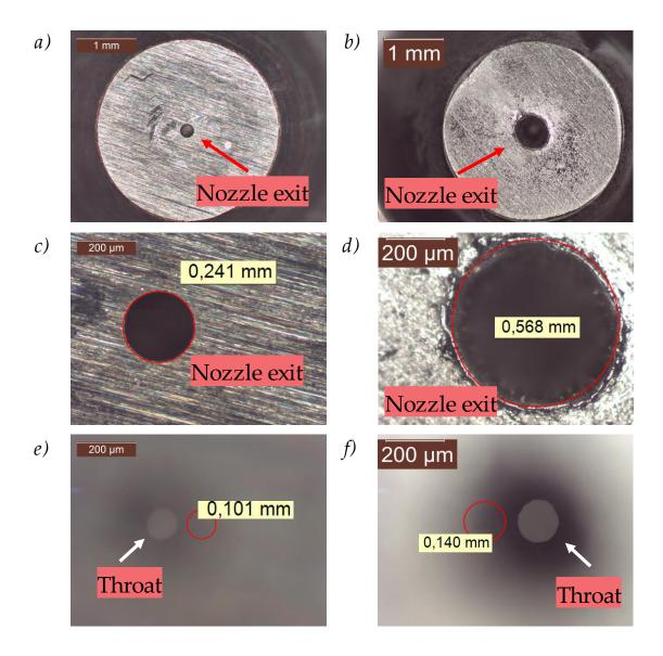
**Figure 6.1** On the left, pictures of the nozzle before the shot. On the right, pictures of the nozzle after one shot. *a*), *b*), *c*) and *d*) show the nozzle exit. *e*) and *f*) show the nozzle throat.
