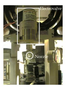
Figure 3.6 Picture of the nozzle and the electro-valve at the LULI laser facility. The nozzle is upside down.
