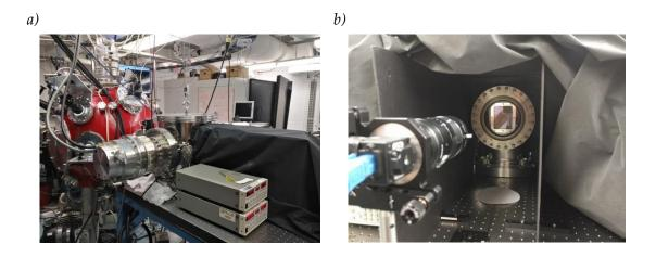
**Figure 3.49** *a)* Picture of the detector chamber connected to the *boule rouge* at EMT-INRS center. *b)* Picture of the CCD pointed at the MCP inside the detector chamber. The picture is taken under the black blanket on the right of picture *a)*.
