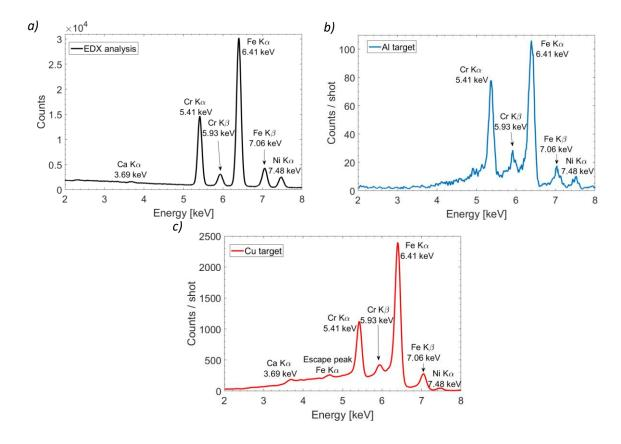
**Figure 5.18** Stainless steel sample analysis: *a)* EDX spectrum; *b)* and *c)* X-ray spectra obtained by a single shot irradiation, using the laser-based sources produced with a low Z (Al, blue) and high Z (Cu, red) target respectively
