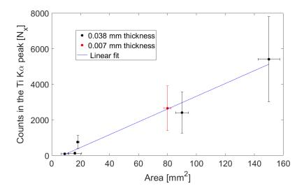
**Figure 5.20** Integrated number of counts in the Ti  $K_{\alpha}$  peak for different sample sizes using the laser-based sources produced by Cu or Au targets.
