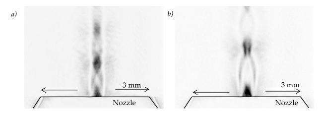
**Figure 3.26** Mach waves generated by the designed *conical nozzle* fed with *a)* 10 bar and *b)* 20 bar of nitrogen propagating through 1 bar air. Mach waves are formed at different distances and propagate until they collapse.
