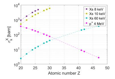
**Figure 5.7**. X-ray  $K_{\alpha}$  cross-sections as a function of Z. In purple squares, X-ray  $K_{\alpha}$  cross-sections induced by 8 keV X-rays, in green squares by 10 keV X-rays, in blue squares by 60 keV X-rays and in pink bullets by 4 MeV protons. XRF values are taken from XRAYLIB 2.3 data library.
