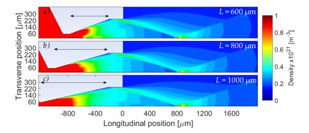
**Figure 3.22** Molecular density maps at 1000 bar for different nozzle lengths L with D and d constant. The longitudinal position is normalized to z = 0 at the exit of the nozzles. a) L = 600  $\mu$ m nozzle length, b) L = 800  $\mu$ m nozzle length and c) L = 1000  $\mu$ m nozzle length. The red color at the entrance of the nozzle can represent densities larger than 1  $\times$  10<sup>21</sup> cm<sup>-3</sup>.
