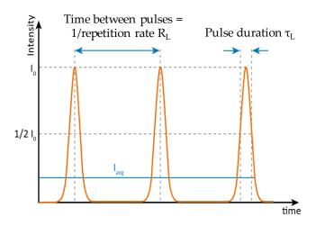
**Figure 2.3** Representation of the laser pulse intensity. The repetition rate  $R_L$  and the pulse duration  $\tau_L$  are represented in the image [the picture is taken from www.silloptics.de].
