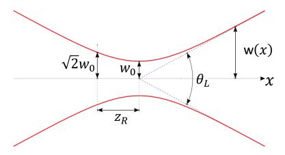
**Figure 2.4** Scheme of a laser beam propagation where w(x) is the beam *spot radius* and  $w_0$  is the *beam waist*,  $\theta_L$  is the divergence and  $z_R$  is the *Rayleigh length*.
