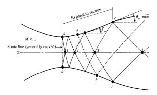
Figure 3.11 Schematic of a supersonic nozzle design in two dimensions. From [Anderson 1990].
