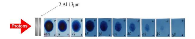
Figure 3.36 Example of an RCF stack irradiated by a proton beam at LULI laser installation. The proton beam traverses the stack from the left to the right. The proton beam has 2 cm spot size at 3.5 cm from the production source where it is almost punctual. The energy of this shot was 23 J, the pulse duration 300 fs, i.e. an intensity of  $2 \times 10^{19}$  W/cm<sup>2</sup>. [Plaisir 2010]
