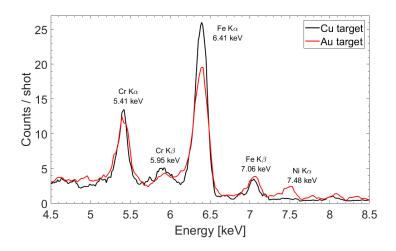
Figure 5.21 XPIF background signal with no sample inside the auxiliary chamber.
