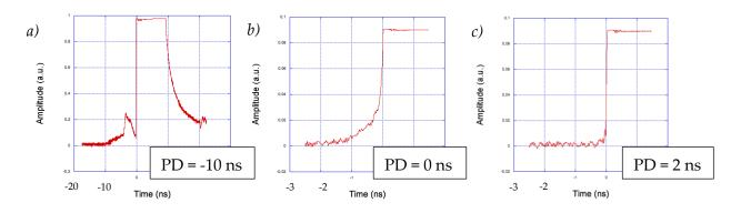
**Figure 3.2** Time spectra for PICO2000 laser for different *Pockel cells delays* (PD). The figures are provided by LULI. The main pulse, on the right of each figure, is saturated. *a)* PD = -10 ns: no delay is applied. The nanosecond ASE is present before the main pulse. *b)* PD = 0 ns: the ASE level is reduced *c)* PD = 2 ns: the level of ASE is further decreased but the duration of the main pulse starts to increase.
