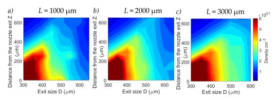
**Figure 3.18** Contour maps of the density at 1000 bar at different distances from the nozzle exit z as a function of the exit size D for three lengths (d= 300  $\mu$ m fixed): a) L = 1000  $\mu$ m b) L = 2000  $\mu$ m and c) L = 3000  $\mu$ m.
