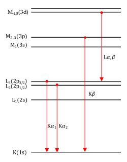
**Figure 5.4** Energy level diagram and the possible transitions from L and M to K shell, from M to L shell and their denotations.
