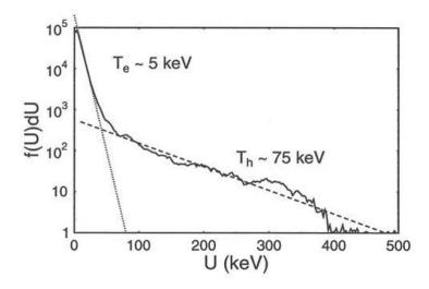
**Figure 2.11** Typical bi-Maxwellian electron distribution resulting from collisionless heating by a laser. This example taken from [Gibbon 2005]; it was obtained from a 1D PIC simulation with a laser irradiance  $5 \times 10^{16} \text{W/(cm}^2 \mu \text{m}^2)$  incident at  $45^\circ$  onto a plasma with  $n_e/n_c = 3$ .
