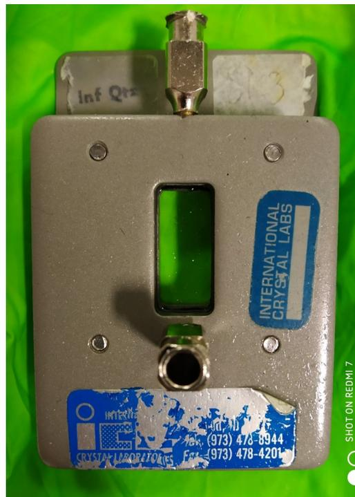
**Figure II.38:** Sealed liquid cell.
