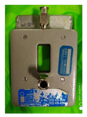
Figure II.38: Sealed liquid cell.
