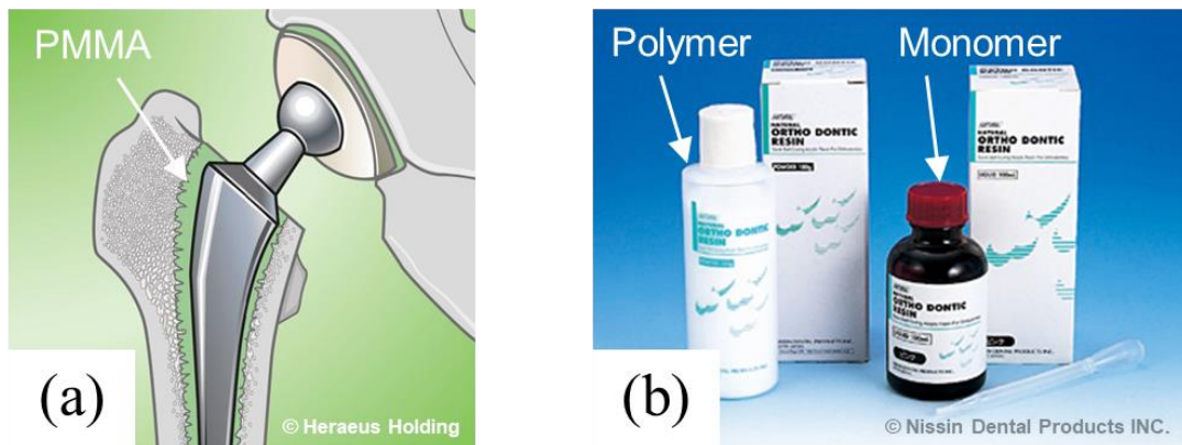
Fig. 3-1 Usage examples of PMMA in medical fields: (a) bone cement, (b) acrylic dental resin
