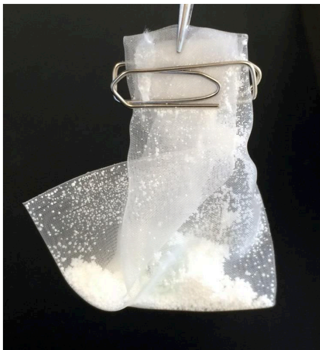
SI Figure 1: Design of the XAD ® -2 insert
