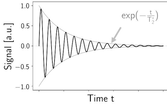
Figure 1.1-4: Free induction decay signal representation, showing the signal that oscillates at the carrier frequency (128 MHz at 3 T), weighted by a decreasing exponential caused by  $T_2^*$  decay. No values are shown on the time axis, as in this simple representation, for the sake of readability, the frequency is orders of magnitude lower than in reality.
