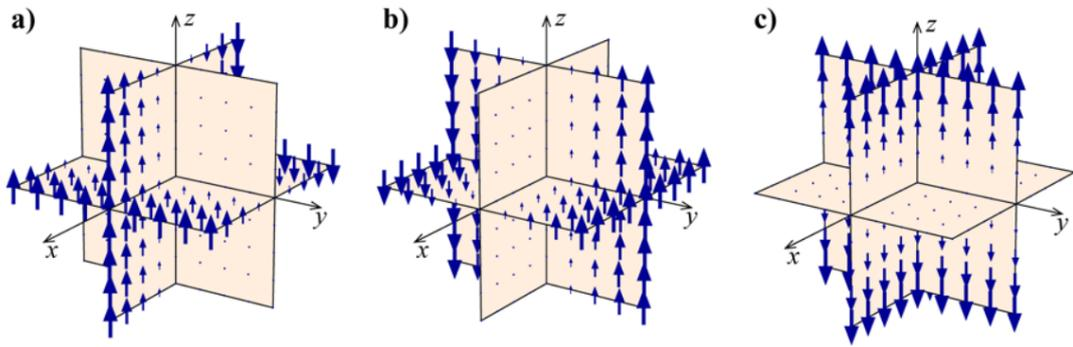
Figure 1.2-5: Diagrams of the  $B_z$  component of the 3D magnetic field variation of a)  $G_x$ -, b)  $G_y$ -, and c)  $G_z$ -gradients. The field is aligned with the direction of the arrows. The scale of the arrows indicates the magnitude of the magnetic field strength at that point. From [Poole 2007].
