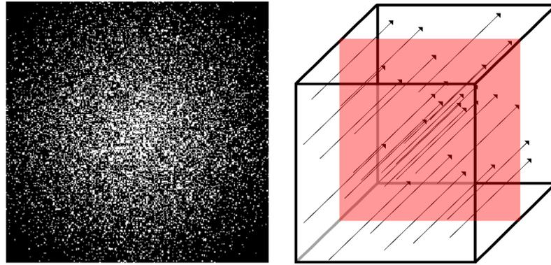
Figure 2.2-2: 3D acquisition with 2D Poisson disk sampling. From [Chauffert 2015]. The readout is performed along the horizontal lines with black arrows, namely orthogonally to the 2D cross-section along which isolated points have been drawn.
