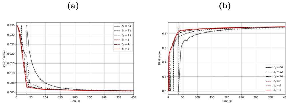
Figure 5.4-12: Fast online reconstruction of 8-fold ( $S = 64$  shots) prospectively accelerated Sparkling scan of ex vivo human brain in a multi-channel coil acquisition setup. Evolution over time of (a) the cost function in Eq. (5.9) and of (b) the SSIM score for increasing values of batch size  $b_s$ . The dark dashed line marks the end of acquisition.
