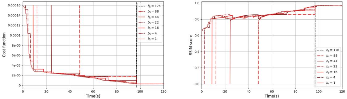
Figure 5.3-2: Single-channel retrospective Cartesian reconstruction: (a) evolution over time of cost function in Eq. (5.5) and (b) of the SSIM score for different batch sizes  $b_s$ . The dark dashed line marks the end of acquisition.
