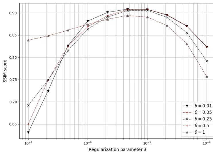
Figure 3.4-5: Impact of sensitivity profiles estimation on the final reconstructed image quality. The last two settings ( $\theta \in \{0.5, 1\}$ ) yield superimposed traces indicating that there is no gain in collecting high-frequency information for the recovery of sensitivity profiles.
