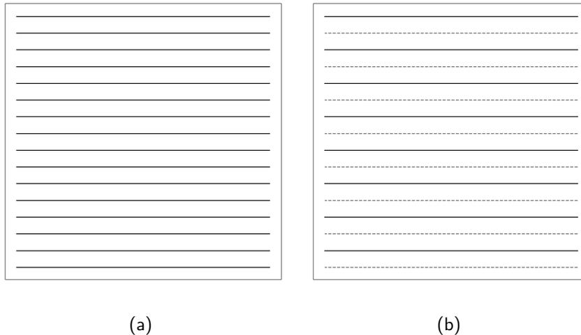
Figure 1.3-14: (a) Fully sampled Cartesian k-space. (b) Acquired k-space for parallel imaging with an acceleration factor  $R = 2$ . Dashed lines represent the missing samples while solid lines correspond to the acquired k-space values. Horizontal axis represents the frequency encoding direction and vertical axis is the phase-encoding one.
