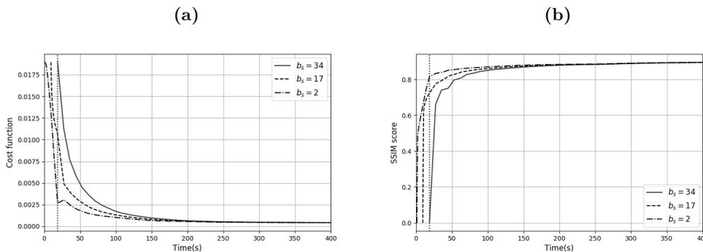
Figure 5.4-13: Fast online reconstruction of 15-fold ( $S = 34$  shots) prospectively accelerated Sparkling scan of ex vivo human brain in a multi-channel coil acquisition setup. Evolution over time of (a) the cost function in Eq. (5.9) and of (b) the SSIM score for batch sizes  $b_s = 2$ ,  $b_s = 17$  and  $b_s = 34$ . The dark dashed line marks the end of acquisition.
