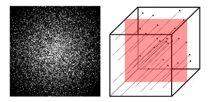
Figure 2.2-2: 3D acquisition with 2d Poisson disk sampling. From [Chauffert 2015]. The readout is performed along the horizontal lines wih black arrows, namely orthogonally to the 2d cross-section along which isolated points have been drawn.
