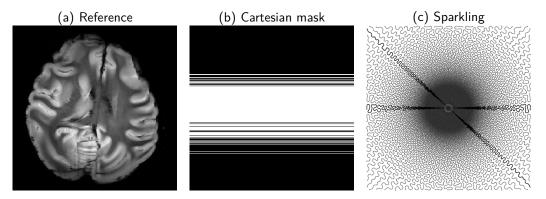
Figure 5.3-1: Single-channel coil acquisition: (a) ex vivo baboon brain Cartesian reference image, (b) retrospective Cartesian under-sampling scheme (AF = UF = 2.9), (c) prospective non-Cartesian Sparkling sampling scheme (implemented with a golden-angle ordering, two consecutive shots are highlighted in black) (AF = 15, UF = 2.5), the first collected being the horizontal one and the rotation being counterclockwise.
