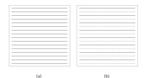
Figure 1.3-14: (a) Fully sampled Cartesian k-space. (b) Acquired k-space for parallel imaging with an acceleration factor R = 2. Dashed lines represent the missing samples while solid lines correspond to the acquired k-space values. Horizontal axis represents the frequency encoding direction and vertical axis is the phase-encoding one.
