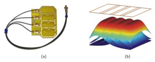
Figure 1.3-12: (a) Four coil phased array showing overlapping coils, (b) their associated sensitivity maps. From [Gruber 2018].
