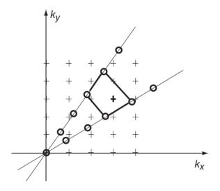
Figure 1.2-8: Grid-driven interpolation, the value at any Cartesian grid point (+) is computed as the interpolation (*e.g.* bilinear) of the four surrounding non-Cartesian points (o). The interpolation kernel is a user-defined parameter of grid-driven methods, tat can be either linear, cubic, or based on the nearest neighbor algorithm.
