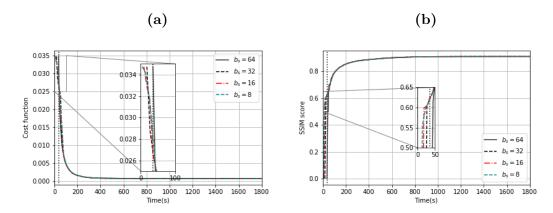
Figure 5.4-7: Online reconstruction of 8-fold (S = 64 shots) prospectively accelerated Sparkling scan of ex vivo human brain in a multi-channel coil acquisition setup. Evolution over time of (a) the cost function in Eq. (5.9) and of (b) the SSIM score for increasing values of batch size  $b_s$ . The dark dashed line marks the end of acquisition.
