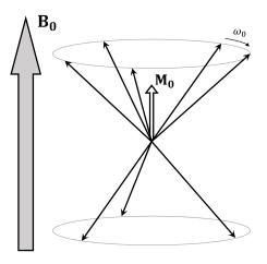
Figure 1.1-1: Classical representation of macroscopic net magnetization  $M_0$  (hollow vector) in an isochromat consisting of several adjacent spins immersed in an external static magnetic field ( $B_0$ , grey vector). It is induced by the slight excess of magnetic moments (black vectors) parallel to  $B_0$ , compared to anti-parallel ones.  $\omega_0$  is the Larmor angular frequency at which each spin precesses around  $B_0$ . From [Tomi-Tricot 2018, ch. 1].
