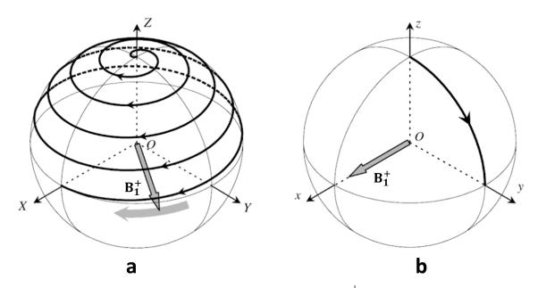
Figure 1.1-2: Effect on macroscopic magnetization of a  $B_1^+$  field rotating at the Larmor frequency  $\omega_0$  viewed (a) from laboratory frame (**XYZ**) where  $B_0$  is aligned with the **Z** axis. (b) It is generally convenient to represent it in a rotating frame of reference (**xyz**) of frequency  $\omega_{rf}$ , where  $B_1^+$  lies along with the **x** axis. The **z** axis is aligned with **Z**. From [Tomi-Tricot 2018].
