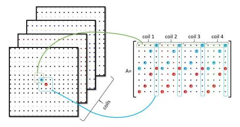
Figure 3.2-3: Left: Set of k-spaces obtained within the multi-coil setting. Right: the calibration matrix A is obtained by sliding a window (small green frame) on the calibration data  $y_{\Omega}^{AC}$  (blue frame).
