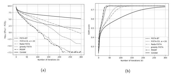
Figure 2.3-8: Comparison of the convergence speed of different proximal algorithms to solve Eq. (2.17). The Nesterov ripples can be seen from the FISTA-CD proposed by [Chambolle 2015]. From [Ramzi 2019].
