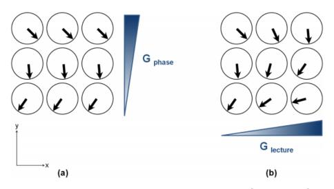
Figure 1.2-6: Encoding the k-space line by line. From [Le Ster 2017].
