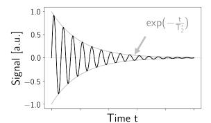
Figure 1.1-4: Free induction decay signal representation, showing the signal that oscillates at the carrier frequency (128 MHz at 3 T), weighted by a decreasing exponential caused by  $T_2^*$  decay. No values are shown on the time axis, as in this simple representation, for the sake of readability, the frequency is orders of magnitude lower than in reality.
