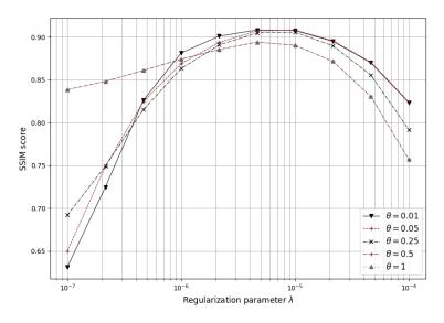
Figure 3.4-5: Impact of sensitivity profiles estimation on the final reconstructed image quality. The last two settings ( $\theta \in \{0.5, 1\}$ ) yield superimposed traces indicating that there is no gain in collecting high-frequency information for the recovery of sensitivity profiles.
