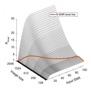
Figure 3.1-1: A view of the maximum under-sampling factor allowing SSIM scores above 0.9 as a function of image size (or resolution as the FOV is fixed) and input SNR. Orange line: Available input-SNR on the 7T scanner (Siemens-Healthineers, Erlangen, Germany). [Lazarus 2018c].
