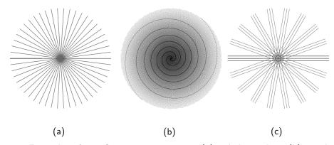
Figure 3.2-2: Examples of non-Cartesian trajectories: (a) radial sampling, (b) spiral sampling, (c) PROPELLER sampling. Oversampling the center of k-space brings a gain in robostness to the patient's motion.
