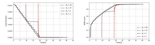
Figure 5.3-4: Online reconstruction of 15-fold (S = 34 shots) prospectively accelerated Sparkling scan of ex vivo baboon brain in a single-channel coil acquisition setup. Evolution over time of (a) the cost function in Eq. (5.5), and of the SSIM score in (b) for batch sizes  $b_s$ corresponding to the primary factors of S. The dark dashed line marks the end of acquisition.
