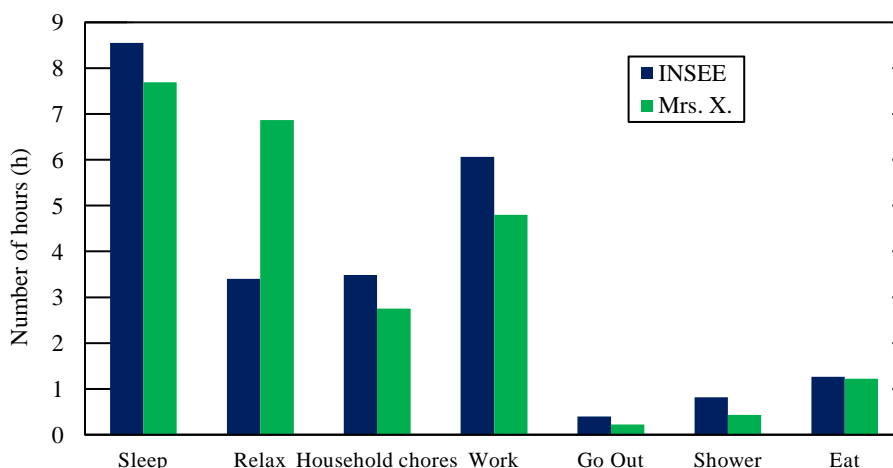
Figure II.2.11 Comparison of the average number of hours spent in one day at each activity obtained by INSEE (Degenne et al. 2012) and Li-BIM
