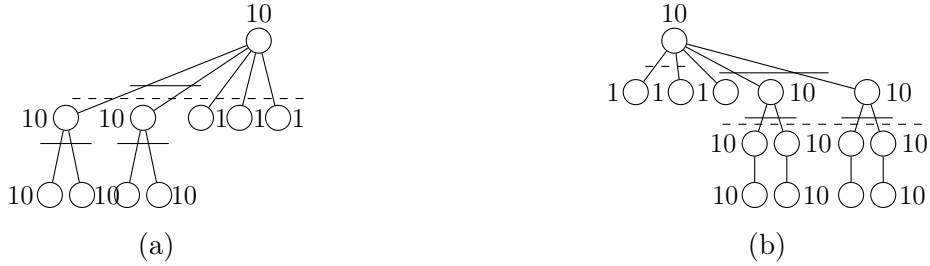
Figure 2.3 – Two cases where SPLITSUBTREES is suboptimal. Dashed edges represent the solution of SPLITSUBTREES, plain edges give the optimal partition.
