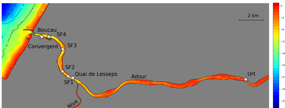
Figure 1.10: Map of the study site, where white stars named SF1 to SF4 represent the location of measurement, the ones named Boucau, Convergent and Urt represent the location of tide gauges. Colors represent depth in meter.
