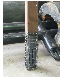
Figure 1.14: a) Panoramic view of the location where the YSI 6920 has been fixed, b) YSI probe inside its protecting structure.
