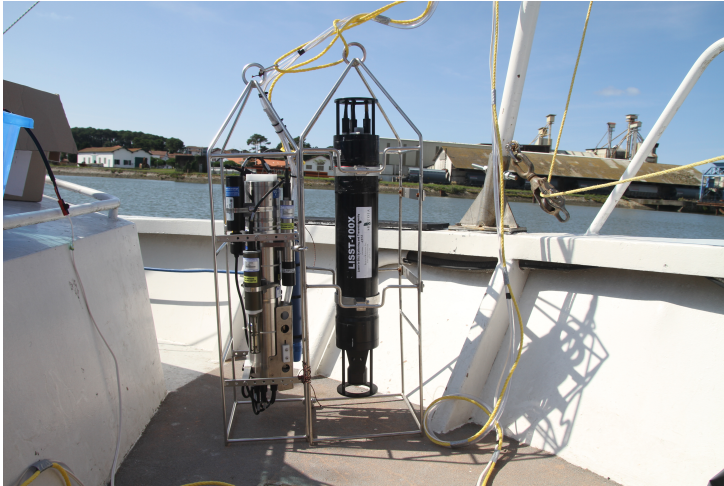
Figure 1.12: a) Frame used in September 2017 with a LISST-100X, a Seabird C19+, and a water pump. b): Frame used in June and September 2018 with a YSI 6920, a Seabird C19+, and a water pump.
