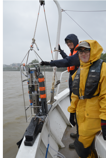
Figure 1.12: a) Frame used in September 2017 with a LISST-100X, a Seabird C19+, and a water pump. b): Frame used in June and September 2018 with a YSI 6920, a Seabird C19+, and a water pump.
