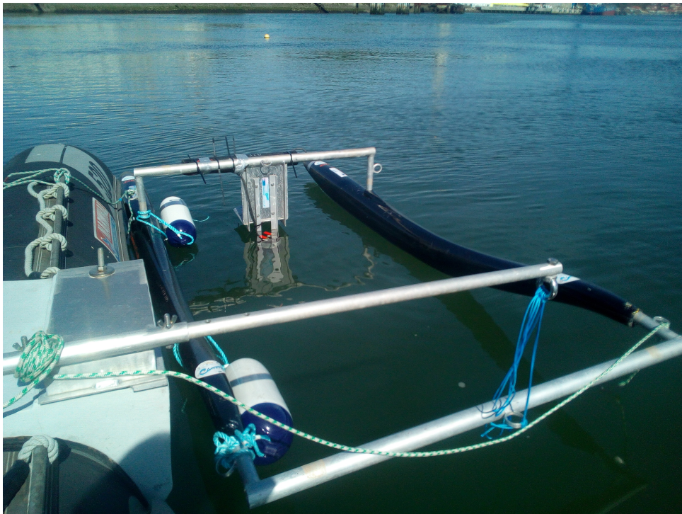
Figure 1.13: Catamaran equipped with a Nortek Signature 1000 and fastened to a semi-rigid craft, used during the field campaign in September 2017.
