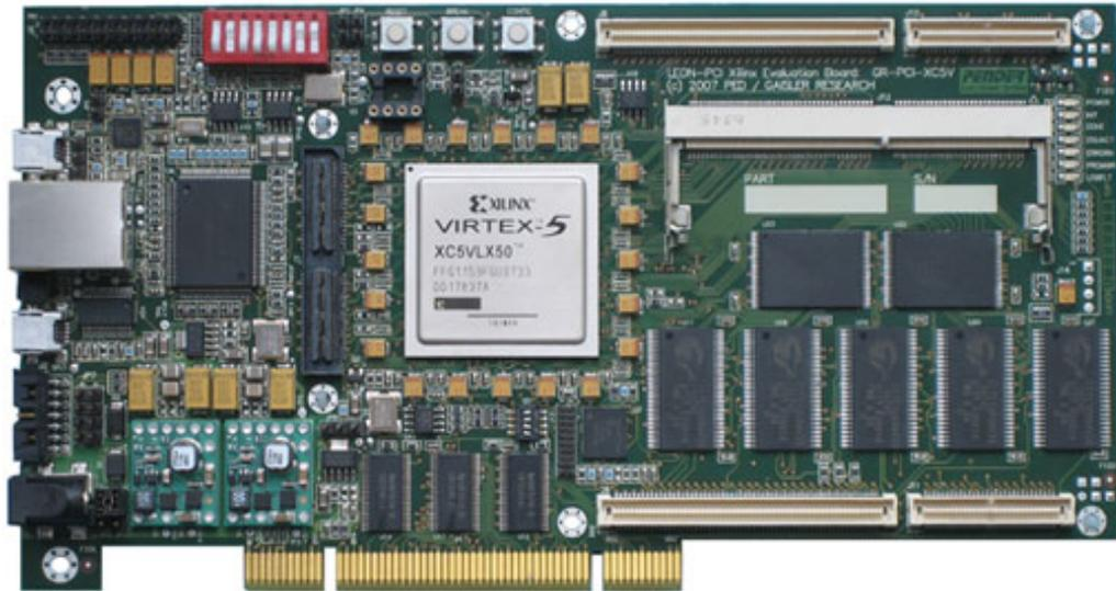
Figure 4.7: Gaisler board used for the LEON3 prototype
