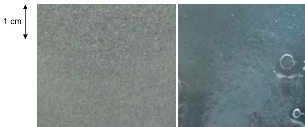
Figure III.1 : Homogeneity of the 3-Mercaptopropyl-functionalized silica dispersion in binding gel in agarose (left) or in polyacrylamide (right)
