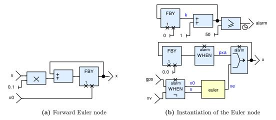
Figure 1.1: SCADE graphical representation
