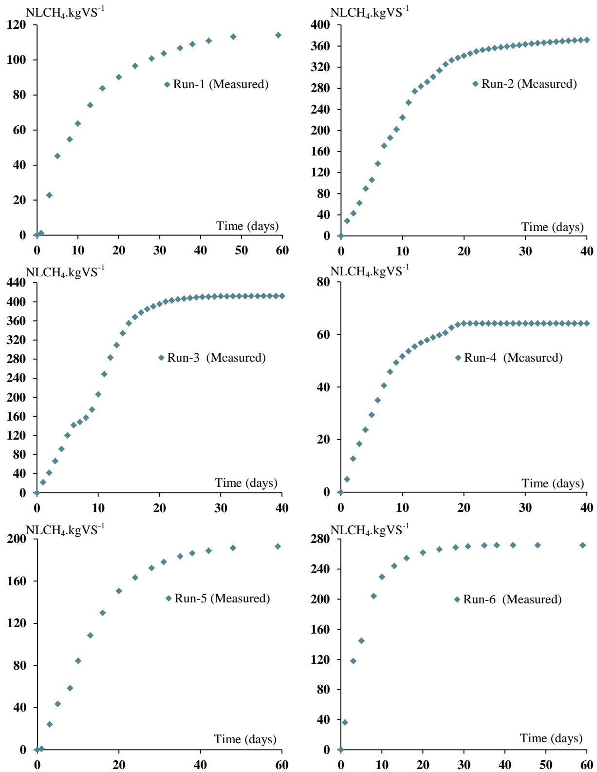
Figure 17: Cumulative methane production for the runs 1 to 6
