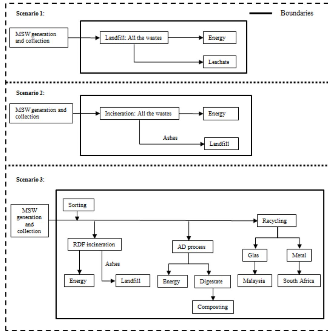
Figure 12: LCA model and boundaries for each scenario.
