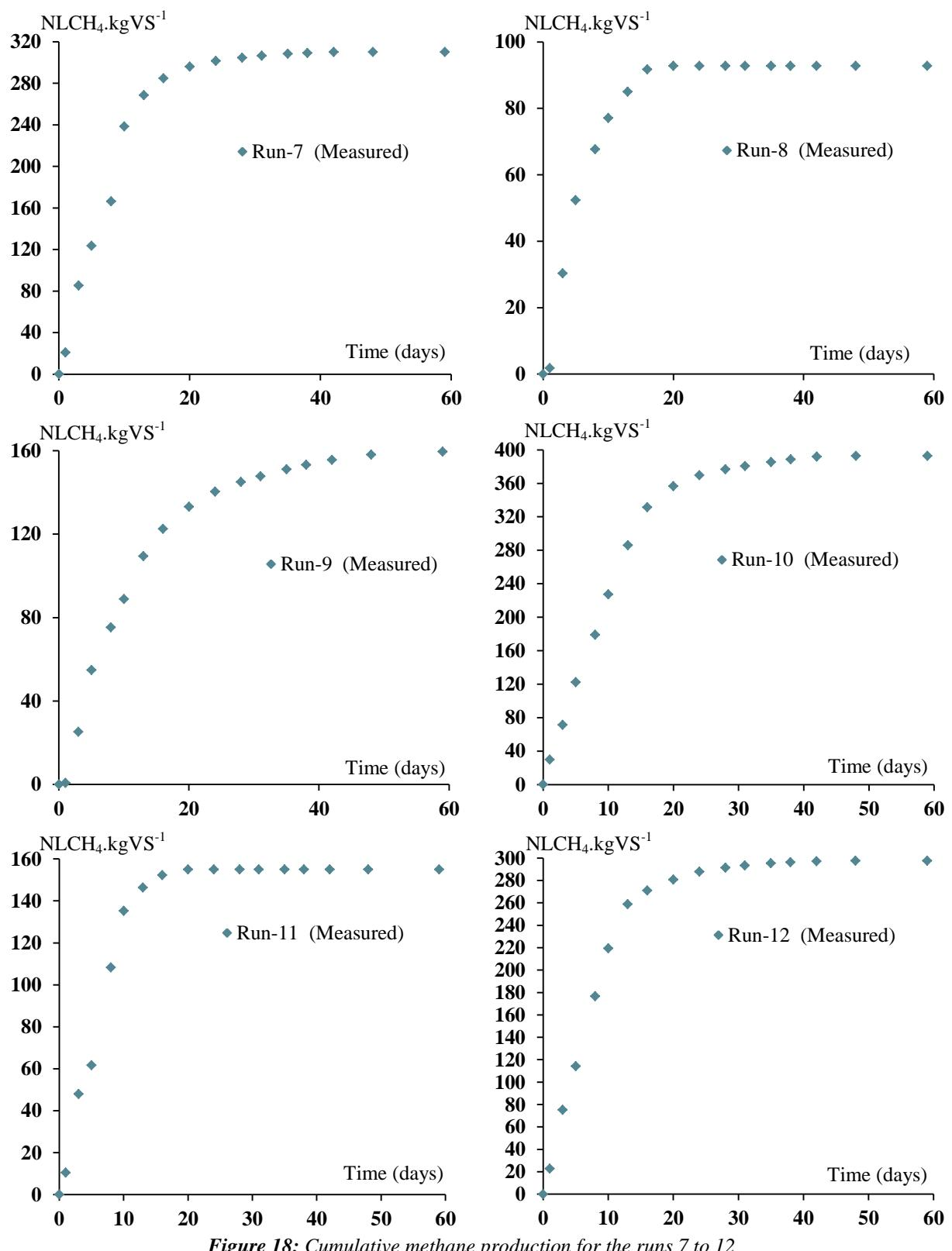
Figure 18: Cumulative methane production for the runs 7 to 12
