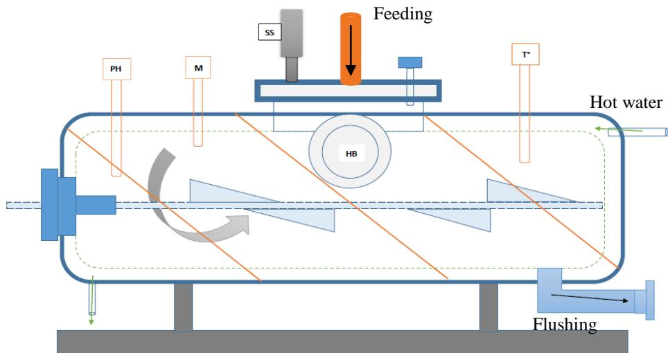
*Figure 32: Pilot scale anaerobic digester schematic representation*
