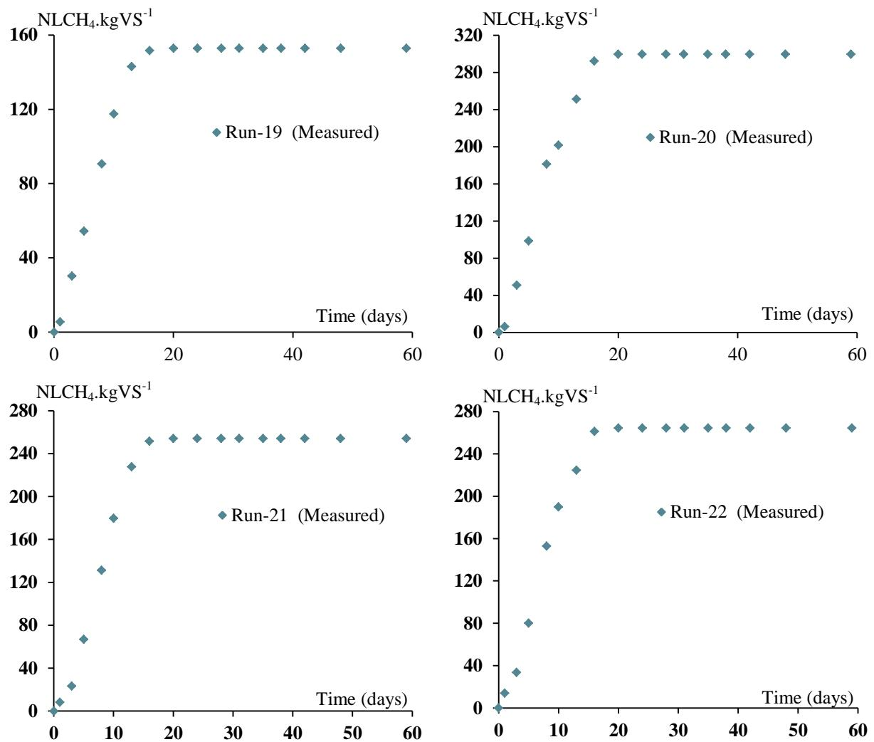
**Figure 20:** Cumulative methane production for the run 19 to 22
