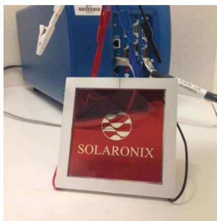
Figure 3.12 Commercial Dye-sensitized solar cell; fabricated by Solaronix PICTO 1010DEMO 114 mm × 114 mm; Ref 52101/Red; total thickness  $\approx$  1 cm). It is composed of FTO electrodes with a surface resistivity of 15 ohm/square. This DSSC is used as a reference for our DSSC experiments in our prototype (Minucell).
