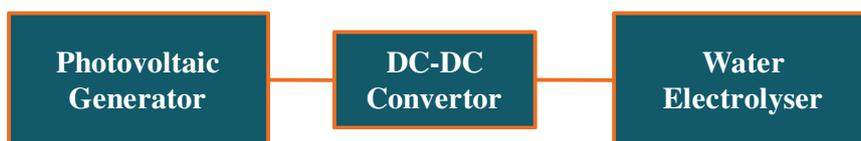
Figure 1.6 Indirect coupling of PV and water electrolysis system via DC-DC converter.
