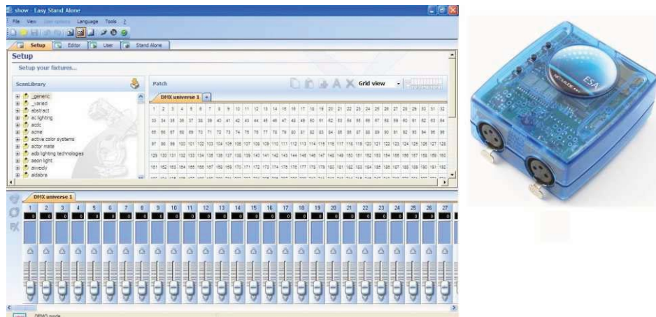
Figure 3.5. Picture of ESA Pro software and U9 Standalone controller. The software permits to adjust the light intensity. The controller box makes the connection between software and LED panel. The light intensity varies by displacing the cursor along the corresponding port (several ports are considered in the software, but one of them has action on the panel).
