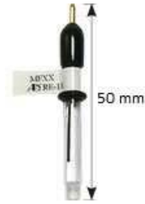
Figure 3.27 RE-1S silver, silver chloride reference electrode, OD: 4.5mm \times L: 50 mm. The Ag electrode is submerged in 3 M NaCl solution. The electrode is appropriate to be used in aqueous solutions.
