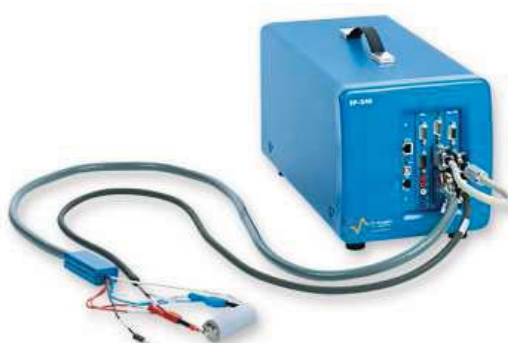
Figure 3.25 SP-240 potentiostat, 4A research grade, distributed BioLogic can work at the voltage range of -3V up to 14V and provides the current between the ranges of 1 \mu A – 4 A. It permits to carry out the data acquisition which will be then interpreted and traced by EC-Lab software. Several electrochemical techniques are provided and supported by EC-Lab such as general voltamperometric (Cyclic Voltammetry, Chronopotentiometry) techniques, impedance techniques, and a technique builder including modular potentiostat and galvanostat.
