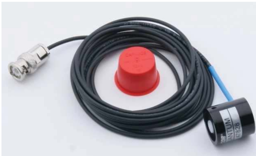
Figure 3.6 Flat panel sensor, LiCor, Li-190SA is able to measure directly the micromole of photons. The measured micromole of photons with flat sensor corresponds to hemispheric photon flux.
