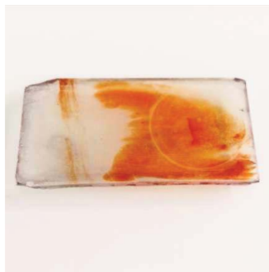
Figure 3.23 Hematite electrode, fabricated by anodic deposition of FeOOH from solution of \text{Fe}^{2+} , (pH 4). The final film is obtained after heating the electrode up to 520^\circ\text{C} . The thickness of deposition can be varied by regulating the time of FeOOH deposition and the annealing temperature.
