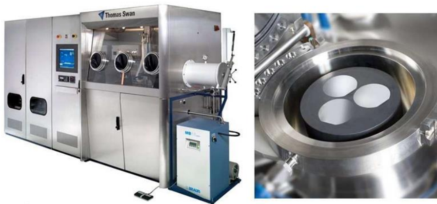
Figure 2.2: The Thomas Swan (Aixtron) 3x2'' CCS MOVPE reactor (left). View on the susceptor with three 2'' substrates (right). (Ref. 3)
