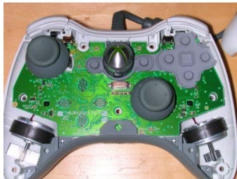
Figure 2-3 – Videogame controller with force feedback motors
