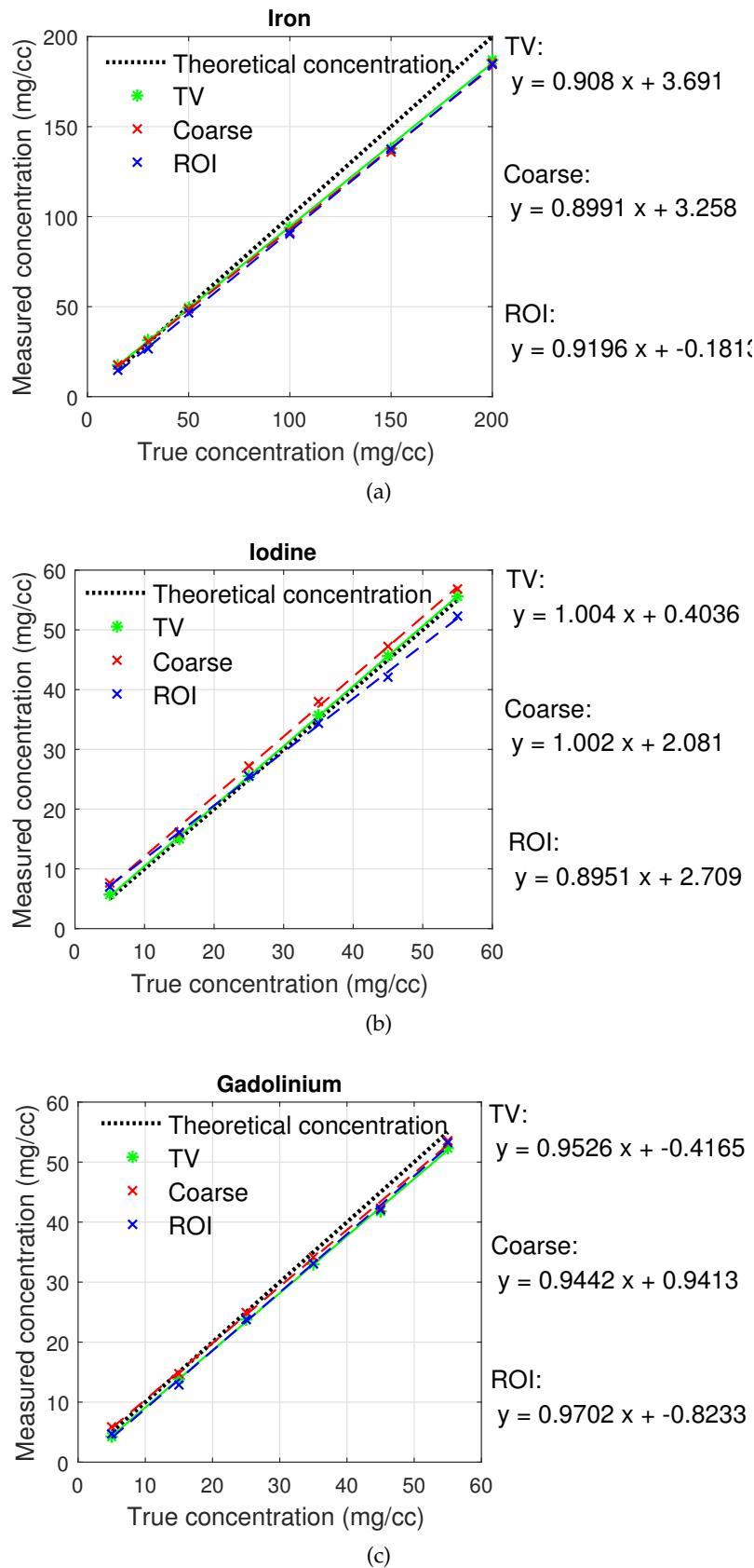
Figure 4.5: The linear regressions of material decomposition using three methods for (a) iron, (b) iodine and (c) gadolinium.
