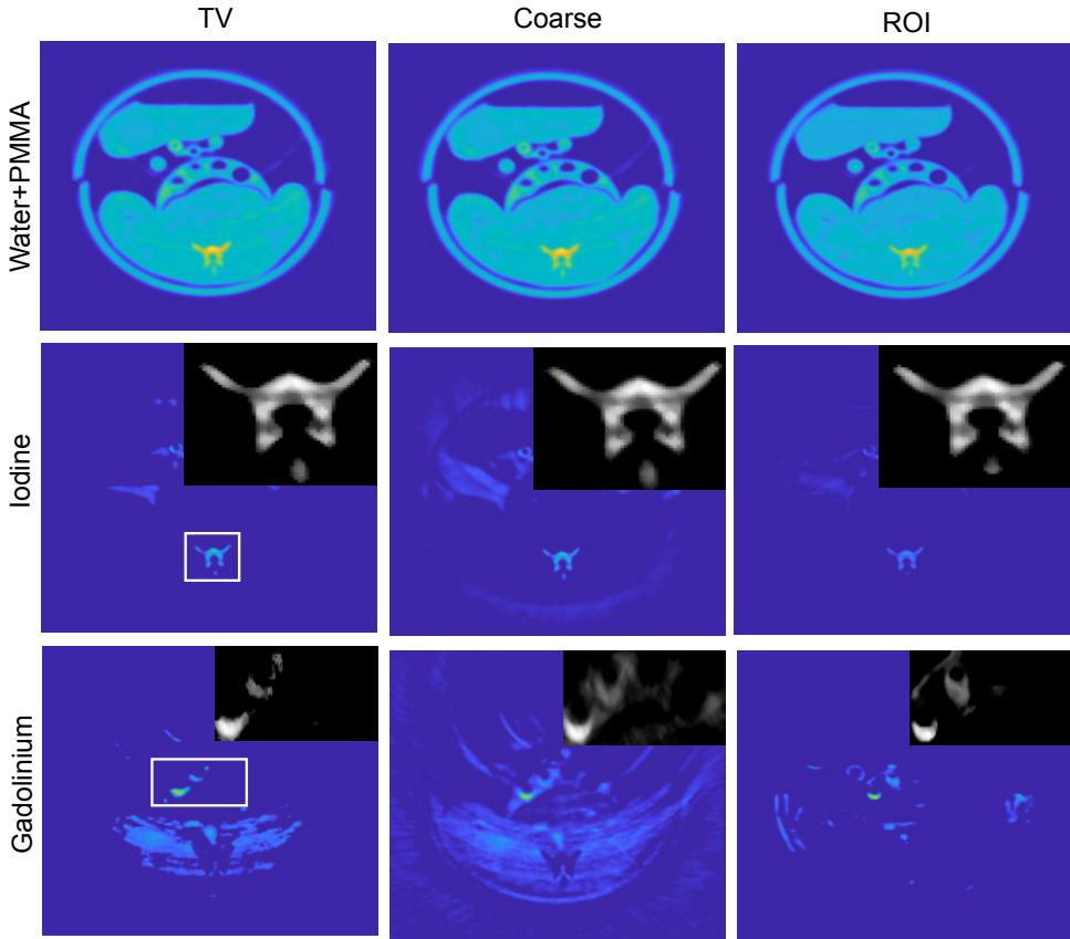
Figure 4.10: The results of material decomposition based on physical phantom. Left to right: Pseudo-inverse with TV, Coarse and ROI.
