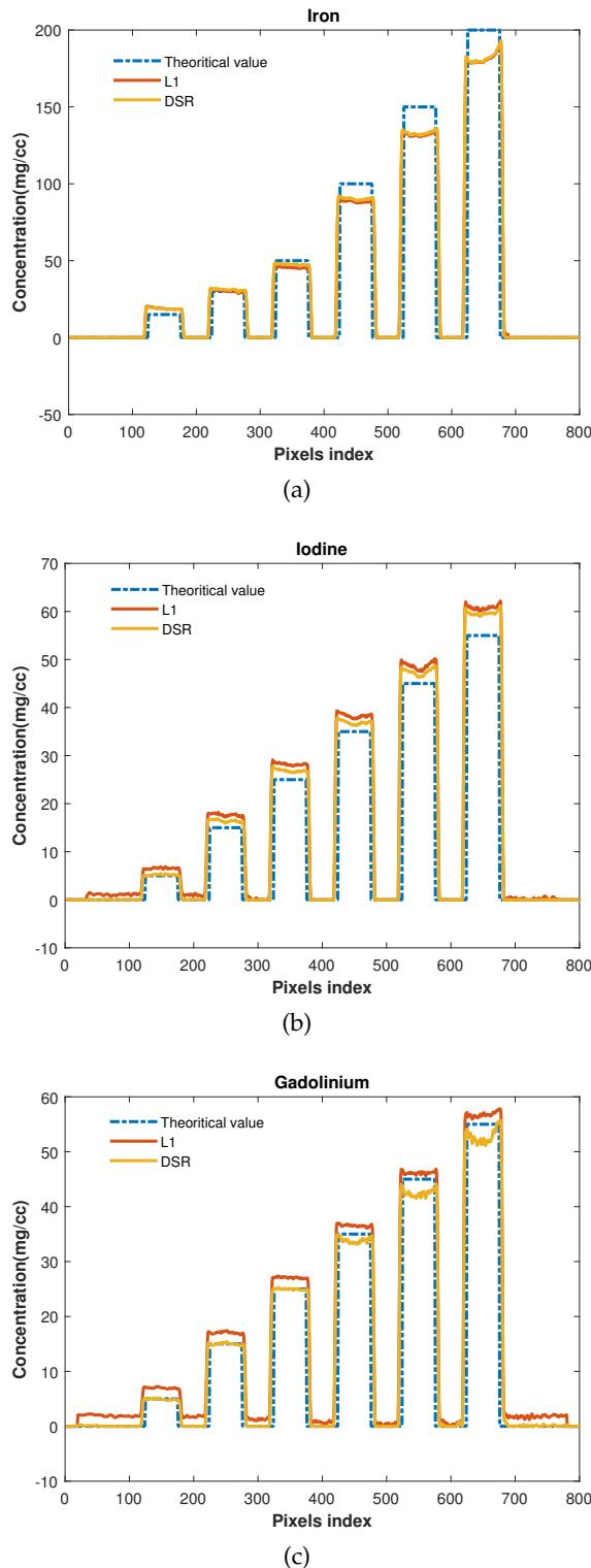
Figure 3.7: The mass densities of iron, iodine and gadolinium: 6 energy bins.
