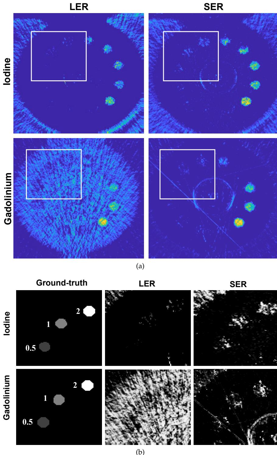
Figure 5.15: (a) The results of different material decomposition methods on physical phantoms in testing; (b) the ROIs in (a) for low-concentration materials. Labels in ROIs refer to the nominal concentration present in each tube (mg/cc).
