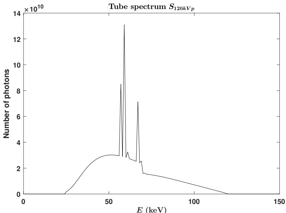
Figure 1.3: X-ray tube spectrum for the tube acceleration voltage  $U = 120$  kV. The spectrum is mainly composed of a broad quantum distribution caused by Bremsstrahlung in the x-ray tube anode material. The characteristic lines are due to inner electron shell transitions during a photoelectric effect event in the anode material atoms. Measured on Philips spectral CT prototype [Cormode et al., 2017, Si-Mohamed et al., 2018]
