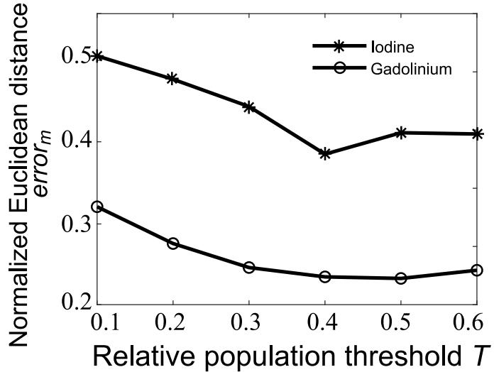
Figure 4.9: Influence of relative population threshold on the normalized Euclidean distance for iodine and gadolinium.
