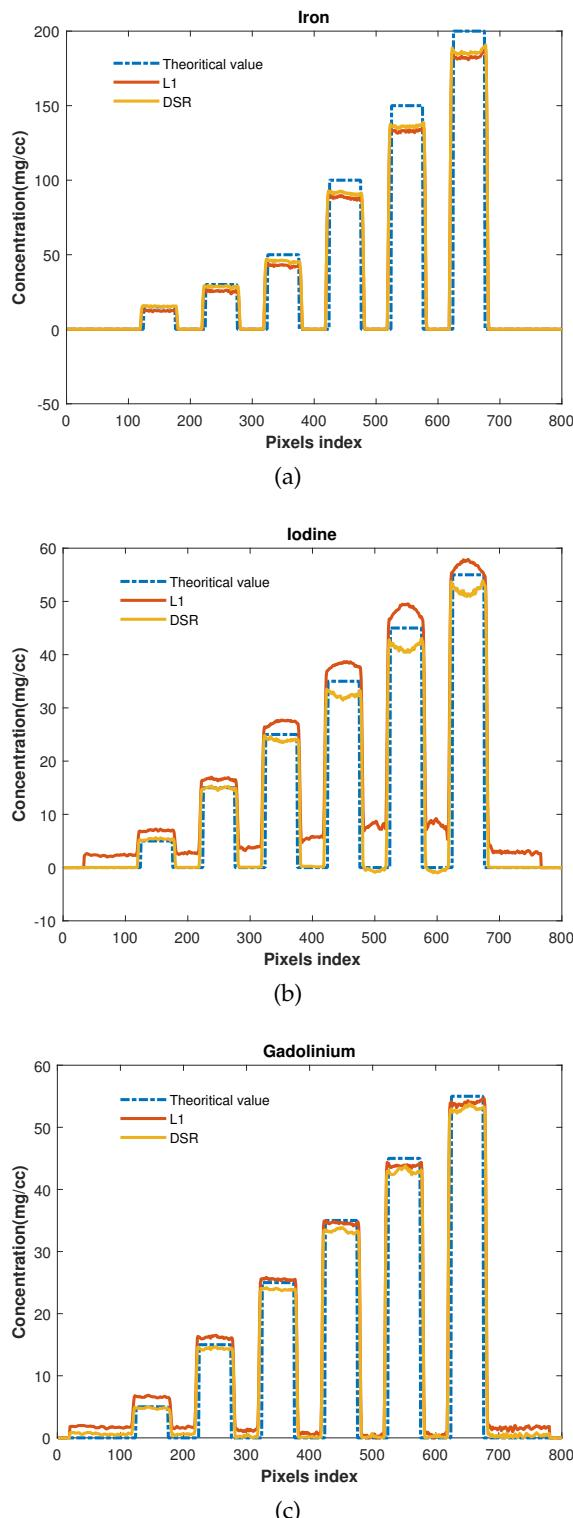
Figure 3.3: The mass densities of iron, iodine and gadolinium: 5 energy bins.
