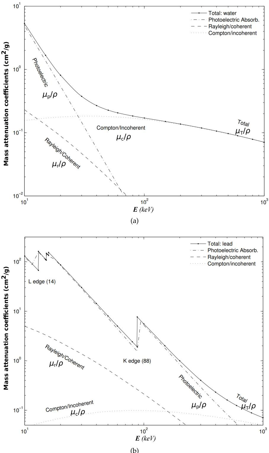
Figure 1.4: Total and components of mass attenuation coefficients of (a) water and (b) lead ( $\rho = 11.5 \text{ g/cm}^3$ ).
