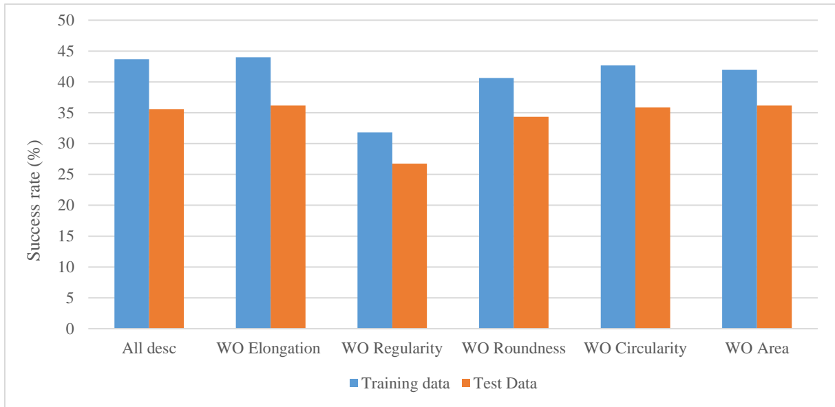
Figure V-6: Results of removing one descriptor from the morphological database using a logistic regression classifier.
