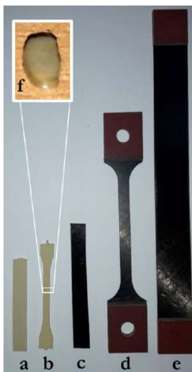
Fig. 2-5: Specimens employed for the experimental campaign
