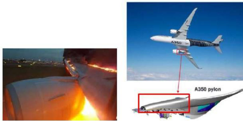
Fig. 1-1: Upper longeron of A350-1000 pylon, (Vinet et al. 2019)
