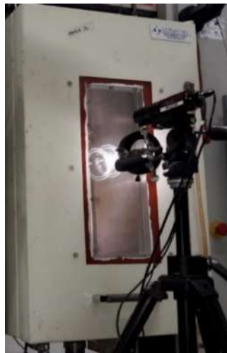
Fig. 2-25: Camera in front of the oven employed during high temperature tests.
