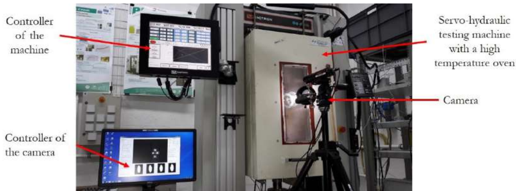
Fig. 2-6: Tensile, load-unload-reload and creep-recovery tests experimental equipment
