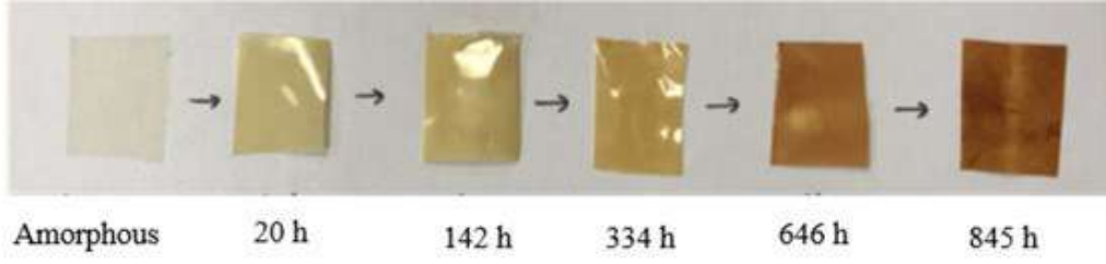
Fig. 1-13: PEKK 7002 AM film aged at 280°C on air (ENSAM Paris) (Roland and Fayolle 2020)
