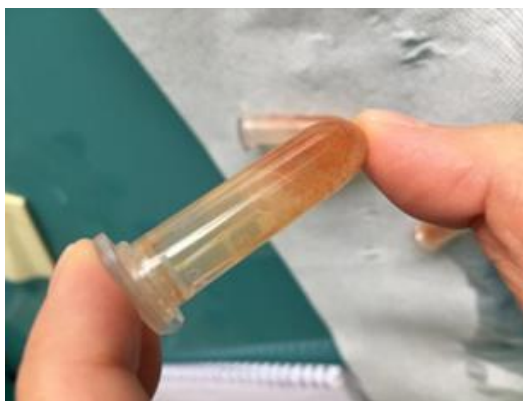
Fig. III-2-5 Commercial Aldehyde particles dispersed by probe sonication for 3 mins (1mg/mL in MQ water)
