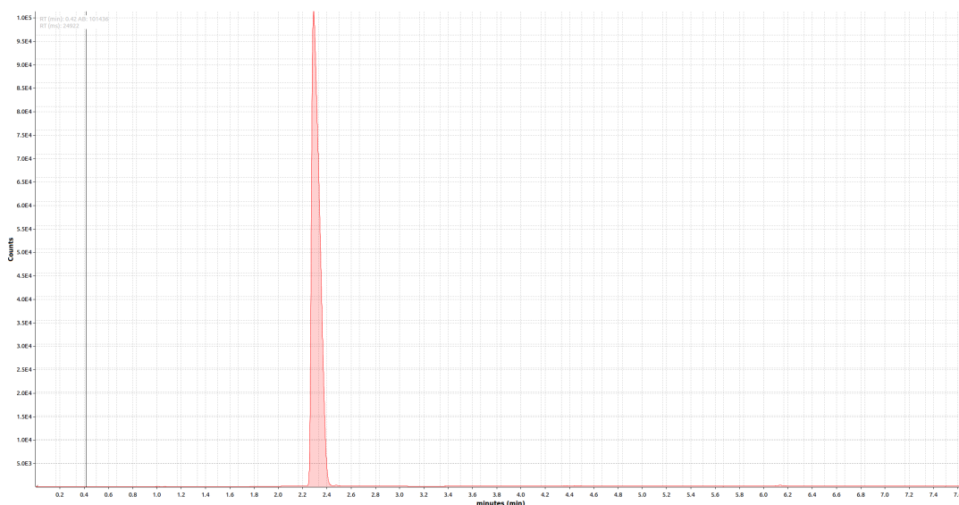
Figure 3.8: Permeate composition obtained using the membrane PERVAP 4510-2898
