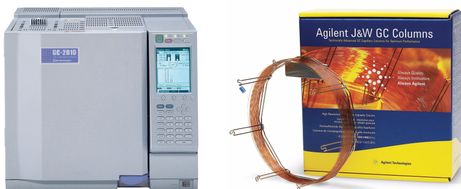
Figure 3.3: The GC device Shimadzu GC-2010 (left) and the column Agilent CP-Select 624 CB (right)
