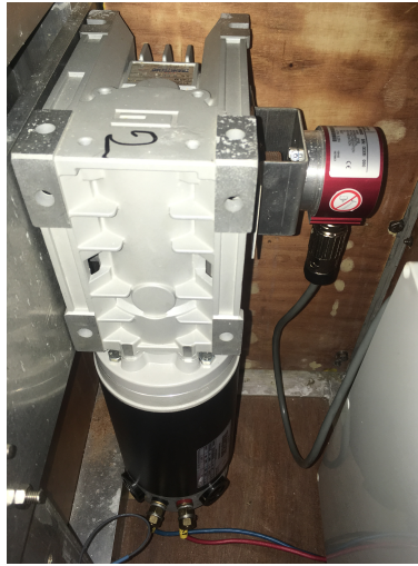
Figure 2.3.: Picture of one of the two gear-motors used for kite control, with the encoder measuring the actuator position (red device).
