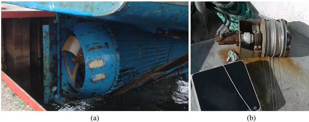
Figure 4.4.: Pictures of some specific parts of the boat. Picture (a) shows the propeller of the boat, and picture (b) shows the hydraulic winch for winding the four tethers of the kite. The two external tethers are the back ones, whereas the center tethers are the front ones, with bigger diameter.
