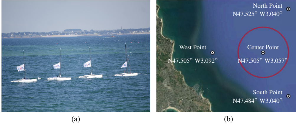
Figure 2.15.: Fixed wind measurement points deployed over the Bay of Quiberon. Picture (a) shows the 4 measurement platforms moored in front of ENVSN. Picture (b) is a GoogleEarth screenshot showing position of the 4 measurement points during trials (white circle); the central one is always occupied by the platform fitted with the 3-anemometer mast (the more on the right on picture (a)); the external locations are occupied by the other platforms fitted with the single-anemometer masts (picture (a), the first three from the right). The red circle shows the limit of the area of measurement (0.7nm radius).
