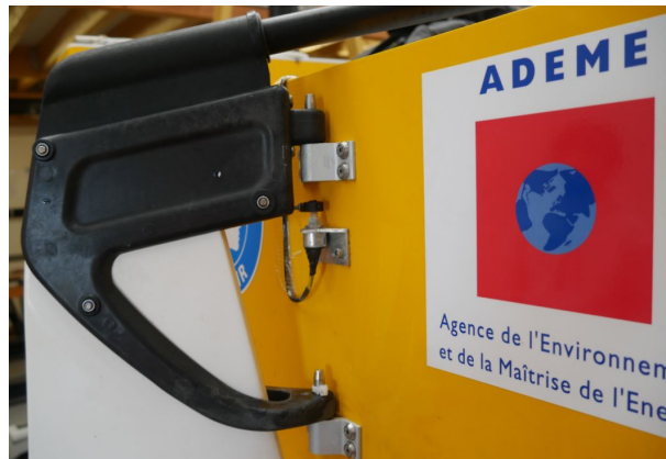
Figure 2.11.: Kiteboat’s steering system and rudder angle sensor
