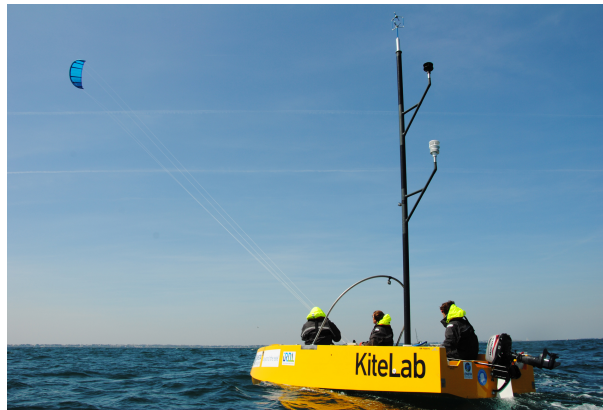
Figure 2.14.: Kiteboat's wind measurement experimental set-up based on three sonic anemometers located at different altitude above sea level.
