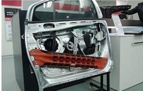
Figure G.4: The A51 side impact beam, as seen in the door structure of a Citroën C3 [G.13].
