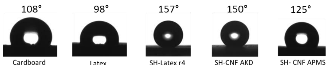
Figure 2. Water drop image on surfaces after 5 s and subsequent measurement of contact angle at the triple line.
