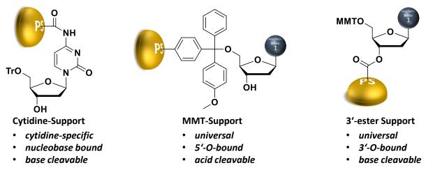
Figure I-13: First generation of solid supports for oligonucleotide synthesis.
