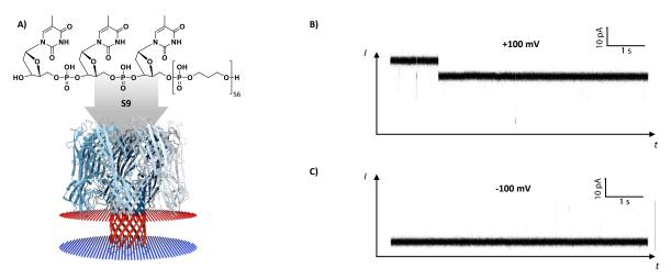
Figure V-5: Interaction between S9 and  $\alpha$ -hemolysin. A) visualization of sequence **S9** and pore; B) current histogram at positive voltage (+100 mV); C) current histogram at negative voltage (-100 mV).
