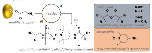
Scheme I-15: Synthesis of uniform information-containing oligo(alkoxyamine amide)s. amidification i): THF, HBTU, DIPEA, coding (AB) monomer; radical-radical coupling ii): CuBr, Me<sub>6</sub>TREN, DMSO, spacer (CD) monomer; cleavage from Wang support iii): TFA, DCM. Abbreviations: 2-(1H-benzotriazol-1-yl)-1,1,3,3-tetramethyluronium-hexafluorophosphat (HBTU), tris[2-(dimethylamino)ethyl]amine (Me<sub>6</sub>TREN).
