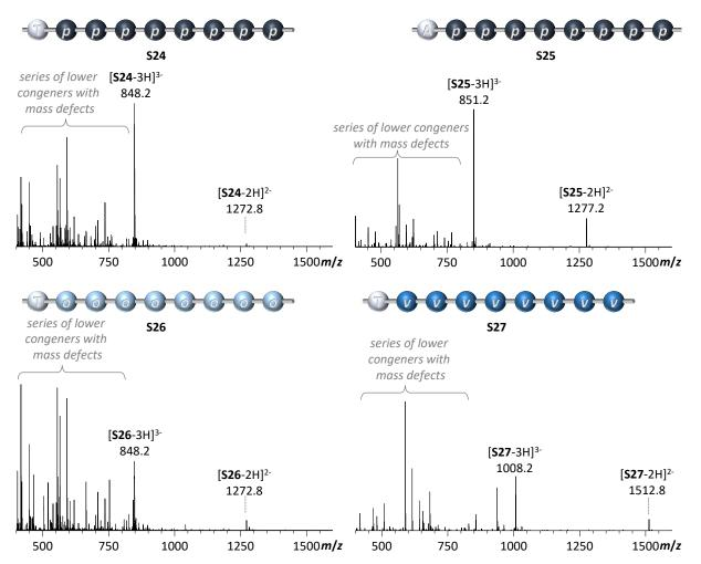
Figure IV-6: Attempted synthesis of test sequences **S24**, **S25**, **S26**, and **S27** using nitrobenzylated carbamate monomers **72**, **75**, and **78**. (ESI(-)-MS spectra shown in the m/z range 400 - 1600; range 100 - 400 cut for clarity: TCA contamination at 116.9, 160.9)
