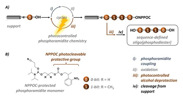
Figure III-1: Project design. A) photocontrolled phosphoramidite chemistry for synthesis of oligo(phosphodiester)s; B) coding phosphoramidite monomers protected with photolabile NPPOC group.
