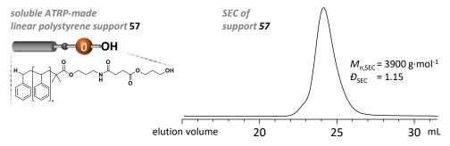
Figure III-3: SEC characterization of soluble ATRP-made linear polystyrene support  $\bf 57$  (SEC UV trace shown in the range of 15-31.5 mL).
