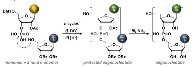
Scheme I-8: Oligonucleotide synthesis using the phosphodiester method.
