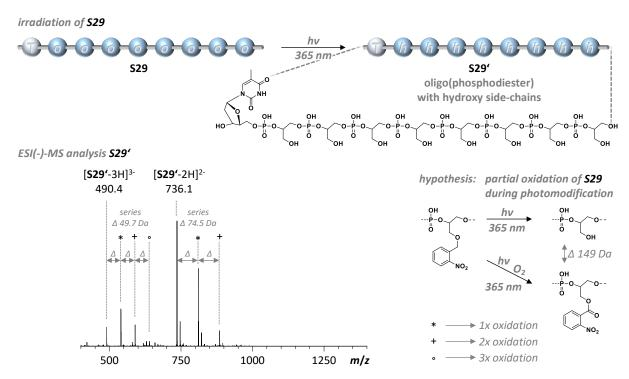
Figure IV-12: First photomodification of **S29** to **S29**'. (MS spectrum shown in m/z range 400 - 1400; side products detected at m/z = 540.0 (\*), 589.7 (+), 639.4 (·) as triply deprotonated species and m/z = 810.6 (\*), 885.1 (+) as double deprotonated species, respectively)
