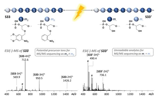
Figure IV-14: Erasing sequence information from sequence **S33** by quantitative photomodification to obtain unreadable sequence **S33'**. ESI(-)-MS spectra of **S33** and **S33'** shown in m/z range 400 - 1600.
