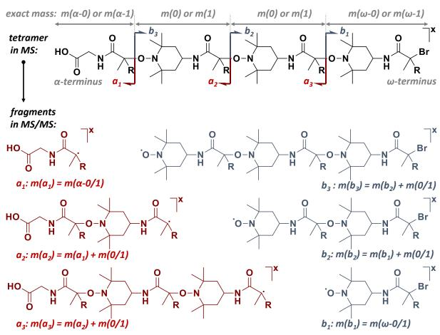
Figure I-16: Concept of MS/MS sequencing of linear macromolecules containing labile alkoxyamine bonds.
