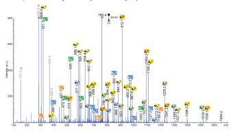
Figure V-20: MS/MS spectrum of the [ $\mathbf{S39'}$ -3H] $^3$ - ion at m/z 760.4.
