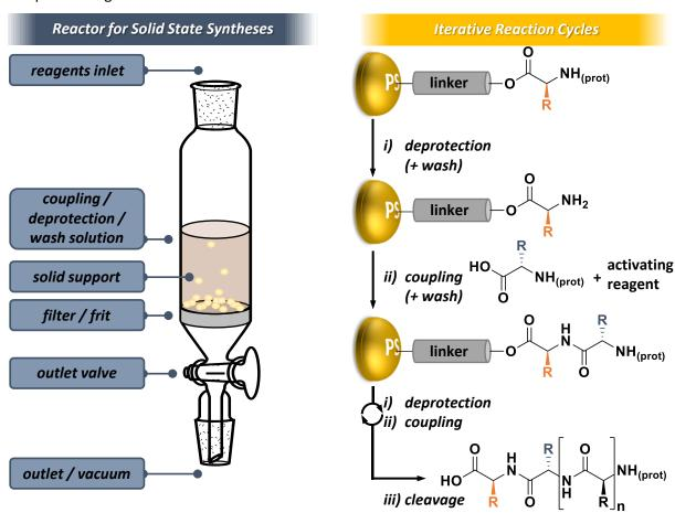
Figure I-3: Reactor for manual SPPS (left) and description of iterative reaction cycles on a solid polystyrene (PS) support (right).
