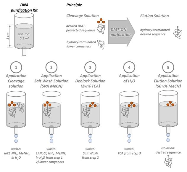
Figure V-1: Overview of DMT-ON purification.
