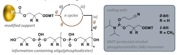
Scheme I-13: Manual synthesis of uniform information-containing oligo(phosphodiester)s. DMT-deprotection i): TCA, DCM; phosphoramidite coupling ii): MeCN, 1H-tetrazole, (AB) monomer; oxidation iii): THF, iodine, 2,6-lutidine, water; phosphate deprotection iv): MeCN, piperidine; cleavage from resin v): methylamine, ammonia.
