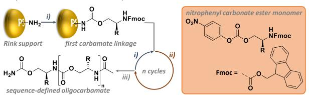
Scheme I-3: Early multistep-growth synthesis of sequence defined oligocarbamate by Schultz and coworkers. Carbamate coupling i): monomer, HOBt, diisopropylethylamine, N-methyl-2-pyrrolidon; deprotection ii): piperidine, N-methyl-2-pyrrolidon; cleavage from Rink resin iii) a. acetic anhydride, N-methyl-2-pyrrolidon, b. TFA, triethylsilane. Abbreviations: 2,2',2"-trifluoroacetic acid (TFA).
