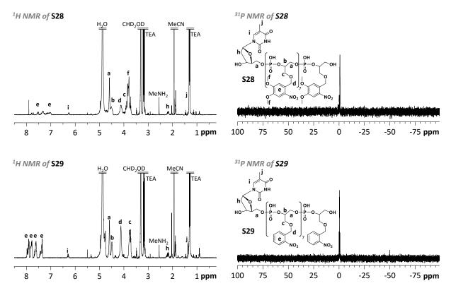
Figure IV-11:  $^{1}$ H NMR and  $^{31}$ P NMR spectra of sequences **S28** and **S29**, recorded in methanol- $^{4}$ , shown in the range of 8.5 to 0.0 ppm and 100 to -100 ppm, respectively.
