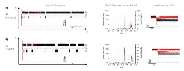
Figure V-7: Event analysis for \$9 with aerolysin at 120 mV. A) using 0.3 M KCl; B) using 1.0 M KCl.
