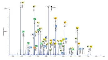
Figure V-17: MS/MS spectrum of the [ $\mathbf{S36'}$ - $\mathbf{3H}$ ]<sup>3-</sup> ion at m/z 625.4.
