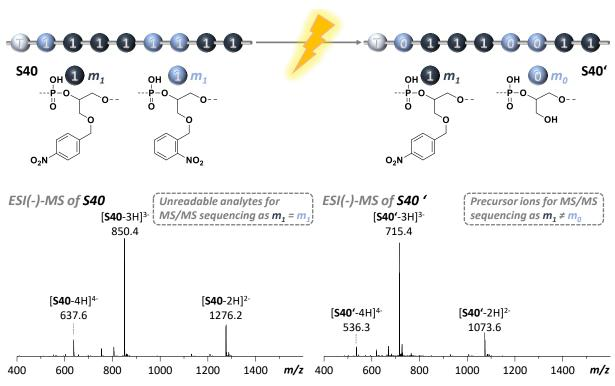
Figure IV-18: Revealing sequence information from sequence **S40** by chemoselective photomodification to obtain readable sequence **S40'**. ESI(-)-MS spectra of **S40** and **S40'** shown in m/z range 400 - 1600.
