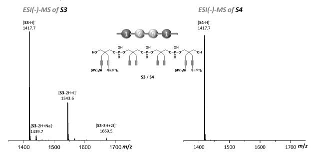
Figure II-7: Comparison of ESI(-)-HRMS for **S3** and **S4**. Negatively charged (-1) species are detected in the m/z 1350–1750 range.
