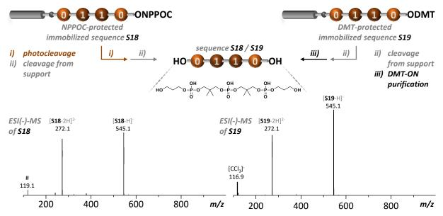
Figure III-6: Analysis by MS of identical sequences **\$18** (left) and **\$19** (right) synthesized from NPPOC and DMT precursors, respectively. (Spectra shown in the m/z range of 100-1000; denoted with #, the impurity is structurally not related to sequence **\$18**.)
