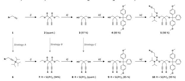
Scheme II-1: Synthesis of phosphoramidite monomers **5** and **10**: i) 1. THF, diethylmalonate, NaH, 0 °C; 2. (TIPS-protected) propargyl bromide; ii) THF, LiAlH<sub>4</sub>, -10 °C; iii) THF, pyr, DMTrCl; iv) DCM, DIPEA, 2-cyanoethyl-N,N-diisopropylchlorophosphoramidite, <0 °C. Strategies A, B, and C were investigated for insertion of the TIPS protective group and are detailed in Scheme II-2.
