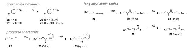
Scheme II-4: Overview Synthesis of further azides to allow diverse side chain tuning. Azide substitution xi): DMSO, NaN<sub>3</sub>, RT; amidification xii)  $K_2CO_3$ , bromoacetyl bromide, DCM, 0 °C; Bz-protection xiv) DIPEA, benzoic anhydride, DCM, 0 °C.
