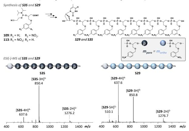
Figure IV-15: Synthesis of test sequences \$35\$ and \$29\$ using nitrobenzyl ether monomers \$109\$ and \$113\$. (ESI(-)-MS spectra shown in the m/z range 400-1600.)
