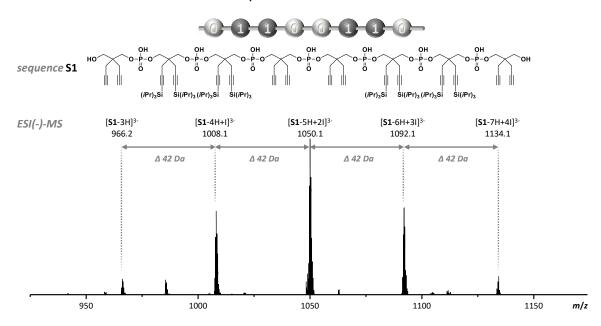
Figure II-6: ESI(-)-MS spectrum (the m/z 925 - 1175 range) recorded for the precursor sequence S1.
