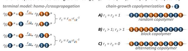
Figure I-10: Reactivity ratio-based copolymer sequence control. Non-exhaustive cases: A) no preference for homo- or crosspropagation; B) homopropagation favored; C) crosspropagation favored.
