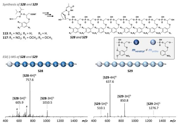
Figure IV-10: Synthesis of test sequences **S28** and **S29** using nitrobenzyl ether monomers **113** and **117**. Indicated with # are unknown contaminations. (ESI(-)-MS spectra shown in the m/z range 400 - 1600.)
