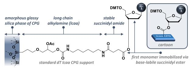
Figure I-14: Standard Icaa CPG support with immobilized deoxynucleotide.
