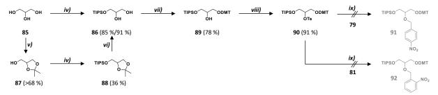
Scheme IV-5: Synthesis of a DMT-protected tosylate precursor **90** for nitrobenzylether formation by nucleophile insertion. TIPS protection iv): pyr, DCM, TIPS-Cl,  $0^{\circ}$ C; acetal formation v): toluene, reflux in Dean-Stark, pTsOH, acetone; acetal hydrolysis vi): AcOH (aq., 80 v%), DCM, 80 °C; DMT protection vii): pyr, THF, DMTrCl, RT; tosylate formation viii): pyr, pTsCl,  $0^{\circ}$ C; ether formation ix): various conditions.
