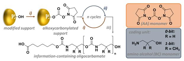
Scheme I-16: Synthesis of uniform information-containing oligocarbamates. alkoxycarbonylation i): MeCN,  $Et_3N$ , DSC (AA) monomer, microwave, 60 °C; carbamate formation ii): DMF,  $Et_3N$ , coding (BC) monomer; cleavage from modified Wang support iii): TFA, DCM. Abbreviations: N,N'-disuccinimidyl carbonate (DSC), triethylamine ( $Et_3N$ )
