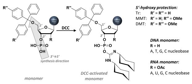
Scheme I-7: Monomer activation with DCC for phosphodiester method.
