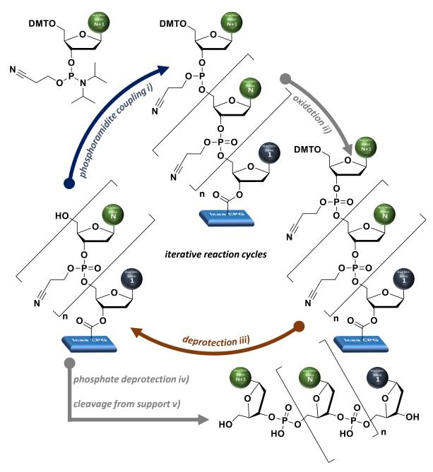
Scheme I-12: Phosphoramidite Chemistry. Iterative reaction cycle comprises phosphoramidite coupling i): MeCN, phosphoramidite monomer, 1H-tetrazole; oxidation ii): THF, iodine, water, 2,6-lutidine; deprotection iii): TCA, DCM. Desired sequence attained after phosphate deprotection (and nucleobase deprotection) iv): MeCN, piperidine; and cleavage from support v): (methylamine) ammonia.
