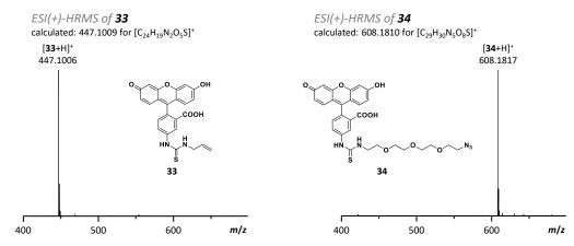
Figure II-3: ESI(+)-HRMS of 33 (left) and 34 (right) shown in the m/z 400-700 range.
