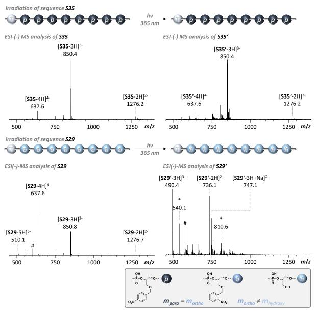
Figure IV-17: Photomodifiation test of sequences  $\bf S35$  and  $\bf S29$ . (ESI(-)-MS spectra shown in the m/z range  $\bf 450-1400$ .)
