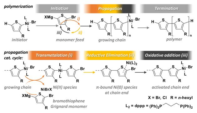
Scheme I-2: Catalytic cycle of a Kumada-Tamao catalyst-transfer condensation polymerization of a Grignard monomer. Abbreviation ligand  $L_2$ : 1,3-bis(diphenylphosphino)propane (dppp).
