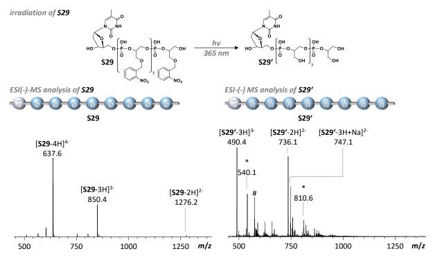
Figure IV-13: Photomodification of **S29** to **S29'**. MS spectra of **S29** and **S29'** shown in m/z range 450 - 1400; oxidation side product \* detected at m/z = 540.1 as triply deprotonated species and m/z = 810.6 as double deprotonated species, respectively.
