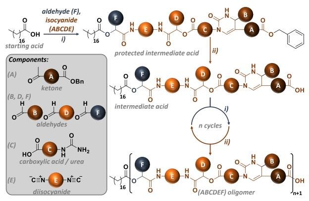
Scheme I-18: Synthesis of information-containing macromolecules from several multi-component reactions. Passerini three-component reaction i): carboxylic acid (intermediate or starting), aldehyde (F), (ABCDE) isocyanate macromonomer, DCM, rt, 3 d; benzyl deprotection ii):  $H_2$ , Pd/C, EtOAc (or THF) rt, 24 h.
