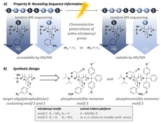
Figure IV-2: Conceptual design to reveal molecularly encoded information. A) Property B: revealing information in digital polymers using light; B) Design of oligo(phosphodiester)s and respective phosphoramidite monomers.
