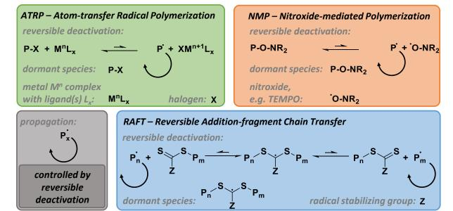
Figure I-11: Mechanisms of controlled/living polymerizations or reversible-deactivation polymerizations. A type of metal-catalyzed ATRP is shown.
