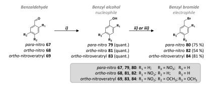
Scheme IV-4: Synthesis of nucleophiles **79**, **81**, and **83** and electrophiles **80**, **82**, and **84** for nitrobenzylation reactions. Aldehyde reduction i): MeOH, DCM, NaBH<sub>4</sub>, RT; bromination for **80** and **82** ii): THF, PBr<sub>3</sub>,  $0^{\circ}$ C; Appellike reaction for **84** iii): THF, CBr<sub>4</sub>, PPh<sub>3</sub>,  $0^{\circ}$ C.
