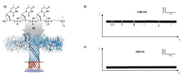
Figure V-6: Interaction between **S9** and aerolysin. A) visualization of sequence **S9** and pore; B) current histogram at positive voltage (+100 mV); C) current histogram at negative voltage (-100 mV).
