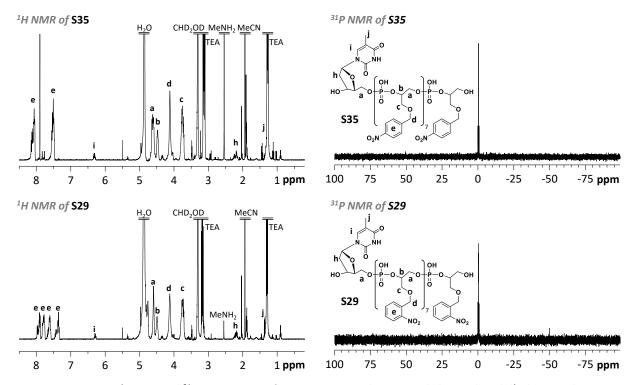
Figure IV-16:  $^1$ H NMR and  $^{31}$ P NMR spectra of sequences **\$35** and **\$29**, recorded in methanol- $d^4$ , shown in the range of 8.5 to 0.0 ppm and 100 to -100 ppm, respectively.
