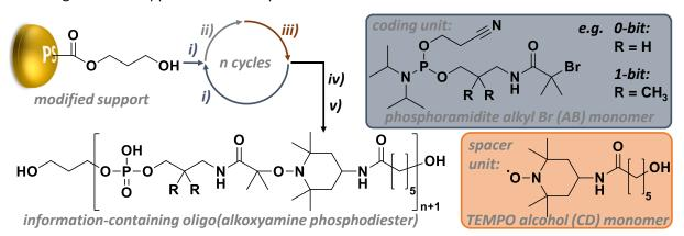
Scheme I-17: Synthesis of uniform information-containing oligo(alkoxyamine phosphodiester)s. phosphoramidite coupling i): MeCN, 1H-tetrazole, (AB) monomer; oxidation ii): THF, iodine, 2,6-lutidine, water; radical-radical coupling iii): DMSO, CuBr, Me<sub>6</sub>TREN, (CD) monomer; phosphate deprotection iv): MeCN, piperidine; cleavage from resin v): methylamine, ammonia.
