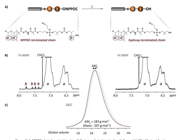
Figure III-4: NPPOC photodeprotection step. A) Cartoon; photodeprotection i):  $2 \text{ mg} \cdot \text{mL}^{-1}$ , 50 mM piperidine in CHCl<sub>3</sub>,  $\lambda = 365 \text{ nm}$ , 120 min; B)  $^1\text{H}$  NMR (zoom of the aromatic region 6.1 - 8.0 ppm) of NPPOC (left)- and hydroxy-terminated chains (right); C) SEC UV traces of NPPOC (black)- and hydroxy-terminated (red, dotted) chains.
