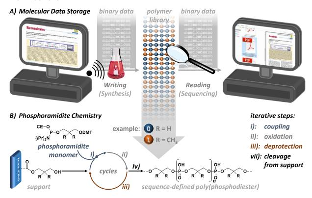
Figure 1: A) Data storage on the molecular level by writing binary information on polymers and reading them. B) Phosphoramidite chemistry to obtain information-containing poly(phosphodiester)s (shown: binary code).
