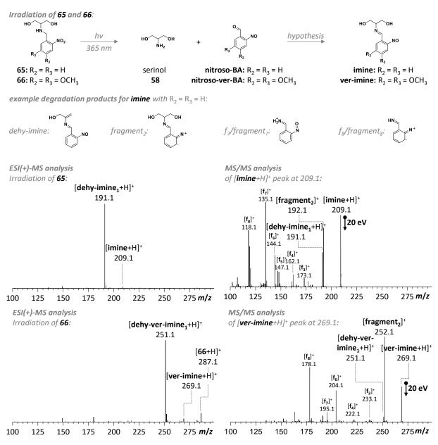
Figure IV-7: Photoinduced cleavage of nitrobenzylamines **65** and **66** and (tandem) MS analysis of reaction products.
