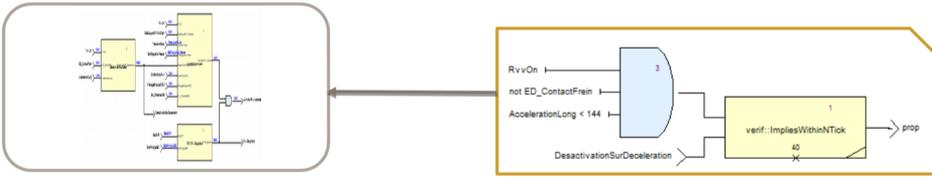
Figure 21: Property  $PI_{40}$  expressed on an isolated sub-node
