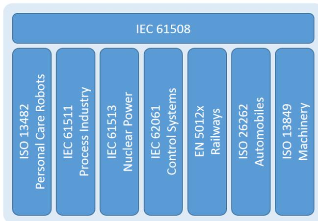
Figure 7: Derivation of safety standards from IEC 61508
