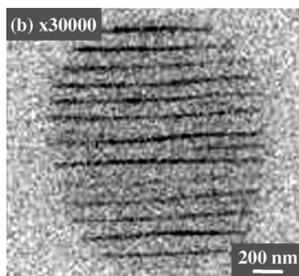
Figure 2.6: Example of a nanostructured silica glass. Here is shown a SEM image taken from [67], where the authors present ‘fingerprints’ left in the sample after direct femtosecond laser writing process.
