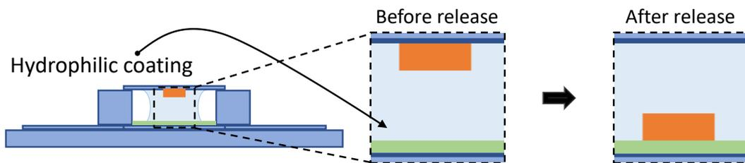
Figure 3.17: *Experimental arrangement dedicated to the optical manipulation of spinners. When the spinner lands on the hydrophilic coated substrate after optical release, it is ready to be manipulated.*
