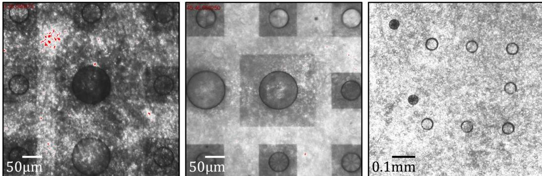
Figure 3.14: *Collection of 25 spinners on their original substrate as received: 21 with a  $50\mu\text{m}$  diameter and 4 with  $100\mu\text{m}$  diameter.*
