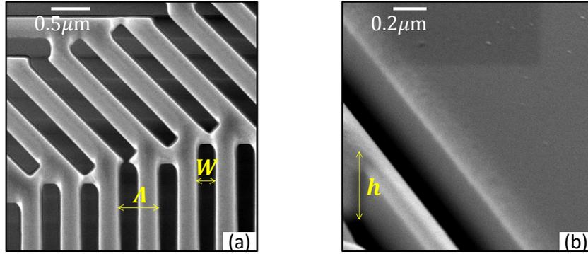
Figure 3.2: Scanning electron microscopy images illustrating the fabricated dielectric space-variant birefringent pattern on a silicon-nitride membrane. (a)  $\Lambda$  and  $W$  correspond to the grating period and the slit width, respectively. (b)  $h$  corresponds to the membrane thickness.
