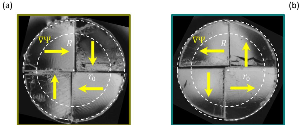
Figure 2.20: Two samples with opposite spatial distribution of the orientational gradients  $\nabla\psi$ , and radius  $R = 3$  mm are prepared to ensure either (a) left-handed or (b) right-handed effects.
