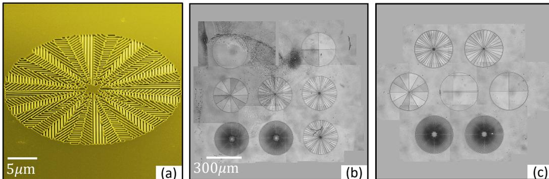
Figure 3.12: *The first batch of nanostructured geometric phase plates fabricated from a diamond membrane. (a) Scanning electron micrograph of an optical vortex generator for  $\ell = 10$ . Extension to any other wavelength is easily achieved by design, adapting the grating pitch, depth and filling factor to the need. (b,c) Bright field optical images of the two nanostructured membranes with 5  $\mu\text{m}$  thickness, whose elements are not yet cut in their periphery.*
