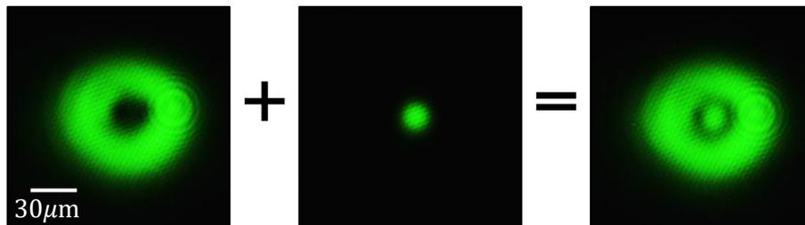
Figure 3.10: *Superposition of two incoherent beams: a doughnut one (radially polarized) and Gaussian one (circularly polarized). Two independent lasers at 532 nm wavelength are used, preventing from interference between the trapping and the manipulating fields*
