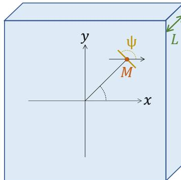
Figure 1.11: Diagram of a plate made of locally-uniaxial birefringent material of thickness  $L$ . Orientation of the optical axis in the plane of the plate is defined at the point  $M$  by the angle  $\psi$ .
