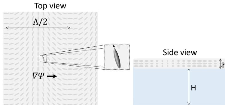
Figure 2.11: Cycloidal birefringent grating patterned on a polymer liquid crystal layer lying on a soft plastic substrate. The polymer liquid crystal layer thickness is  $h \sim 2\mu\text{m}$ , that corresponds to  $\Delta \simeq \pi$  at  $\lambda = 532 \text{ nm}$ ; the soft plastic substrate thickness is  $H \sim 200\mu\text{m}$ .
