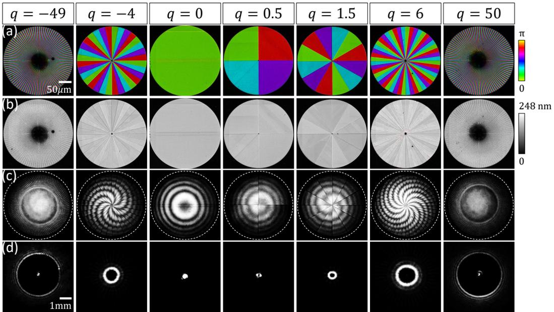
Figure 3.13: *Structural (a,b) and optical (c,d) characterization of the first batch of diamond elements. (a) Slow axis orientation maps, see orientation angle color bar at the end of the row. (b) Maps of birefringent phase retardation in gray scale, from 0 to 248 nm, see color bar at the end of the row. (c) Interference patterns between a test beam and the vortex generated by each structure in its plane for incident circular polarization. (d) Far-field image of the generated vortex.*
