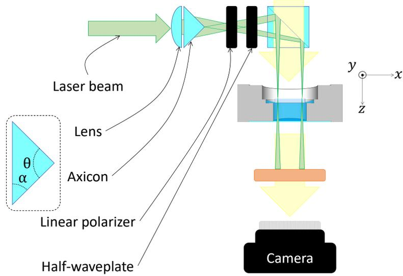
Figure 2.18: A secondary line is added to the arrangement depicted in Fig.2.5(c). The use of a lens followed by an axicon, combined with the use of a linear polarizer and a half-waveplate, allow generating a circular polarized ring-shaped illumination.
