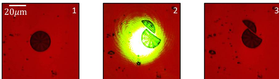
Figure 3.7: *Example of a failed attempt to transfer a spinner between substrates, where you wanted to focus on a new substrate after being released and collected from its original substrate, in the end, it breaks. After several tests with this spinner, it was determined that the safe beam power is  $< 100$  mW, with a beam of diameter  $\sim 30$   $\mu\text{m}$ .*
