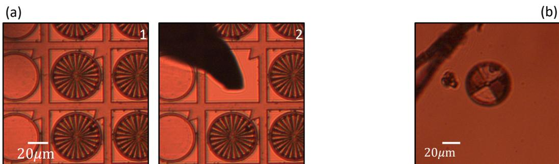
Figure 4.2: (a) *Sequence of image illustrating the micro-poking strategy: (1) initial array, (2) just after poke, the shadow of the micro-needle can be seen. (b) Image of a poked spinner that has landed on air/water interface place underneath the array.*
