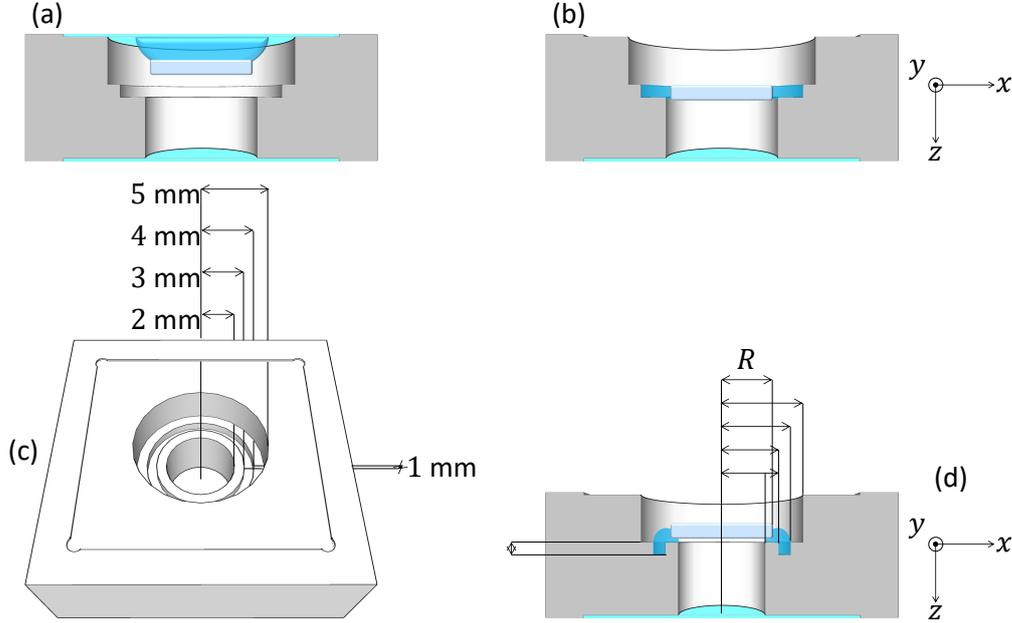
Figure 2.10: *Alternative systems tested for the left-handed torque experimental realization in order to reduce the viscous torque. (a) A liquid droplet is placed at a cover-slip to hold the disk by capillarity. (b,d) The sample is held by a ring of water sealing an air chamber created in between a cover-slip at the bottom of the pool, the pool, and the disk itself. (c) New pool designed with a trench milled at the middle step for the system (d).*
