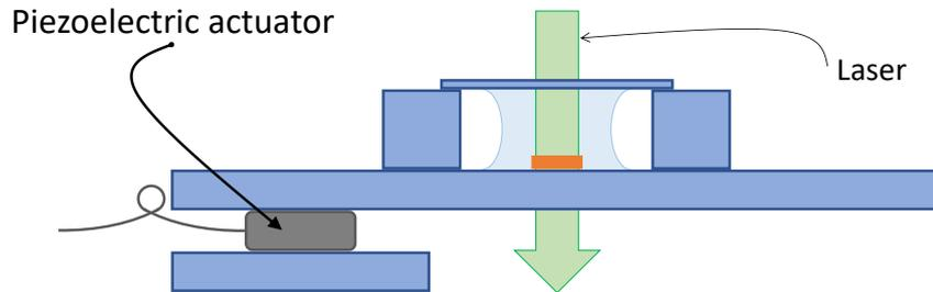
Figure 4.1: *Sketch of the experimental approach aiming at creating mechanical vibration of the substrate on which sits the micro-optical element to be manipulated in order to facilitate its ability to rotate under the action of light.*
