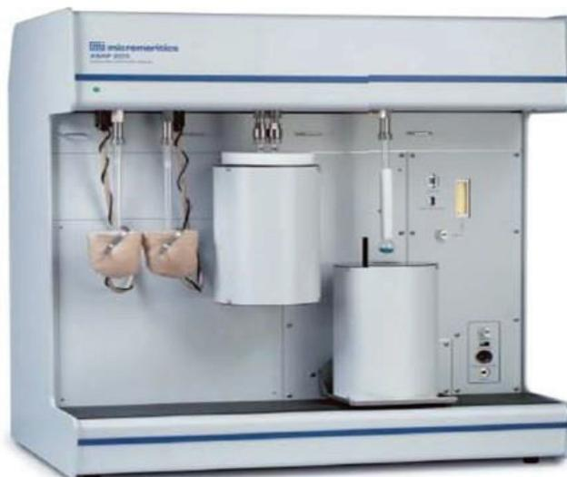
Figure 3-5 – Picture of Micrometrics ASAP 2020
