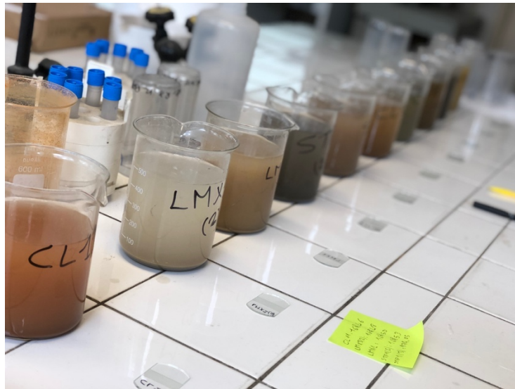
Figure 2.41: Decantation of the samples during the dilution step, the last step before preparing aggregate clay slides.
