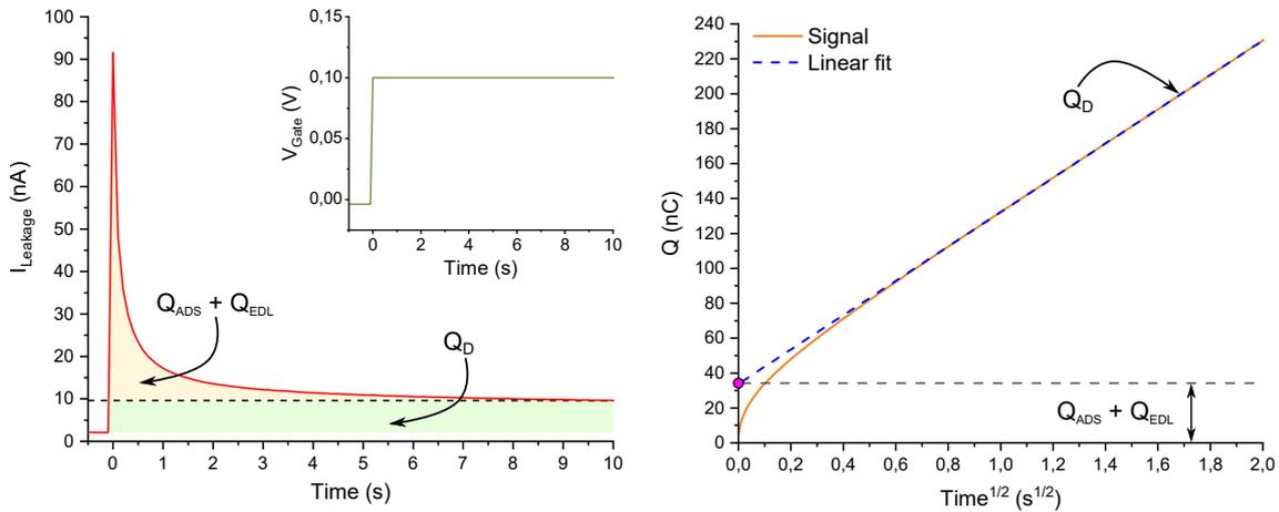
Figure 4.7: (left) Leakage current response (in red) when applying a potential step (inset) in  $0.1 \text{ mol.L}^{-1}$  NaCl electrolyte. The different contributions are highlighted from (right) the total charge generated during the interval, plotted as a function of  $\sqrt{t}$ .
