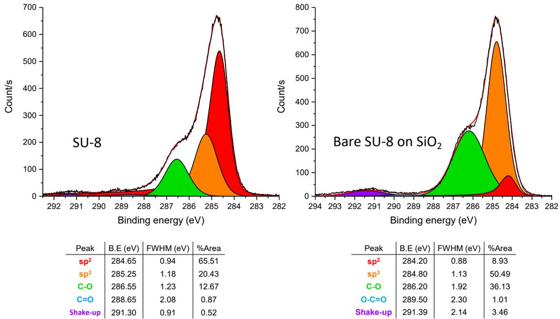
Figure 3.12: High-resolution C1s spectra after SU-8 passivation, and on the surface of bare SU-8 on SiO<sub>2</sub> with the different contributions.
