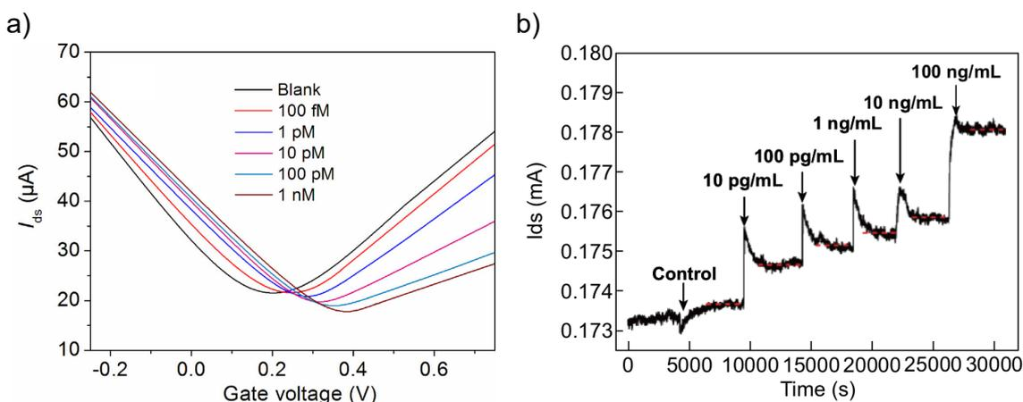
Figure 1.26: Examples of monitoring a) DNA hybridization through  $V_{\text{Dirac}}$  variations (from [185]), or cancer protein biomarker binding as a function of time at a working gate potential (from [186]).
