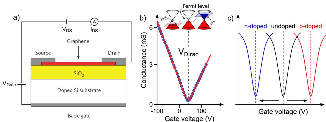
Figure 1.16: a) Graphene-based back-gated FET (from [148]), b) the associated typical transfer curve showing the ambipolar characteristic due to the peculiar charge injection by electrostatic gating (data from [120]) and c) the effect of doping on the Dirac point of the transfer curve.
