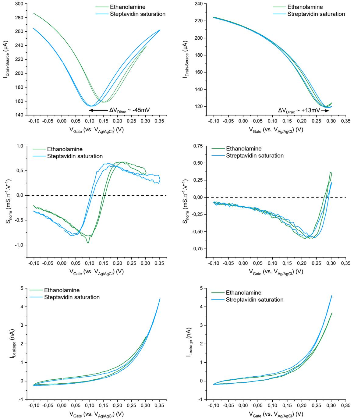
Figure 5.7: Transfer curves, normalized electrical sensitivity and leakage current curves of SGFET before (green) and after (blue) the sensor saturation with streptavidin of tripod (left) and PBASE (right) functionalized SGFET.
