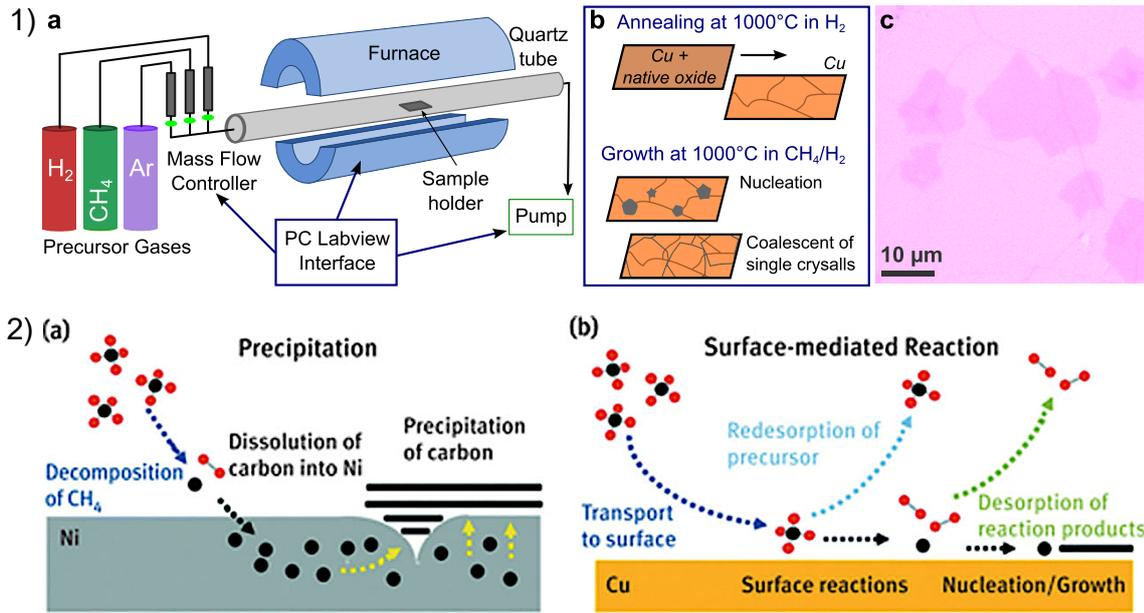
Figure 1.14: 1) a) Typical experimental setup for the CVD growth of graphene, b) Schematic representation of the growth principle and c) Optical picture of graphene (transferred on a Si/SiO<sub>2</sub> substrate after growth) showing the multilayer patches (from [137]), 2) a) Surface segregation mechanism and b) Surface adsorption process (from [138]).
