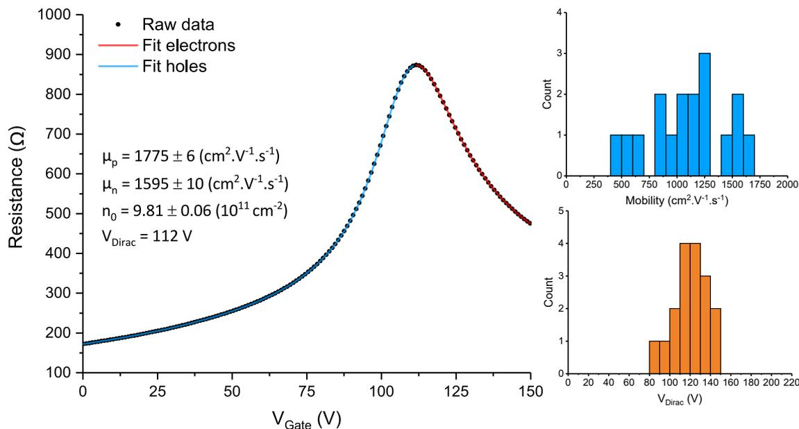
Figure 4.1: Transfer curve of a  $250\text{ }\mu\text{m} \times 50\text{ }\mu\text{m}$  device before SU-8 passivation (left), with typical hole mobility (upper right) and  $V_{\text{Dirac}}$  potential values (lower right) obtained with our process.
