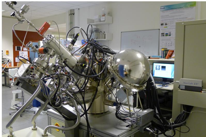
Figure 13: PHI 5000 Versa Probe II XPS spectrometer.
