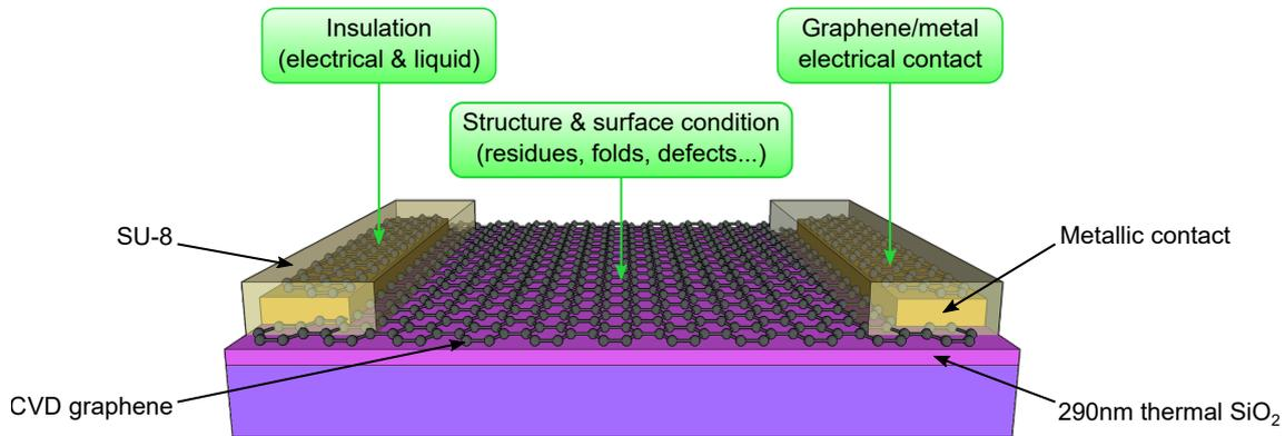
Figure 2.1: Requirements specification for the fabrication of SGFET devices.
