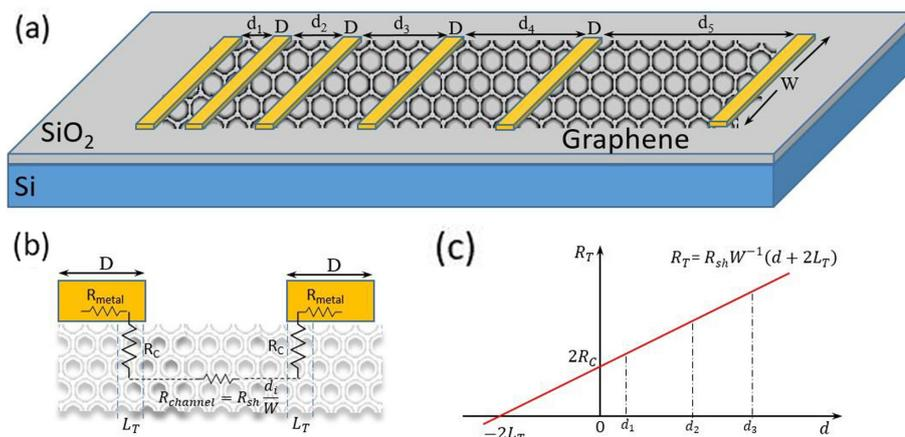
Figure 1.17: a) Device architecture for TLM measurement, b) the equivalent electrical model and c) the resulting linear behaviour of the total resistance as a function of channel length for extracting  $R_s$ ,  $R_c$  and  $L_t$  (from [155]).
