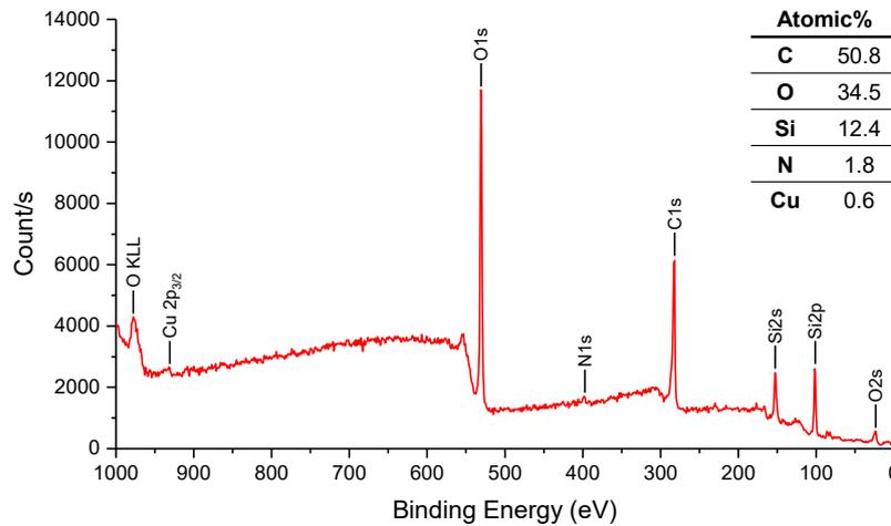
Figure 3.9: Survey spectrum of the pattern Cu sample, showing the presence of the Cu element and the relative atomic composition.
