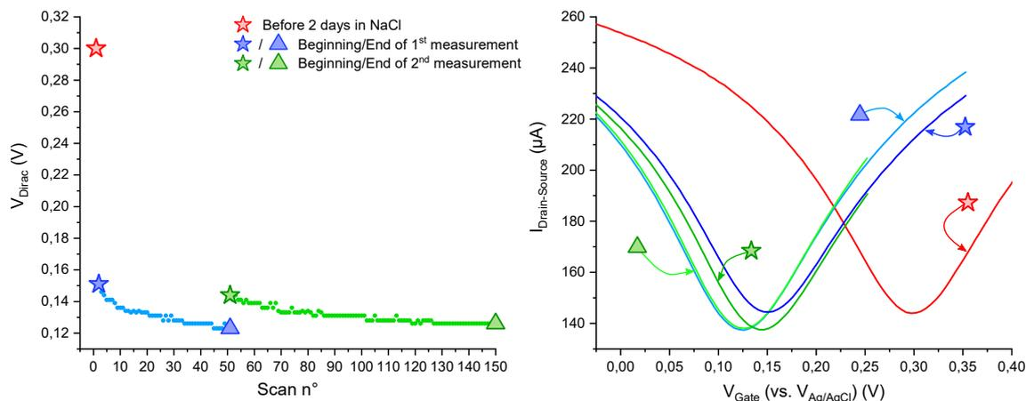
Figure 4.16: (left)  $V_{Dirac}$  slow drift between consecutive measurements, after 2 days in NaCl, and (right) the corresponding transfer curves (see symbols on the left figure).  $V_{DS}$  was set to 0.1 V, the gate potential was swept at a scan rate of  $10 \text{ mV} \cdot \text{s}^{-1}$  in  $0.1 \text{ mol} \cdot \text{L}^{-1}$  NaCl electrolyte.
