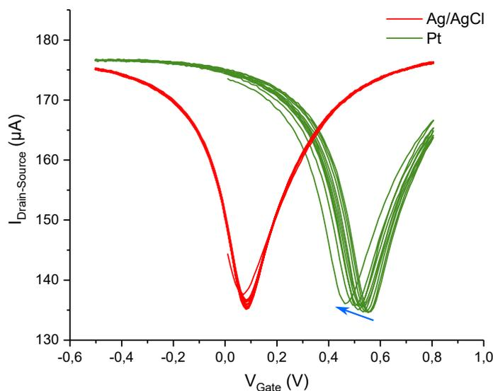
Figure 4.4: Stability comparison between Ag/AgCl and Pt gate electrode for SGFET measurements.  $V_{\text{DS}}$  was set to  $0.1\ \text{V}$ , the gate potential was swept 5 times between  $-0.5$  and  $0.8\ \text{V}$ , at a scan rate of  $50\ \text{mV.s}^{-1}$  in  $0.1\ \text{mol.L}^{-1}$  NaCl electrolyte.
