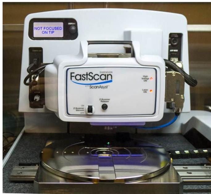
Figure 12: AFM Dimension FastScan scanner (Bruker).
