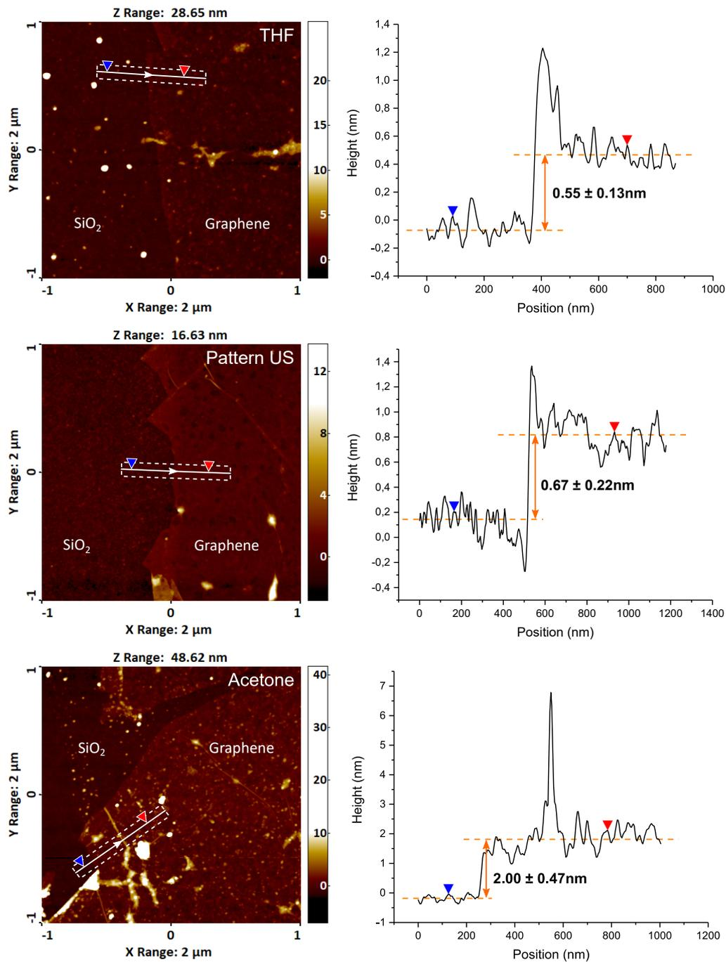
Figure 3.2: 2 μm × 2 μm scan (left) at the graphene/SiO<sub>2</sub> interface and the associated step height (right) after acetone and THF cleaning and graphene lift-off. Colormaps are harmonized (white spots are higher than 10nm).
