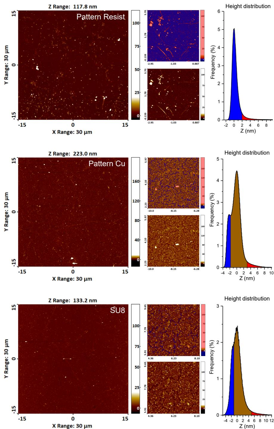
Figure 3.5:  $30\ \mu\text{m} \times 30\ \mu\text{m}$  2D maps of the graphene surface (left), raw zoomed view (middle-bottom) and colorized (middle-top) with the associated height distribution (right) after graphene patterning and passivation.
