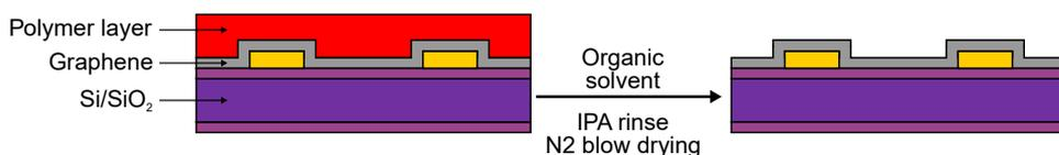
Figure 2.12: PMMA stripping step in organic solvent.
