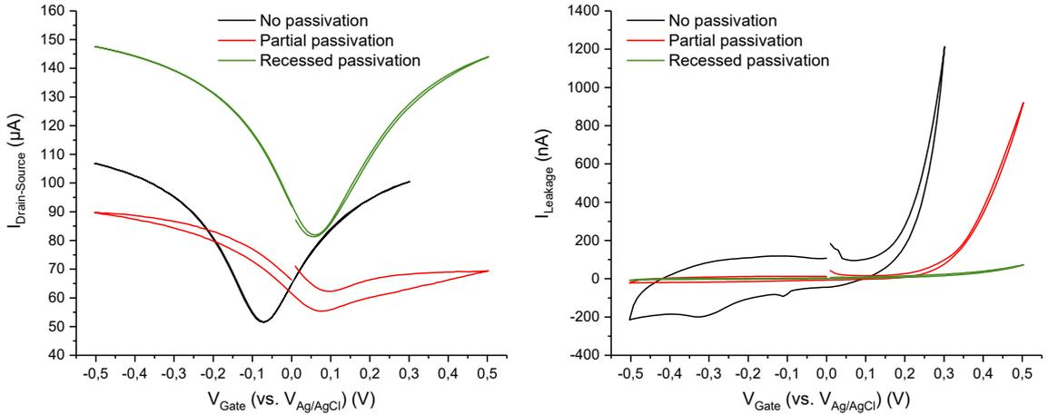
Figure 4.5: Comparison of devices not passivated (black), passivated with the "partial passivation" design (red) and "Recessed passivation" design (green) through drain-source (left) and leakage (right) I-V curves.  $V_{\text{DS}}$  was set to  $0.1\ \text{V}$ , the gate potential was swept at a scan rate of  $50\ \text{mV.s}^{-1}$  in  $0.1\ \text{mol.L}^{-1}$  NaCl electrolyte.
