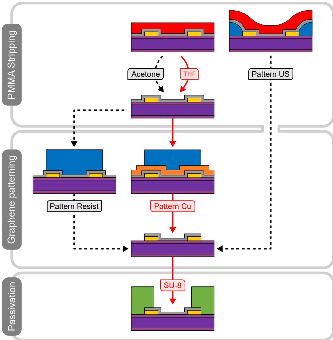
Figure 2.33: Recap of different fabrication methods tested and developed. Red arrows indicate the "main" process, dashed arrows indicate "variants" for a given step of the fabrication process (for example: the "Pattern Resist" sample corresponds to the patterning of graphene with a resist etching mask, with the PMMA stripped in THF at the previous fabrication step).
