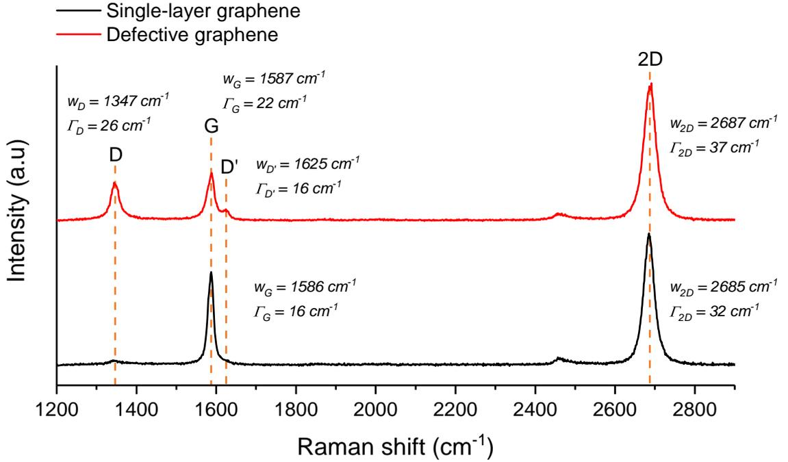
Figure 3.14: Raman spectra of typical graphene single-layer transferred onto SiO<sub>2</sub> substrate, and defective graphene.
