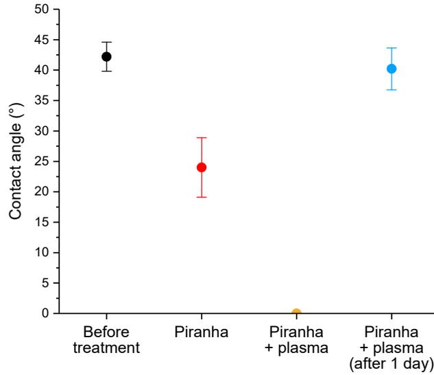
Figure 2.9: Combined effect of the "Piranha" cleaning with the plasma surface treatment on the contact angle of water with the surface of Si/SiO<sub>2</sub> single chips. Each point represents 5 measurements.
