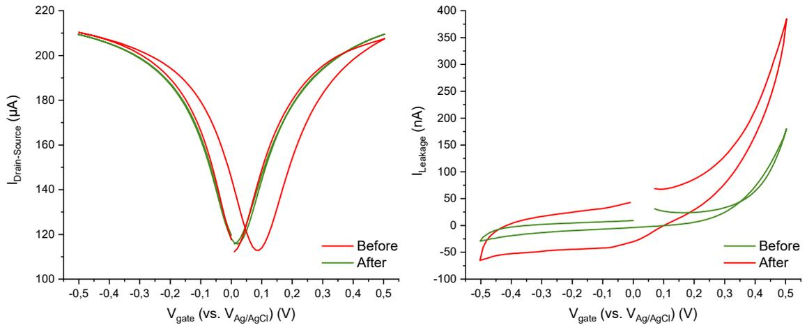
Figure 4.9: Transfer curves (left) and leakage current (right) before (green) and after (red) scanning the gate potential up to 1 V.  $V_{\text{DS}}$  was set to 0.1 V, the gate potential was swept between  $-0.5$  and  $0.5$  V, at a scan rate of  $10 \text{ mV}\cdot\text{s}^{-1}$  in  $0.1 \text{ mol}\cdot\text{L}^{-1}$  NaCl electrolyte.
