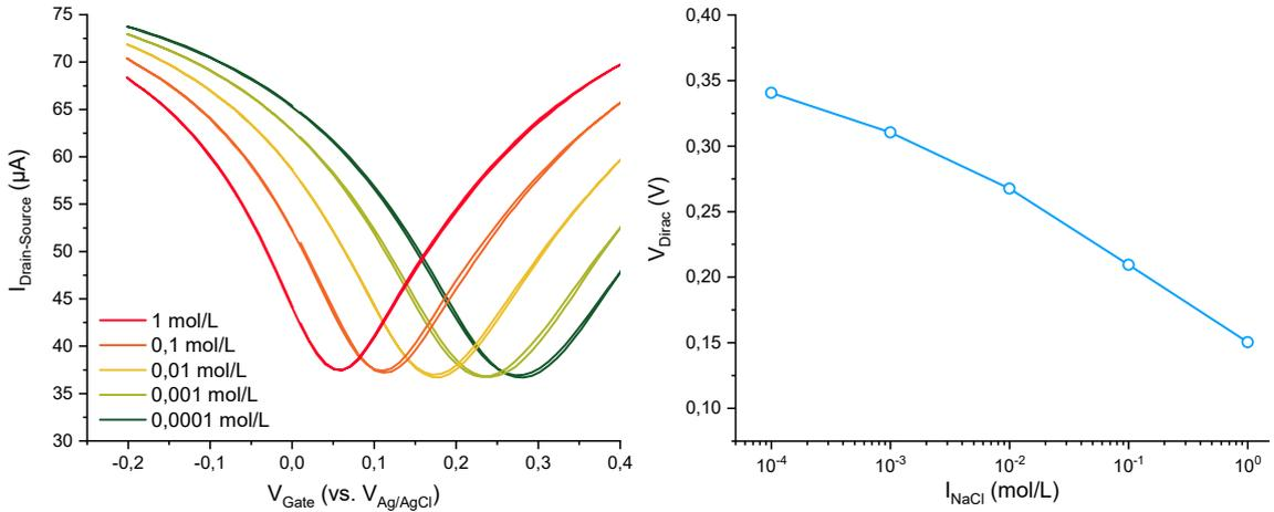
Figure 4.17: Influence of the ionic strength of a NaCl solution, shifting the transistor curves (left) and  $V_{Dirac}$  (right) (mean value extracted from 5 devices).  $V_{DS}$  was set to  $0.1 \text{ V}$ , the gate potential was swept between  $-0.2$  and  $0.4 \text{ V}$ , at a scan rate of  $10 \text{ mV.s}^{-1}$  in NaCl electrolyte.
