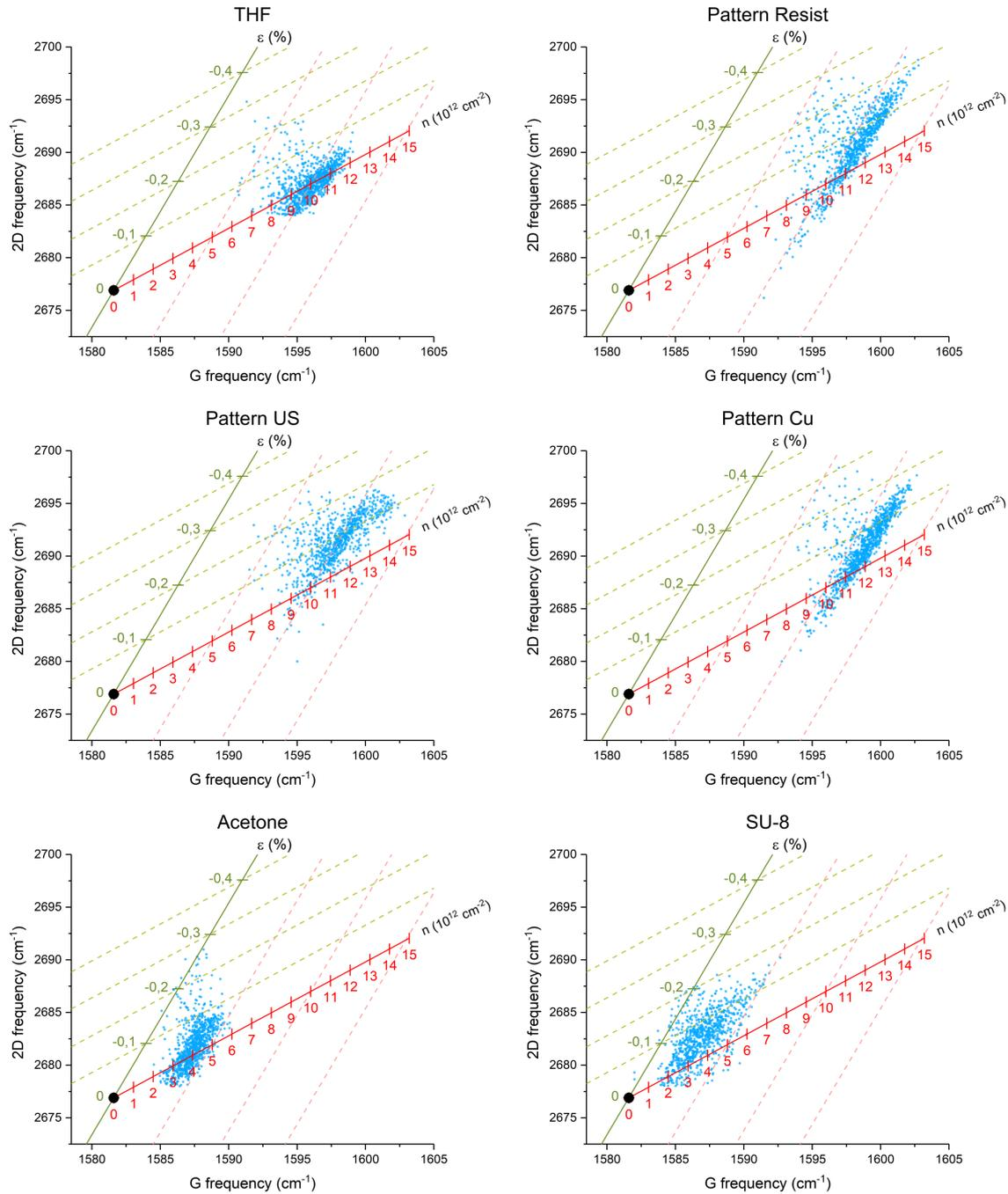
Figure 3.17: Strain-doping plots for the different step of the fabrication process, based on the method developed by Lee *et al.* The experimental ( $w_{2D}$ ,  $w_G$ ) data are plotted as blue points, the strain main axis in green and the hole-doping axis in red. The dark point indicates the origin corresponding to suspended graphene.
