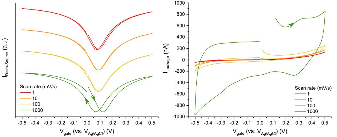
Figure 4.6: Scan rate effect on (left) the transistor current and (right) leakage current.  $V_{\text{DS}}$  was set to 0.1 V, the gate potential was swept between  $-0.5$  and  $0.5$  V in  $0.1 \text{ mol.L}^{-1}$  NaCl electrolyte.
