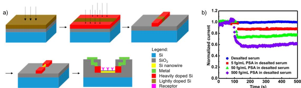
Figure 1.10: a) Top-down fabrication process of SiNWs-based FET label-free biosensor (adapted from [113]), b) Real-time detection of prostate cancer biomarkers with a SiNW-FET biosensor (from [110]).
