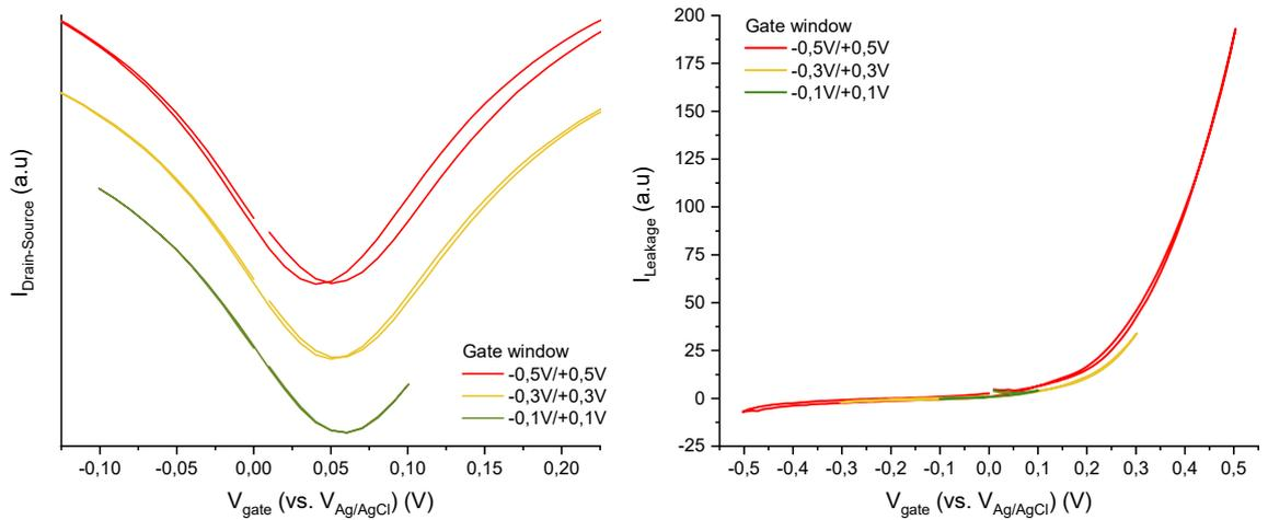
Figure 4.10: Transfer curves (left) and leakage current (right) for different gate potential windows, with  $V_{\text{DS}}$  set to 0.1 V a scan rate of  $10 \text{ mV}\cdot\text{s}^{-1}$  in  $0.1 \text{ mol}\cdot\text{L}^{-1}$  NaCl electrolyte. The curves for  $-0.2/+0.2$  V and  $-0.4/+0.4$  V gate windows are not shown for clarity.
