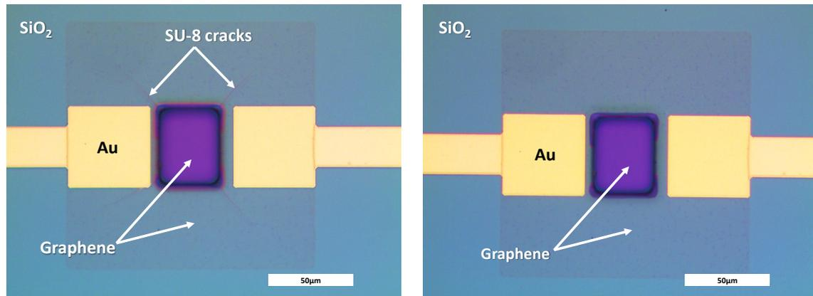
Figure 2.26: SU-8 passivation of the devices and the hard-bake effect on cracks induced by mechanical stress during the process, before (left) and after hard-bake (right). Scale bars are 50  $\mu\text{m}$ .
