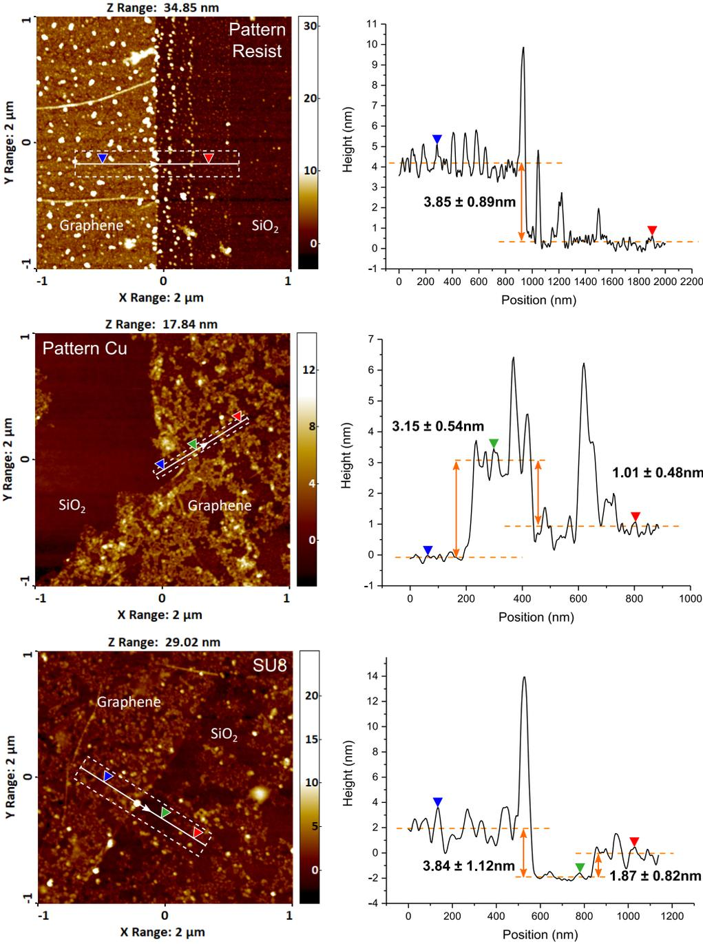
Figure 3.4: 2 μm × 2 μm scan (left) at the graphene/SiO<sub>2</sub> interface and the associated step height (right) after graphene patterning and passivation. Colormaps are harmonized (white spots are higher than 10nm).
