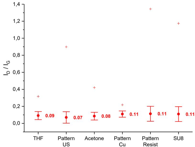
Figure 3.15: Mean values of the  $I_D/I_G$  ratio of the six samples, with standard deviation, min (minus sign) and max values (plus sign).
