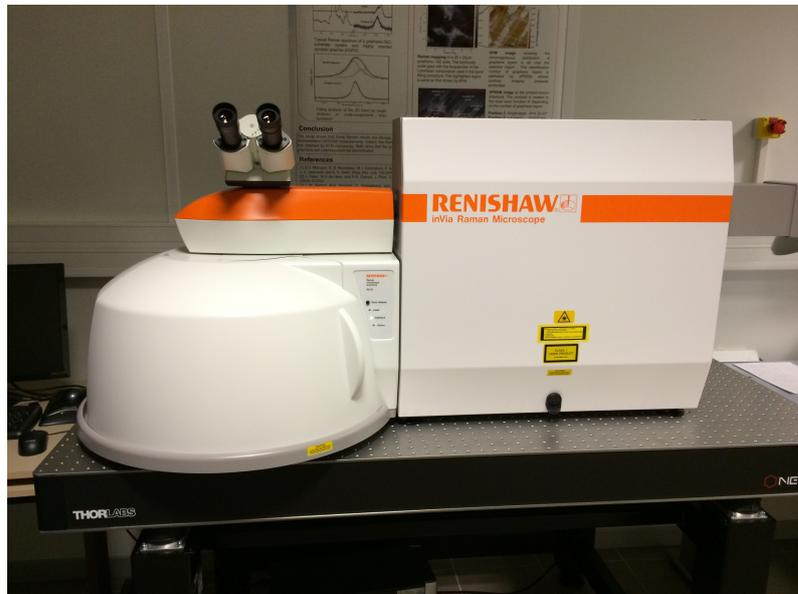
Figure 14: Raman inVia (Renishaw) spectrometer.
