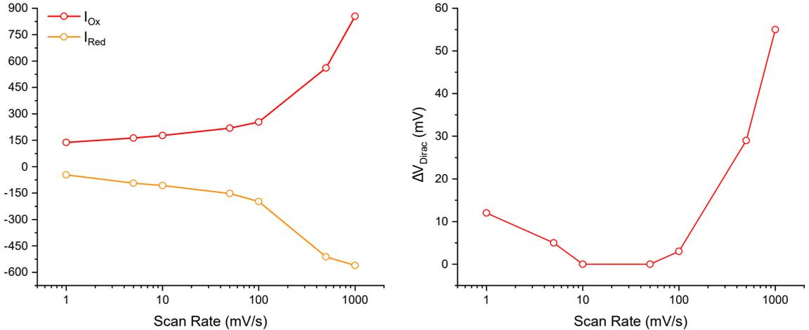
Figure 4.8: Evolution of (left) the hysteresis at  $V_{Dirac}$  and (right) of the maximal ( $I_{Ox}$ ) and minimal ( $I_{Red}$ ) transistor leakage current.  $V_{DS}$  was set to  $0.1 \text{ V}$ , the gate potential was swept 5 times between  $-0.5$  and  $0.5 \text{ V}$  in  $0.1 \text{ mol.L}^{-1}$  NaCl electrolyte.
