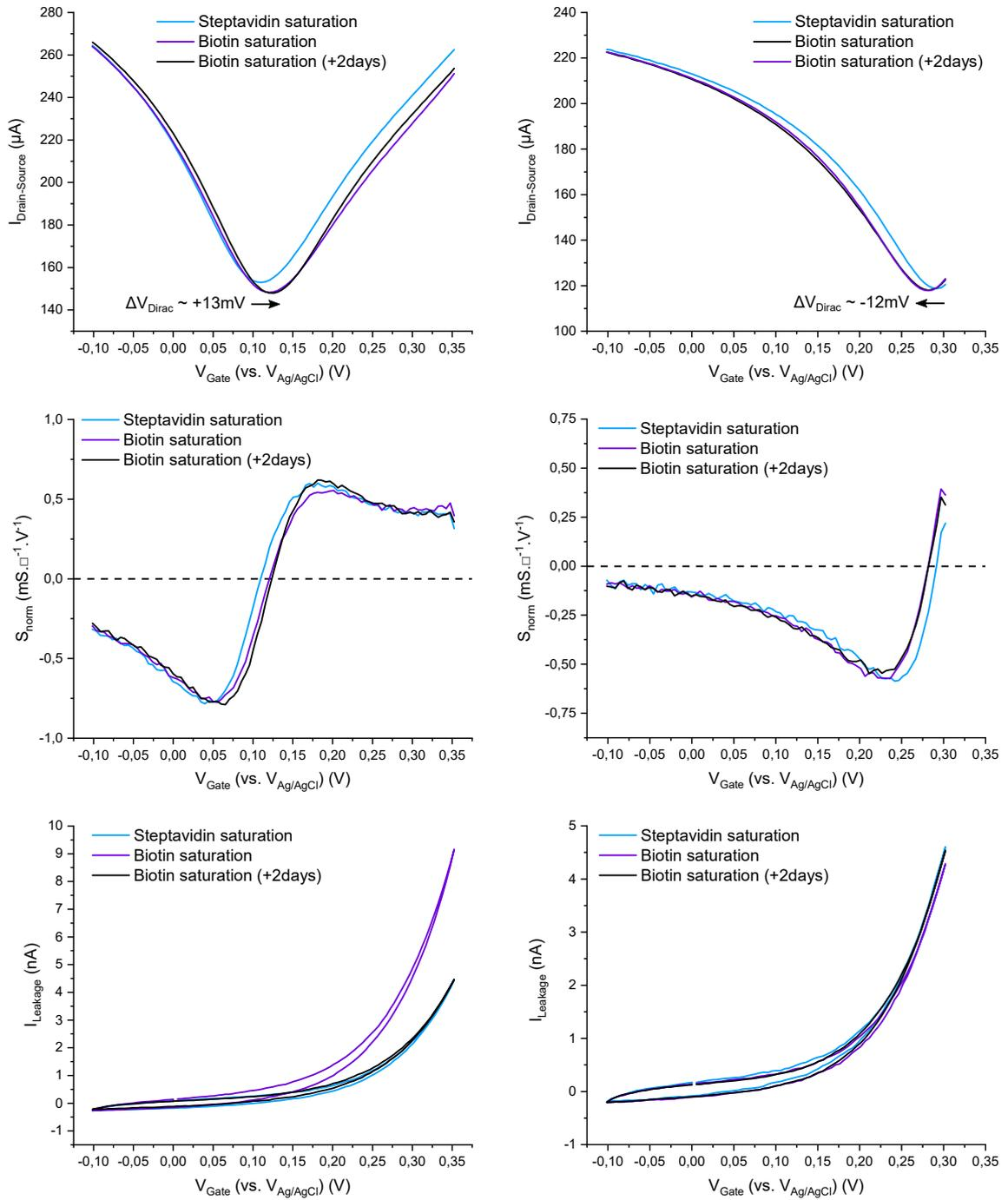
Figure 5.9: Transfer curves, normalized electrical sensitivity and leakage current curves after the sensor saturation with streptavidin (blue), after saturation with biotin (purple) and 2 days after (black) of tripod (left) and PBASE (right) functionalized SGFET.
