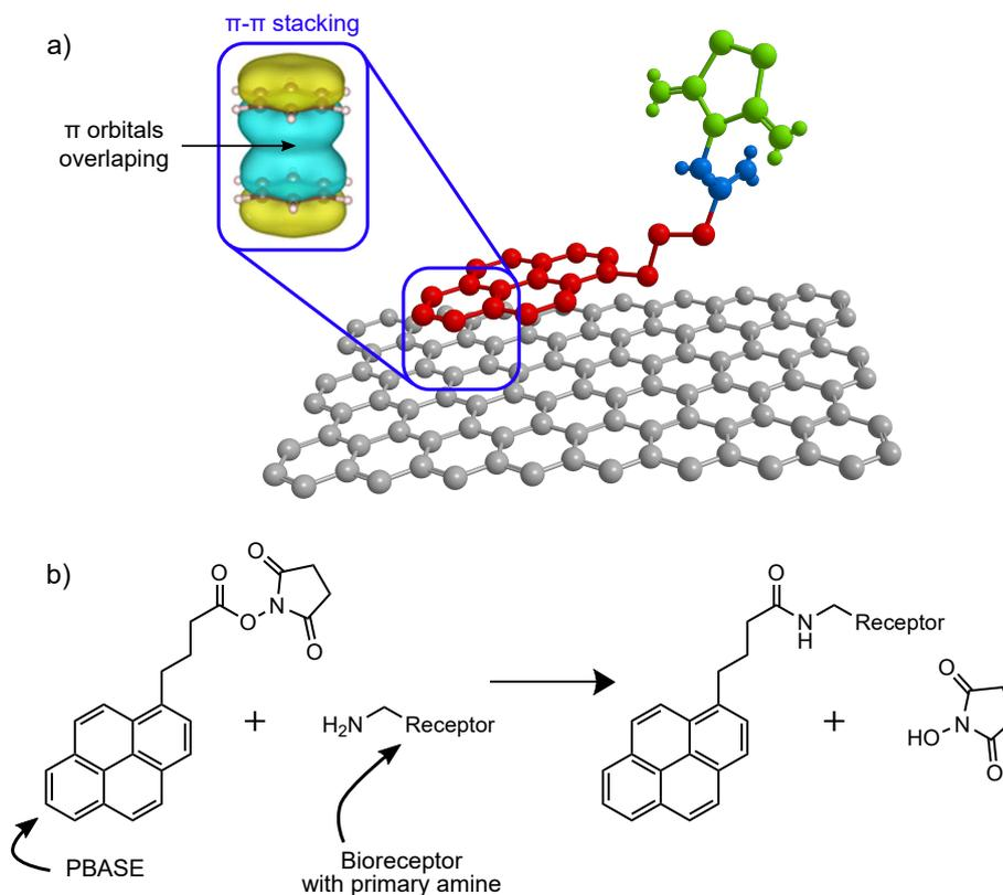
Figure 1.28: a) PBASE interacting with graphene by  $\pi$ - $\pi$  interactions (orbitals from [205]), b) Chemical reaction of bioreceptor grafting to PBASE by nucleophilic attack of the primary amine on the NHS leaving group.
