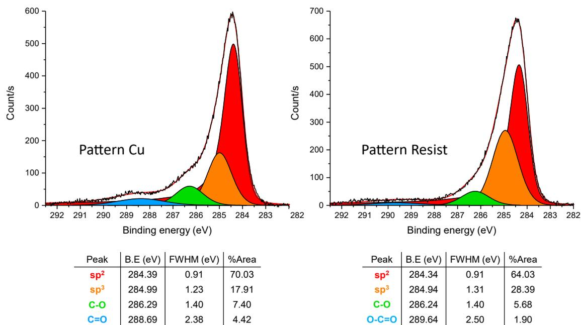
Figure 3.10: High-resolution C1s spectra of the pattern Cu and pattern resist samples with contributions of the different chemical bonds.
