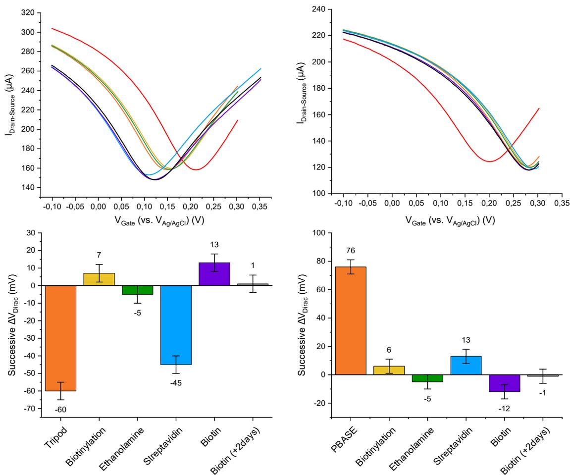
Figure 5.10: Transfer curves (top) and successive  $V_{\text{Dirac}}$  shifts (bottom) through the whole biosensing experiment of tripod (left) and PBASE (right) functionalized SGFET.
