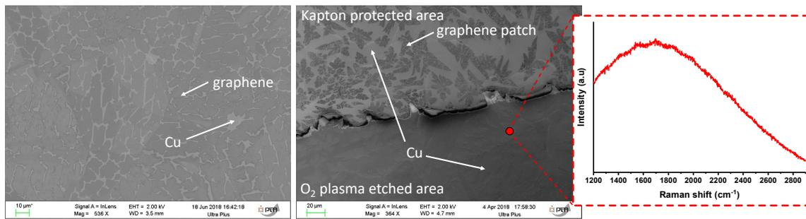
Figure 2.7: SEM observation of the non-continuous graphene bottom layer: before etching (left), after O<sub>2</sub> plasma etching (right), at the junction between an area protected from the plasma by kapton tape and an unprotected area. The absence of any graphene-related Raman peaks between 1200 cm<sup>-1</sup> and 2900 cm<sup>-1</sup> in this area indicates the complete removal of graphene. The background observed is due to the fluorescence of Cu.
