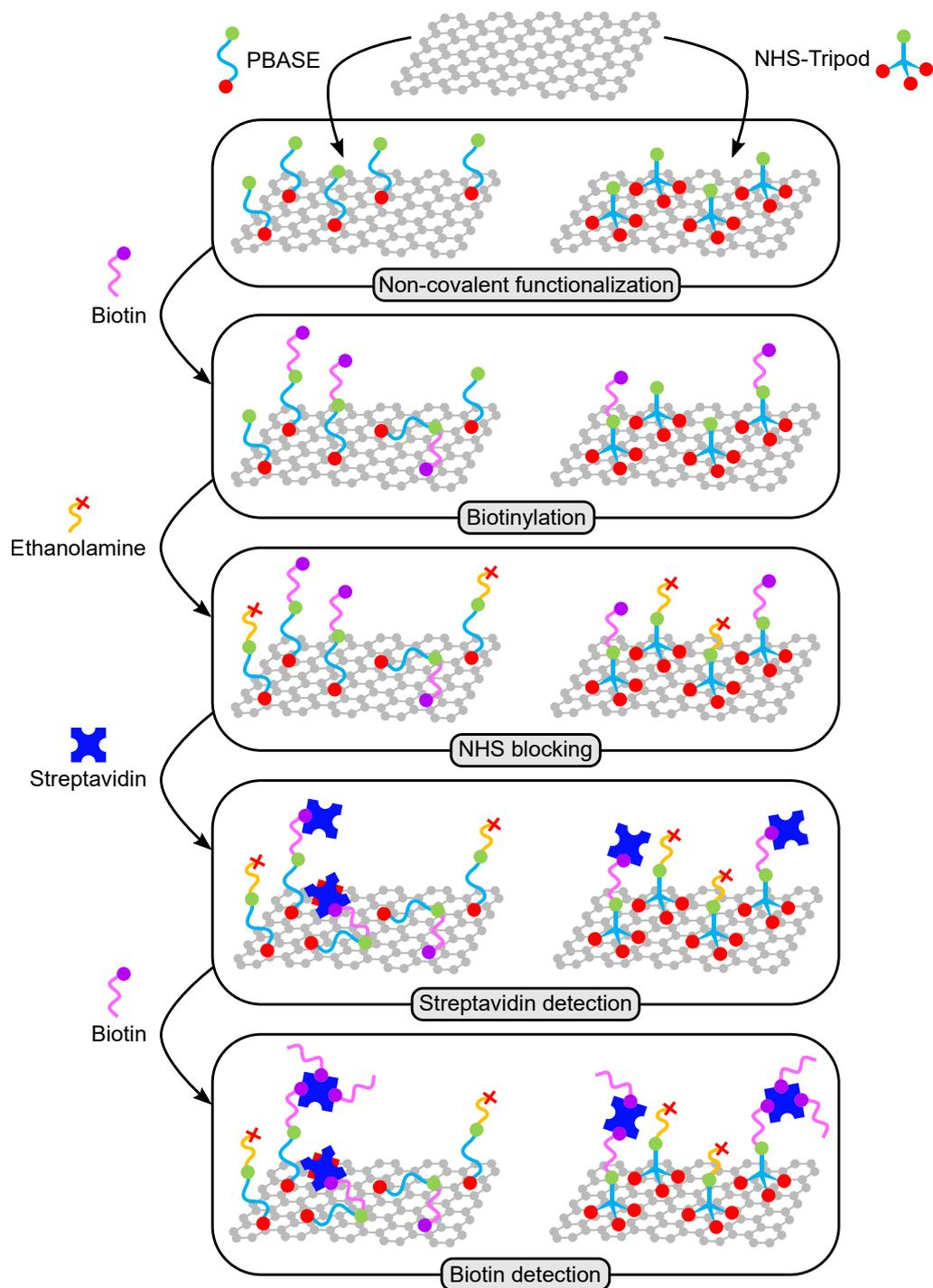
Figure 5.3: Schematic of the main steps of the procedure followed for both biosensing experiments carried out with either the tripod or PBASE.
