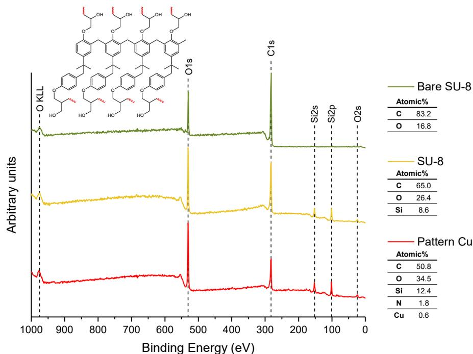
Figure 3.11: Survey spectra after SU-8 passivation (yellow) and on the surface of bare SU-8 on SiO<sub>2</sub> (green) and the relative atomic compositions. The survey spectrum of **Pattern Cu**, corresponding to the previous fabrication step was added for comparison. The monomer constituting the cross-linked SU-8 polymer is also shown (the red bonds are cross-linked to other polymer chains).
