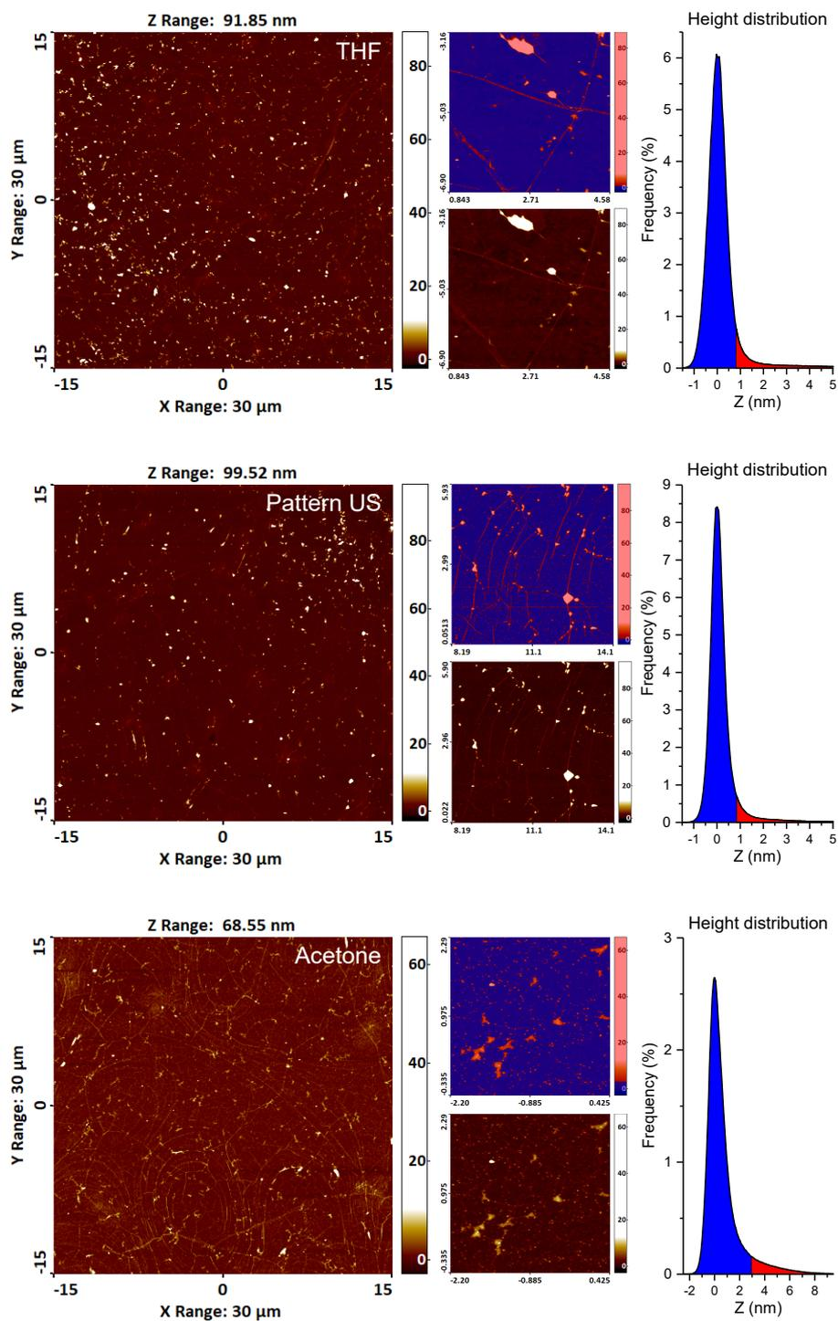
Figure 3.3:  $30\ \mu\text{m} \times 30\ \mu\text{m}$  2D maps of the graphene surface (left), raw zoomed view (middle-bottom) and coloured (middle-top) with the associated height distribution (right) of THF and acetone cleaning and graphene lift-off.
