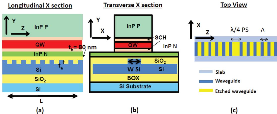
Figure 2.17: III-V on silicon DFB structure. (a) Longitudinal cross section. Grating is made on top of the silicon waveguide. (b) Transverse cross section. DFB parameters depends on the rib width  $W_{Si}$ . (c) Top view featuring the slab (light blue), the waveguide (blue) and the etched region (yellow). A  $\lambda/4$  phase shift is inserted in the centre of the cavity [57].
