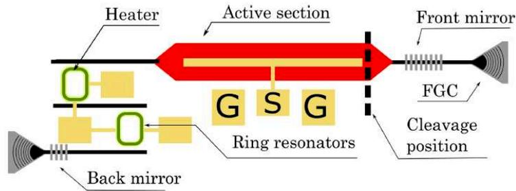
Figure 2.12: Schematic of a double RR laser design [57].
