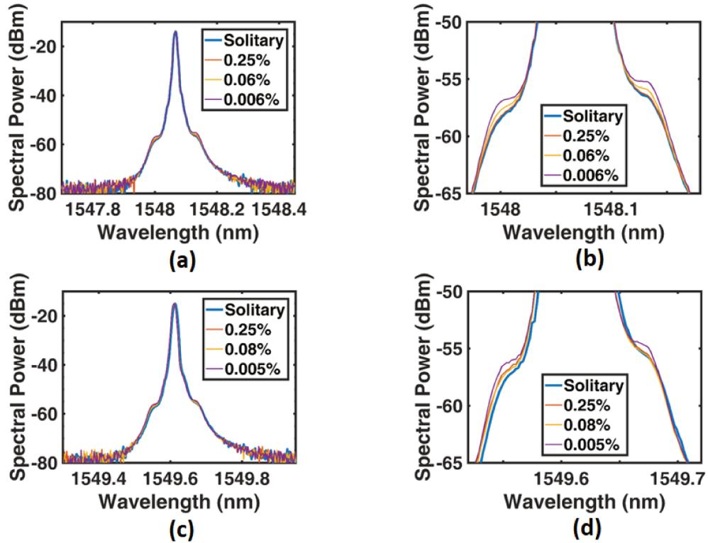
Figure 4.26: Optical Spectra of the hybrid III-V/Si DFB device at 20°C and 35°C under different feedback strengths: (a). Full spectrum, at  $T = 20^\circ\text{C}$ ; (b) Zoomed-in spectrum at  $T = 20^\circ\text{C}$ ; (c) Full shifted spectrum, at  $T = 35^\circ\text{C}$  and; (d) Zoomed-in shifted spectrum at  $T = 35^\circ\text{C}$ .
