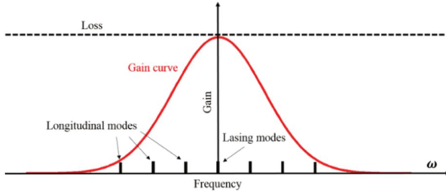
Figure 2.3: Schematic illustration of the gain curve and longitudinal modes of a semiconductor laser: cavity modes are given by  $m\frac{\lambda}{2} = nL$ , where  $m$  is an integer and  $n$  the effective refractive index [22].
