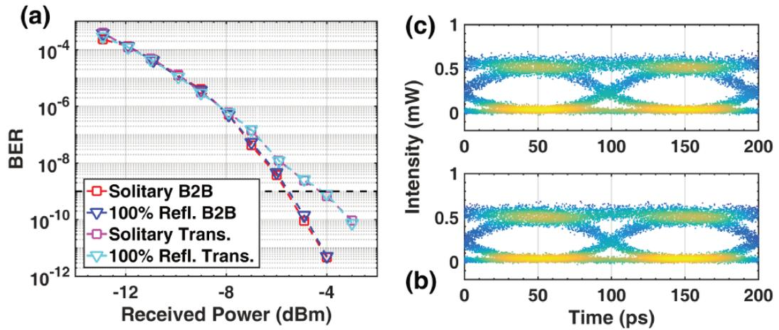
Figure 5.9: (a) BER characteristics of the high- $Q$  laser with (blue and cyan triangles) and without (red and magenta squares) feedback; eye diagrams (b) in B2B without feedback and (c) with maximal feedback after transmission.
