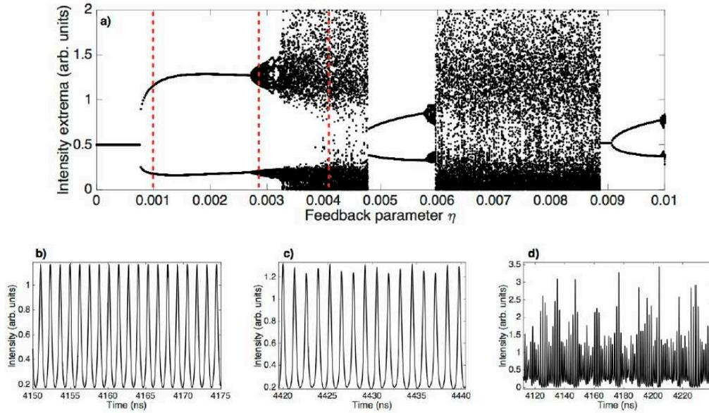
Figure 3.6: a) Numerical bifurcation diagram for  $T = 1700$ ,  $P = 0.5$ ,  $\theta = 500$  ( $L_{ext} \approx 30$  cm) and  $\alpha_H = 3$ . b) Corresponding time trace for  $\eta = 0.001$ . c) Time trace for  $\eta = 0.0027$ . d) Time trace for  $\eta = 0.0042$  [33].
