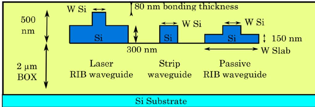
Figure 1.6: Silicon waveguides developed by III-V lab-Leti technology [74].
