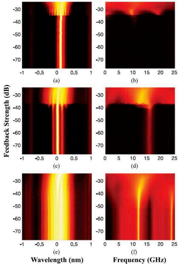
Figure 4.22: Evolution of the optical (left) and RF (right) spectra with the long feedback strength for three positions of the cleaved fiber. a) and b) correspond to a feedback phase of  $1.9\pi$  (minimum ROF, stable). c) and d) correspond to a feedback phase of  $0.3\pi$  (maximum ROF, stable). e) and f) correspond to a feedback phase of  $0.25\pi$  (strongest oscillations).
