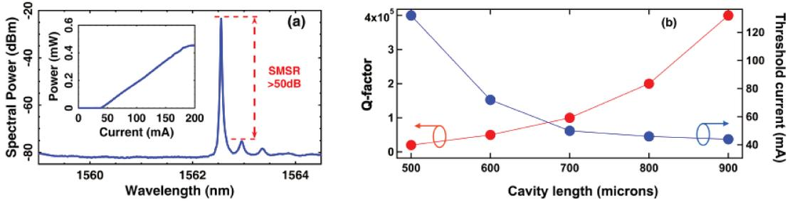
Figure 5.4: (a) Optical spectrum of the high- $Q$  DFB laser and L-I curve (inset) at  $3 \times I_{th}$ ; (b) The calculated  $Q$  factor and threshold current as a function of the total cavity length.
