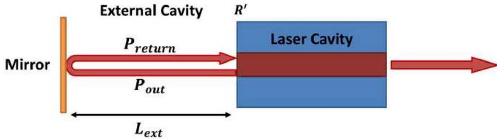
Figure 3.1: Semiconductor laser subject to optical feedback [4].
