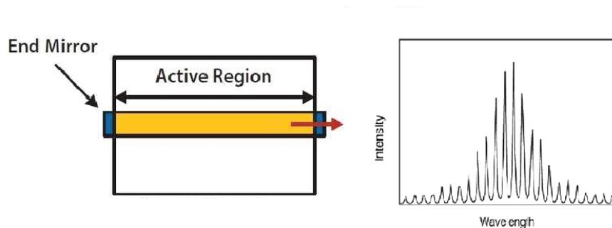
Figure 2.5: Fabry-Perot: Device schematic and laser spectrum [39].
