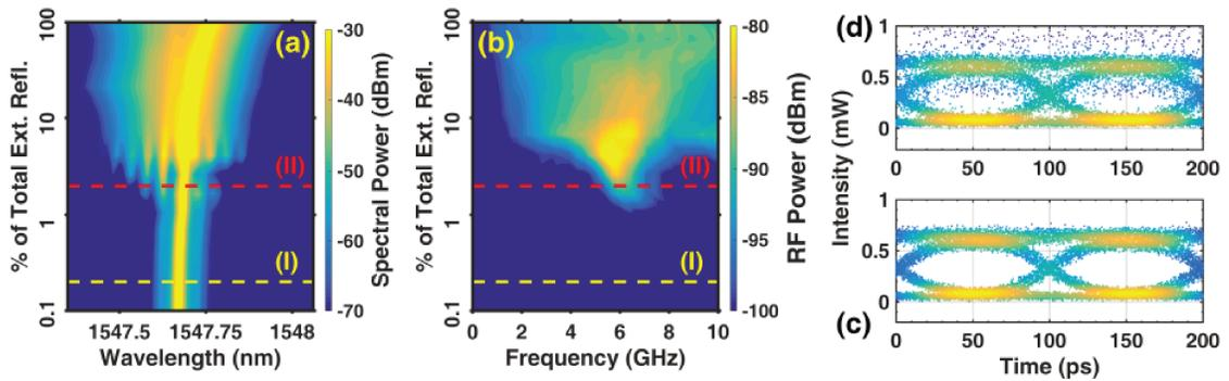
Figure 5.8: (a) Optical and (b) RF spectral map of a conventional QW DFB laser; eye diagrams at (c) level (I) and (d) level (II) marked in the map.
