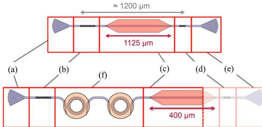
Figure 4.1: Schematic view of the FP (top) and TUL (bottom) under study, with the Si waveguides shown in grey. The lettered sections correspond to (a) and (e) vertical couplers, (b) high-reflectivity DBR, (c) III-V gain section, (d) low-reflectivity DBR, and (f) Si rings. The dotted red line on the TUL design shows where the samples used in this study were cleaved.
