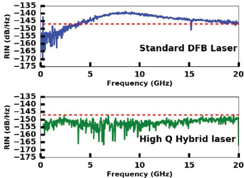
Figure 5.1: Relative intensity noise measurements at bias current of 120 mA with similar threshold values for: (a) A standard  $\lambda/4$  phase shifted hybrid DFB laser design (top) and a high- $Q$  hybrid laser (bottom) [11].
