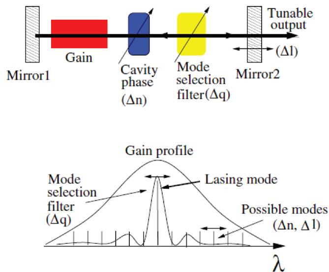
Figure 2.8: Tunable single laser and gain profile [53].
