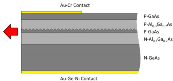
Figure 2.7: First fabricated DFB structure [41, 42].
