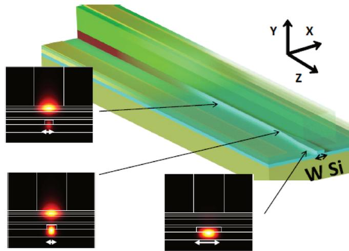
Figure 2.15: 3D view of a III-V on Si waveguide. The with  $W_{Si}$  of the Si waveguide controls the confinement in the III-V region. [59].
