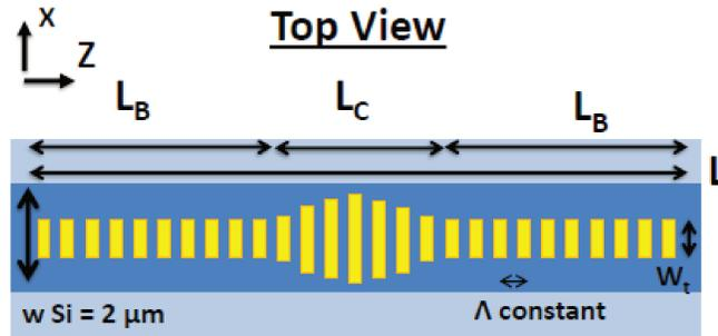
Figure 5.3: Top view of of the high- $Q$ . The 300 nm slab is in light blue, the 500 nm waveguide in darker blue and the 30 nm tooth etched regions in yellow. The grating has two regions: a parabolic tapered grating in the centre and a uniform grating at each side
