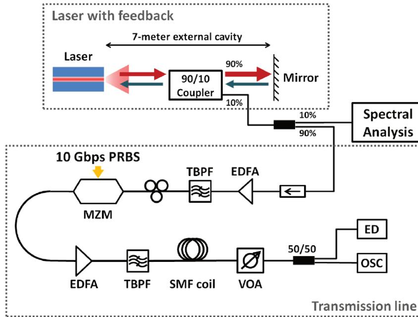
Figure 5.6: Experimental set-up used for optical feedback investigation.
