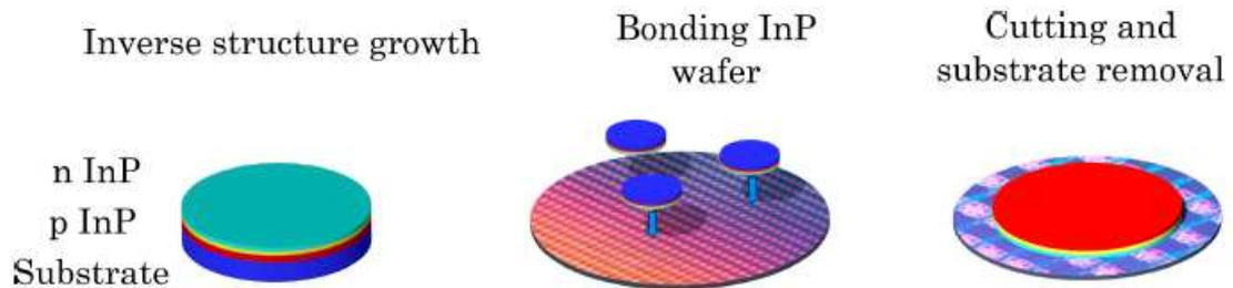
Figure 1.7: III-V on silicon epitaxy and bonding [74].
