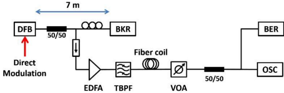
Figure 4.25: Experimental set-up used for optical feedback investigation.
