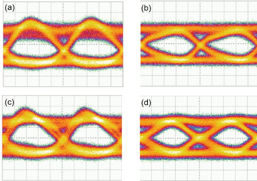
Figure 4.29: Eye diagrams in (a) back-to-back (solitary) for  $T = 20^{\circ}\text{C}$ , (b) after 10 km transmission (solitary)  $T = 20^{\circ}\text{C}$ , (c) back-to-back (solitary) for  $T = 35^{\circ}\text{C}$ , (d) after 10 km transmission (solitary)  $T = 35^{\circ}\text{C}$  .
