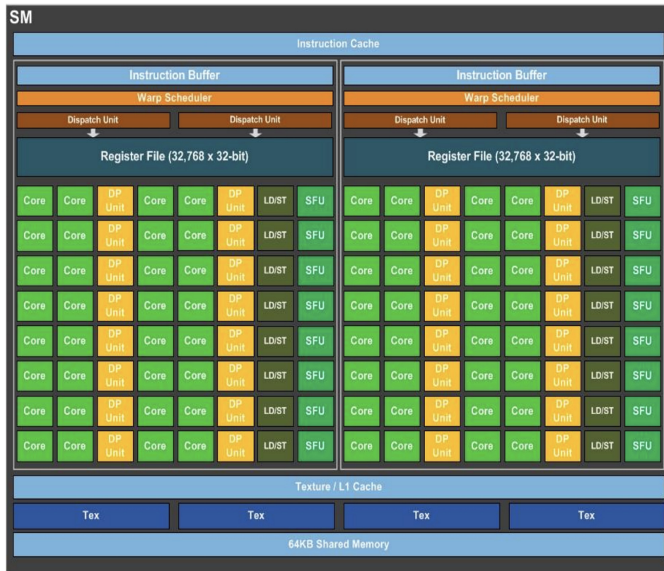
Figure 2.16: Nvidia Pascal GP100 Streaming Multiprocessor Unit [87].
