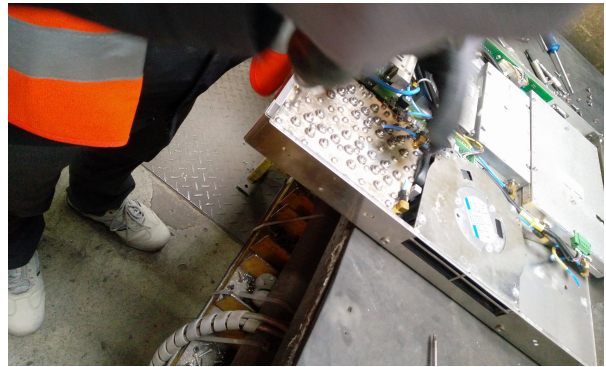
(b) Human operator cutting the wires manually for recycling the electronic device.
