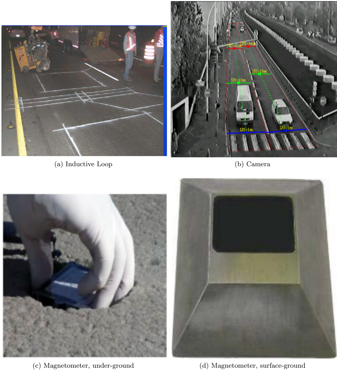
Figure 2.1: Some examples of vehicle detector technologies [12]
