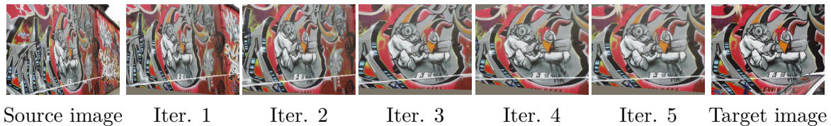
Figure 3-12: Qualitative results on the Graffiti benchmark, pair (1, 5). The first and last columns show the source and target images. The intermediate columns show the progress of the alignment at different iterations.
