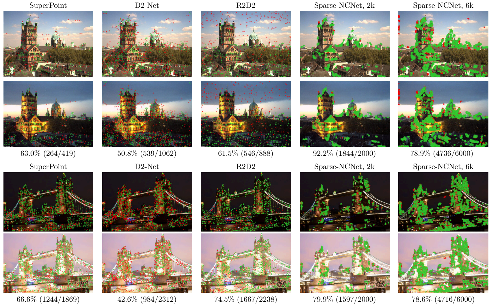
Figure 6-7: HPatches qualitative results (illumination) . We present the results of Sparse-NCNet, along with state-of-the-art methods SuperPoint [DeTone et al., 2018], D2-Net [Dusmanu et al., 2019] and R2D2 [Revaud et al., 2019]. The correct correspondences are shown in green, and the incorrect ones in red for a threshold t = 3\text{px} . Below each pair we indicate the fraction of correct matches (both in percentage and absolute values). Our method is presented for both the top 2K and top 6K matches, and it obtains the largest fraction of correct matches for both cases. Examples are from the illumination sequences.
