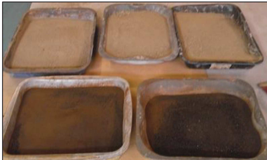
Figure 3.1 The clay (lighter colour) and alum sludge after grinding and sieving
