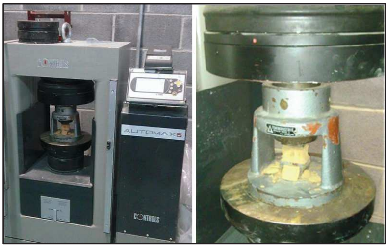
Figure 3.4 The compression strength testing
