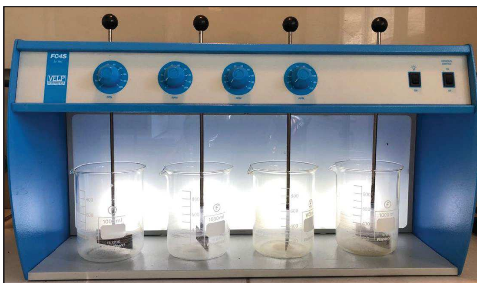
Figure 2.15 Jar-test apparatus of co-conditioning trials
