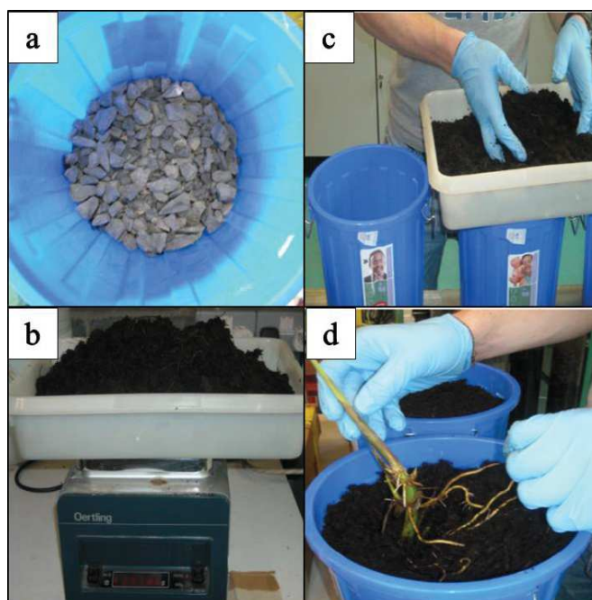
Figure 4.3 Pot setup (a) filled with gravel; (b) measuring the media mass; (c) filled with peat; (d) planting reeds
