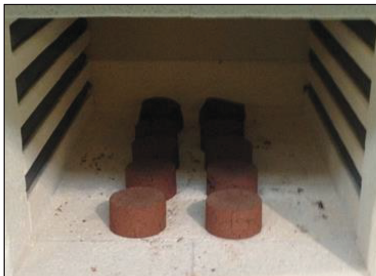
Figure 3.3 The bricks from Batch 3 in the kiln after firing
