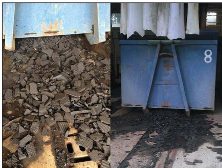
Figure 2.1 Alum sludge being collected for disposal in Dublin Ballymore Eustace WTP
