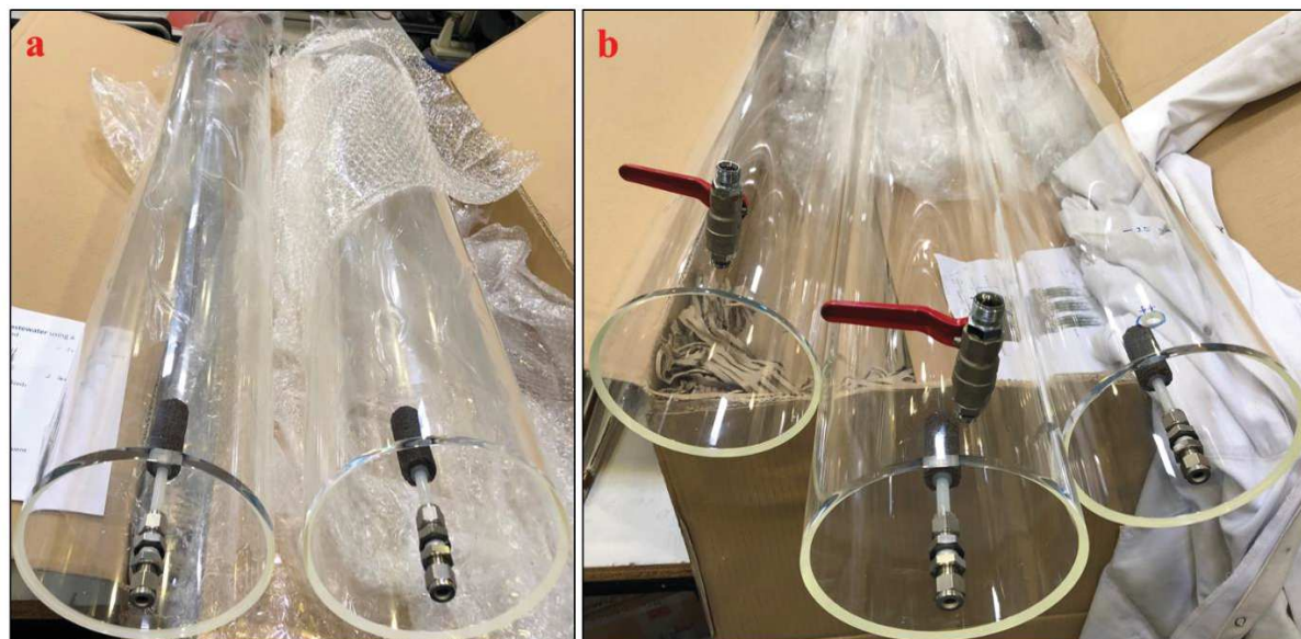
Figure 7.1 The columns setup; (a) the aeration diffuser of the column, (b) the outlet valves of the columns
