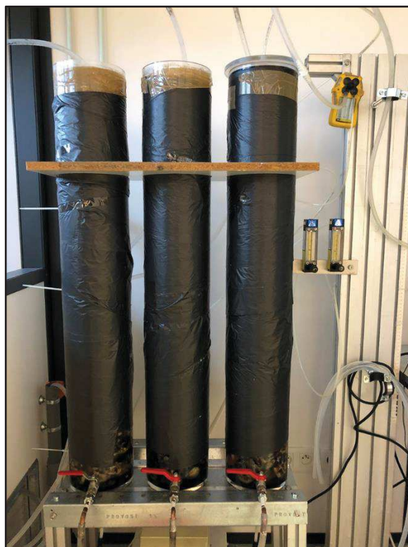
Figure 2.18 The three parallel aerated alum sludge constructed wetland
