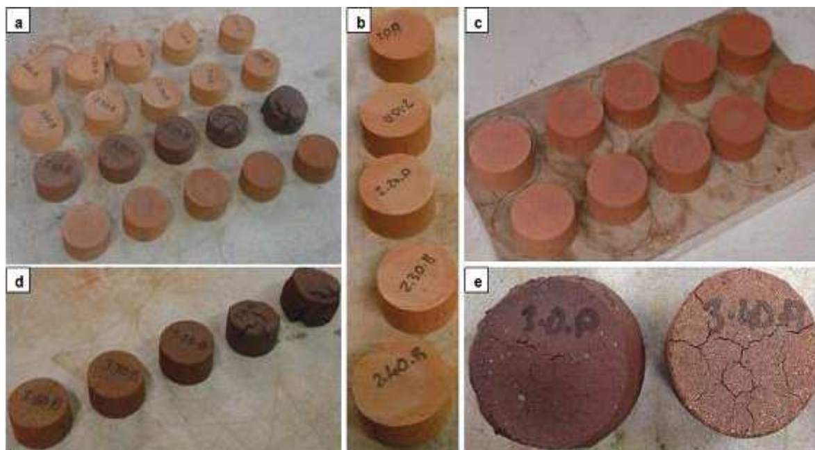
Figure 3.7 General appearance: (a) Batch 1–4 from top to bottom in the picture; (b) Batch 2; (c) Batch 4; (d) Batch 3; (e) The 0 % sludge brick (left), and the 40 % sludge brick (right) fired at 1200 °C
