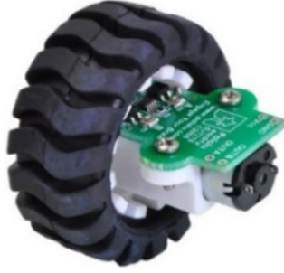
FIGURE 1.3: Wheel odometry encoder ( Pololu Corporation 2016 )
