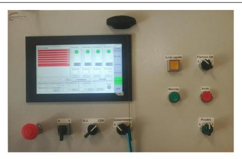
Figure 2.1 Interface of the HVOF spray control system
